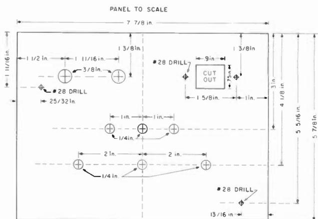
Fig. 4. Front panel layout.
