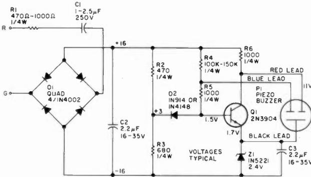
**DING-A-LING:** This electronic bell needs no power supply. The layout and most of the resistors are not critical, although C2, R2, and R3 work best at the values given. Leaving out R1 will make the unit ring louder. The piezo buzzer may vary from store to store, so if it has two leads, connect the red lead to the collector and the black lead to the emitter of Q1. If a third (blue) lead is present, connect it to the base of Q1.—E. C. Sherrill W5TPP, Fort Worth TX.
