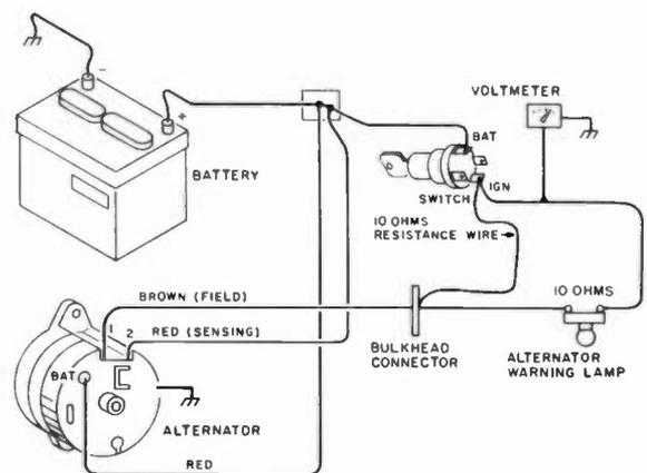
Fig. 2. Typical automobile charging circuit.
