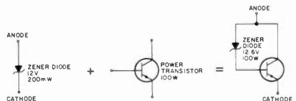
Fig. 5. The amplified zener diode.
