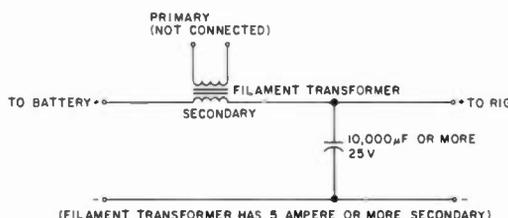
Fig. 3. Alternator-whine filter using filament transformer for inductor.
