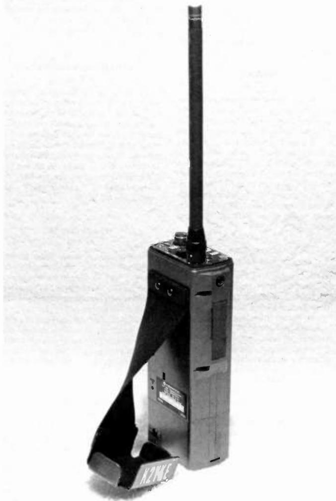
Photo C. Detail of attachment of band to top rear of unit using the belt-clip mounting nuts already in the unit.
