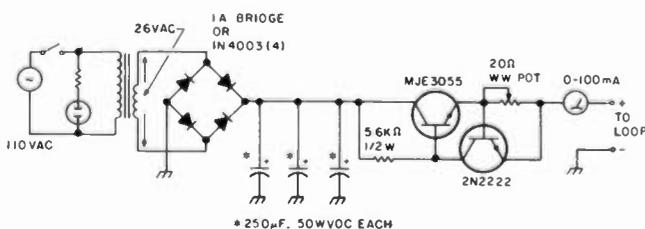
Fig. 1. Low-voltage loop supply.
