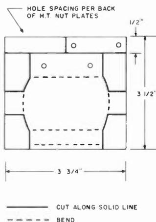
Fig. 1. Metal-cutting pattern.
