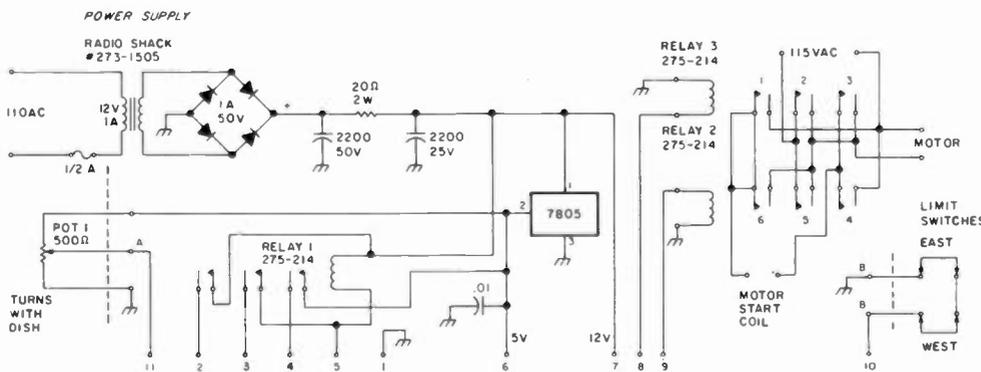
Fig. 12. Power supply schematic.
