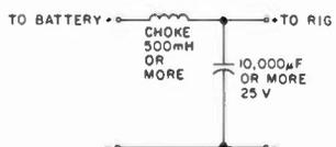
Fig. 2. Inductor-capacitor alternator-whine filter.
