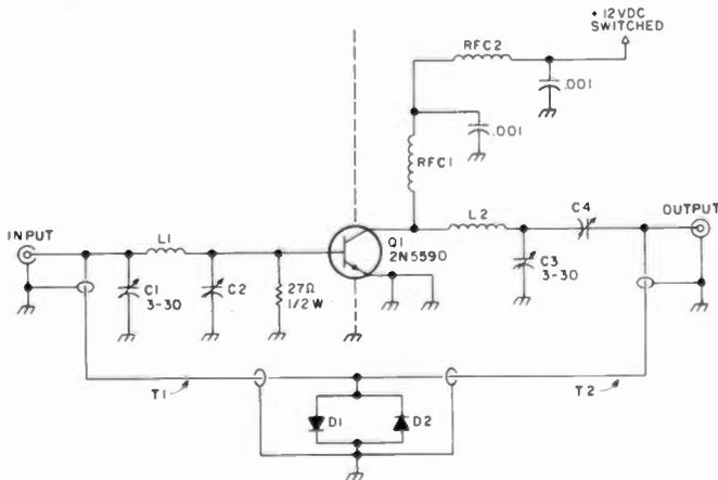
Fig. 1. Amplifier schematic. C2—68 pF mica in parallel with 7-45 pF trimmer; C4—7-45 pF trimmer; D1,D2—1N914; L1,L2—2-1/2 T, #22 solid wire, 1/4" dia., spaced 3/4"; RFC1, RFC2—approx. 6 T #22 PE, 1/4" dia., close-spaced; T1, T2—1/4λ, RG-174 (approx. 13-1/2').
