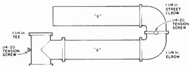
Fig. 1. Gimbal-mount construction detail.
