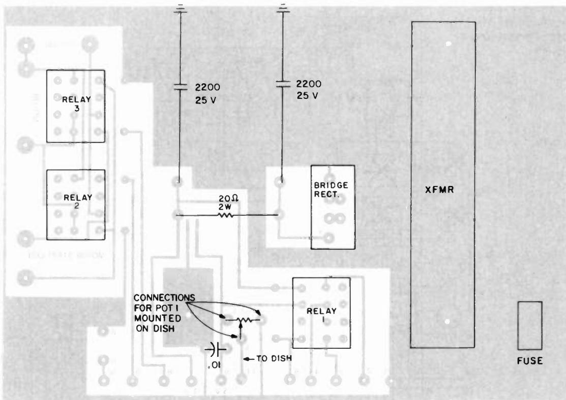
Fig. 11. Power supply PC board (component side).
