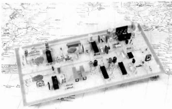
RTTY AFSK mod/demod terminal unit from GFS Electronic Imports.
