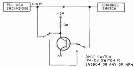
**USE THOSE MISSING CB CHANNELS:** Add more frequencies to your PLL CB-to-10 conversion by adding a switch and a transistor to invert the least significant bit going to the PLL chip. With the switch as shown, you can get 10 kHz above channels 3, 11, and 19, as well as 10 kHz below channels 8 and 16.—Bob Raker WB8ZFF, Cincinnati OH.
