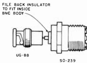
**BETWEEN-CONNECTOR SERIES ADAPTER:** A BNC female (UG-625) fits nicely in a UHF male (PL-259). Just solder a wire to the BNC center and insert it in the body of the PL-259. Solder the center conductor and the seam between the bodies. With just a little more difficulty, an SO-239 can be attached to a BNC male (UG-88). An "F"-type female will thread directly into a BNC male. SMA to BNC (both ways) can be done just as easily.—Bob Raker WB8ZFF, Cincinnati OH.
