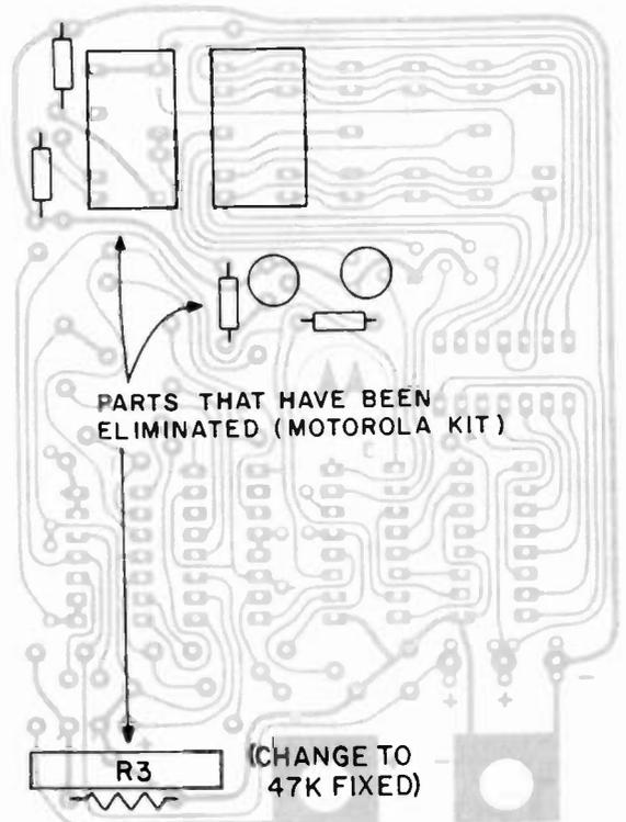
Fig. 2(b). Component side of the Motorola board showing which parts are not used.
