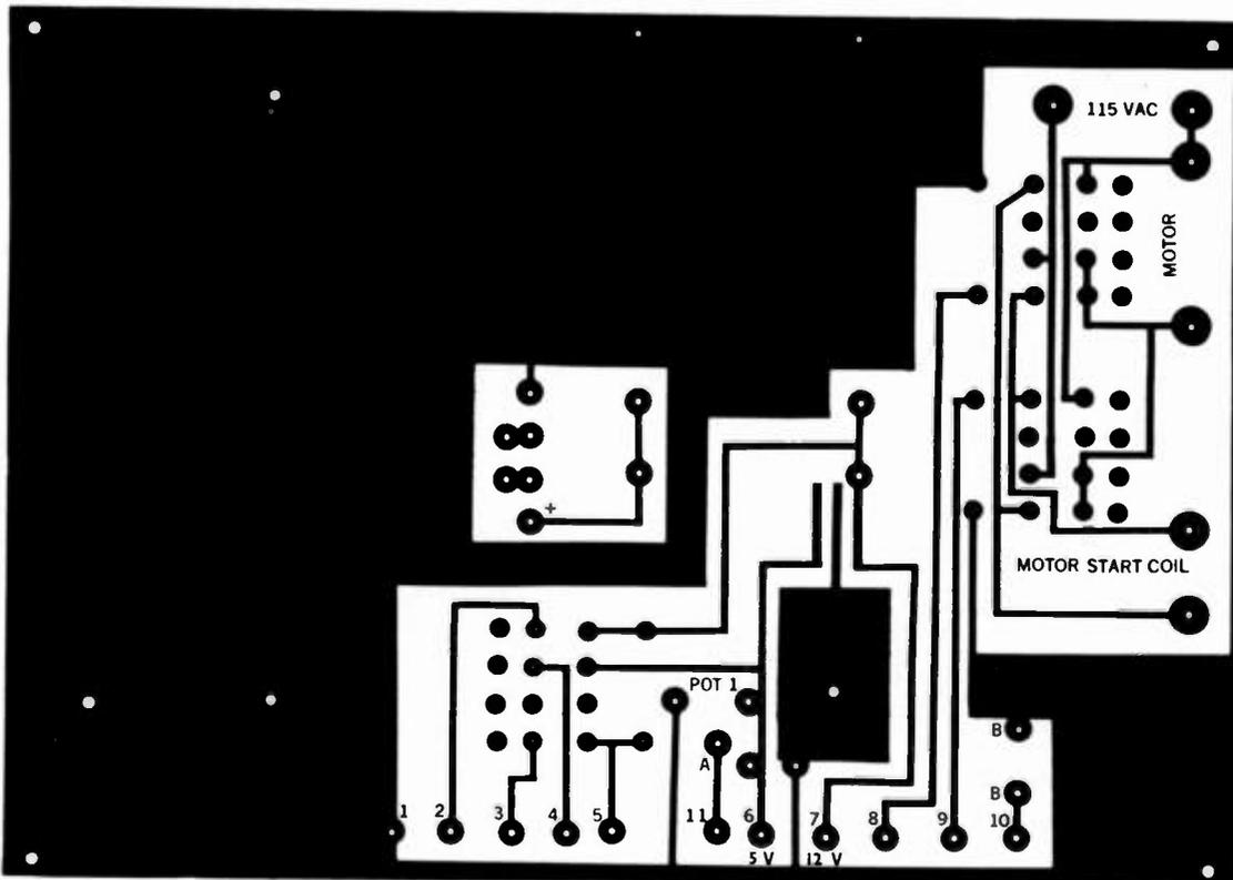
Fig. 10. Power supply PC board (foil side).
