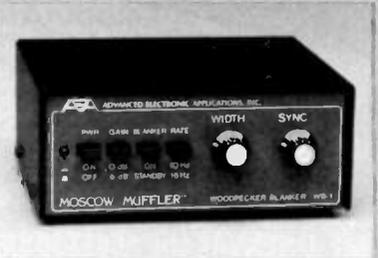
This extremely useful accessory is designed for direct insertion between your receiver (or transceiver) and the antenna. It is both MORE EFFECTIVE than I.F. type blankers and requires NO MODIFICATIONS to your receiver! The unit operates from a 13 VDC ± 2 VDC power source at less than 575 mA. (AEA AC wall unit AC-1 will operate the blanker.)
