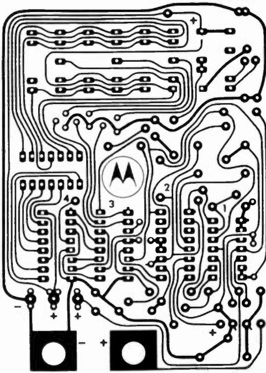
Fig. 1. Motorola PC board (foil side).
