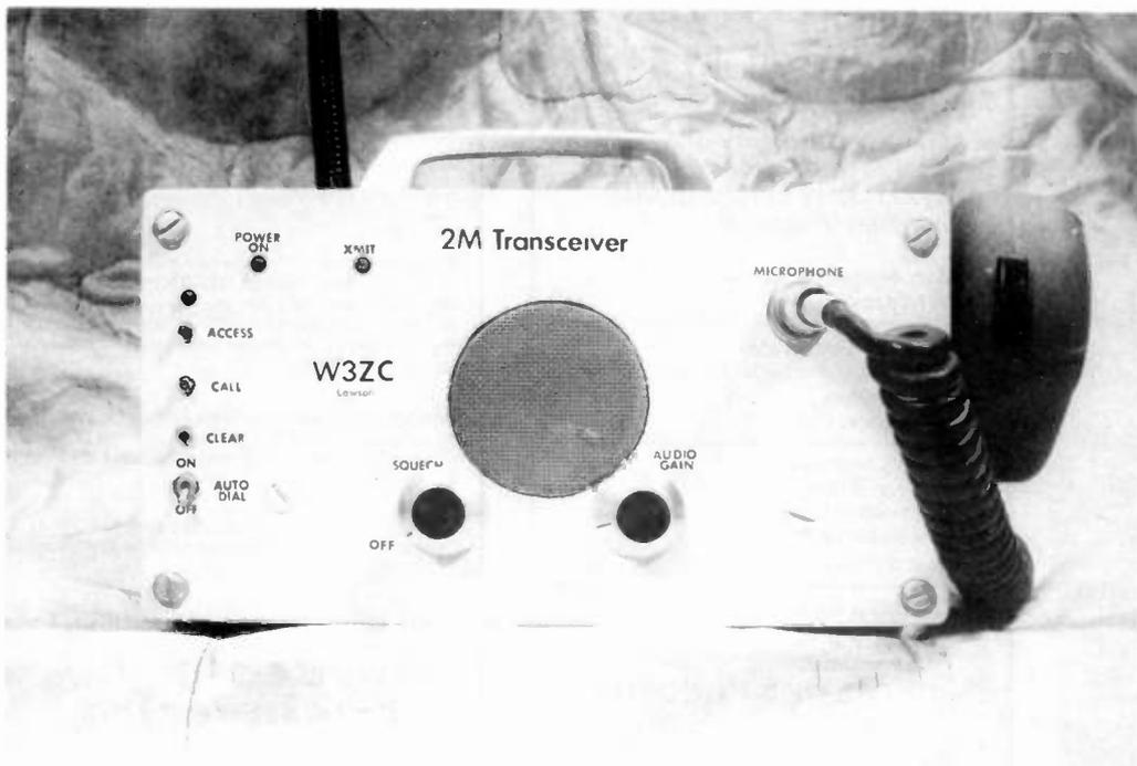
Photo A. Front-panel mounting of switches and LED.
