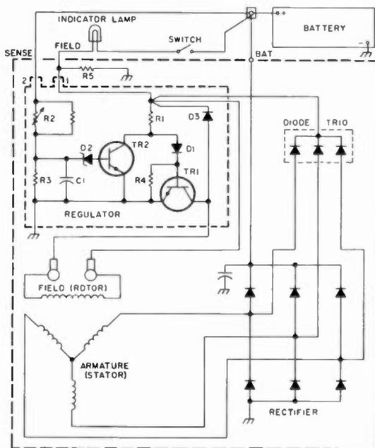
Fig. 1. Alternator schematic diagram.
