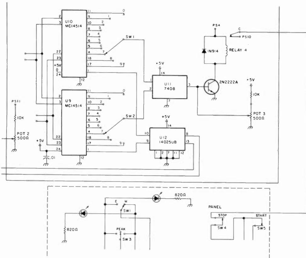
Fig. 9. Control panel schematic.
