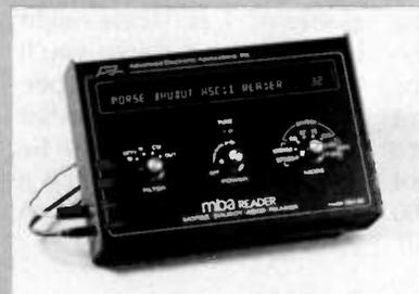
While no machine can yet match the ability of a skilled CW operator in copying poor fists or signals buried in the noise, the MBA-RO by AEA excels even when compared against units costing much more. The large 32 character display allows much easier reading than shorter displays, especially at higher speeds such as 60 WPM or 100 WPM RTTY. The MBA-RO also features dual filters for RTTY decoding of either 170 Hz or 425 Hz (easily changed to 850 Hz) shift transmissions.
