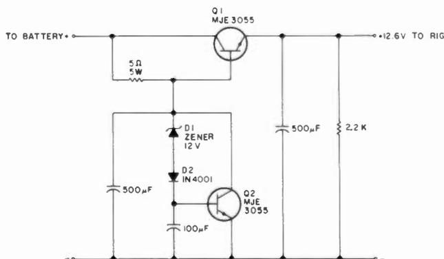
Fig. 4. Electronic regulator to remove alternator whine.
