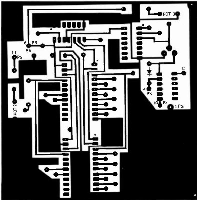
Fig. 7. Control PC board (foil side).
