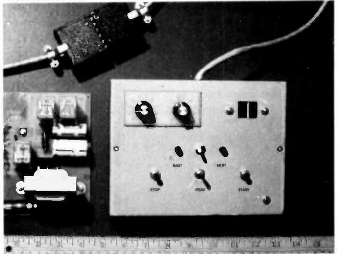
Photo D. Cabinet, power supply, and connector.
