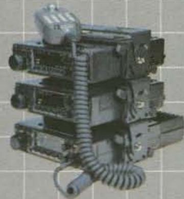
**Stacking Mobile Mounts.** The IC-27A/37A/47A can be stacked to provide a three band mobile station. Each band is full featured and will operate even when another band is in use.
