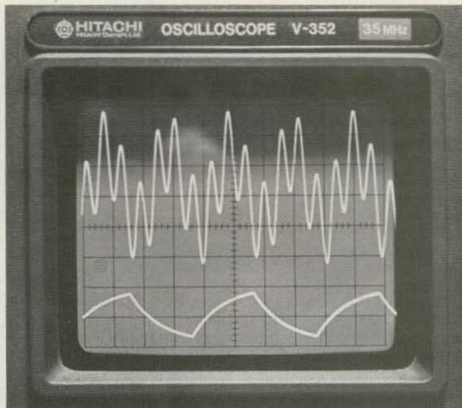
Photo E. Upper trace shows the composite audio output of the Two-Tone Plus generator. Tones are synchronized but are not harmonically related. Lower trace shows sync waveform. Both tones are harmonics of the sync frequency.
