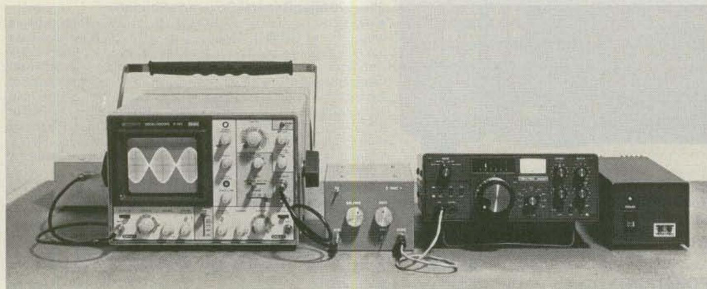
Photo B. Typical two-tone test setup. Refer to the text for high-power testing precautions.
