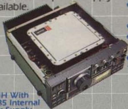
IC-471H With IC-PS35 Internal Power Supply Installed
