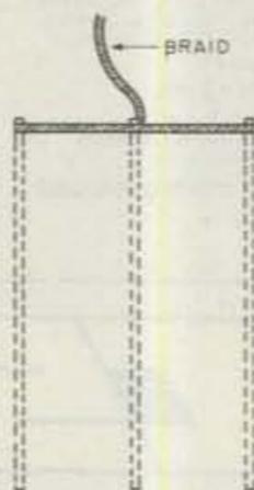
Fig. 2(b). Three ground rods connected in parallel.
