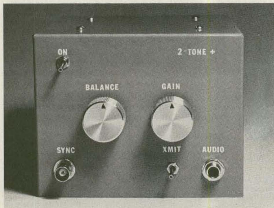
Photo A. Two-Tone Plus is an SSB-transceiver and linear-amplifier tuning aid which includes a sync output for stable rf-waveform viewing.
