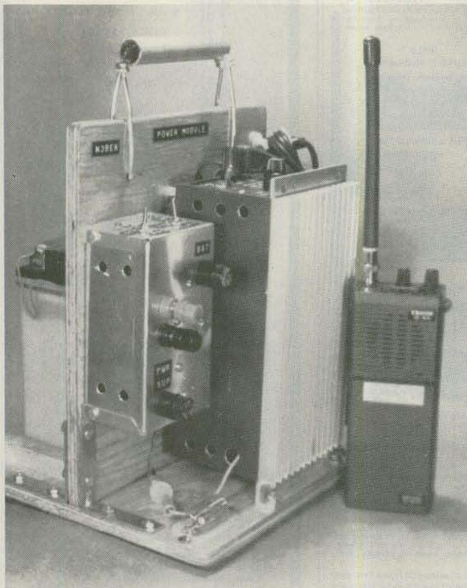
Photo A. Power supply and control box mounted on one side of plywood frame.
