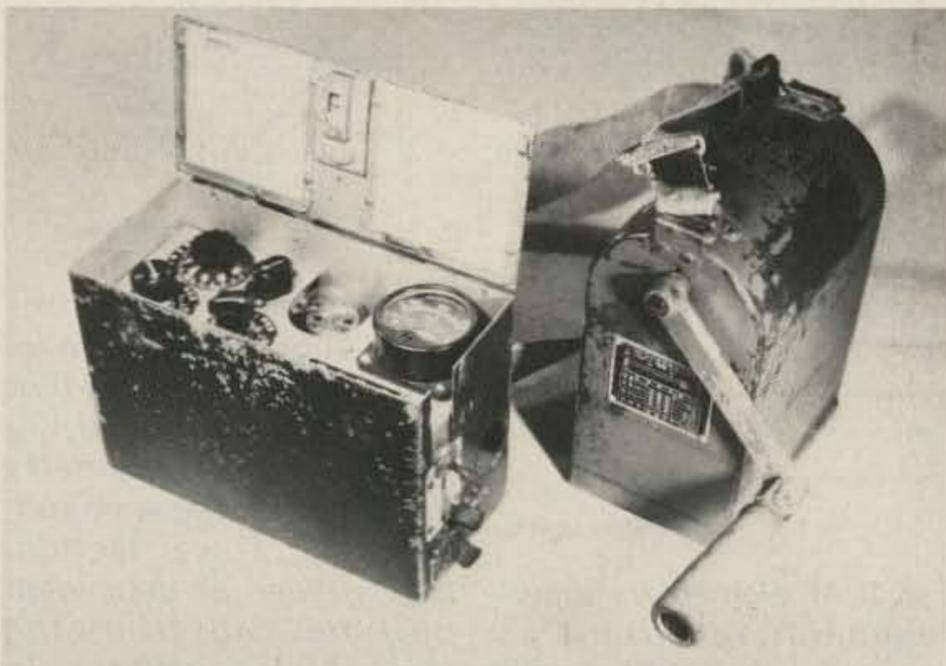
Photo A. Japanese WWII transceiver with hand-cranked generator used when transmitting.
