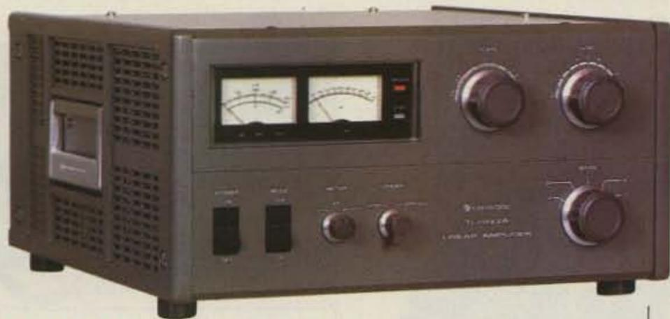
**TL-922A** 160-15 m 2 KW PEP/1 KW DC Input Linear Amplifier. Pair of EIMAC 3-500Z tubes and excellent IMD characteristics. Perfect safety protection with blower turn-off delay circuit.
