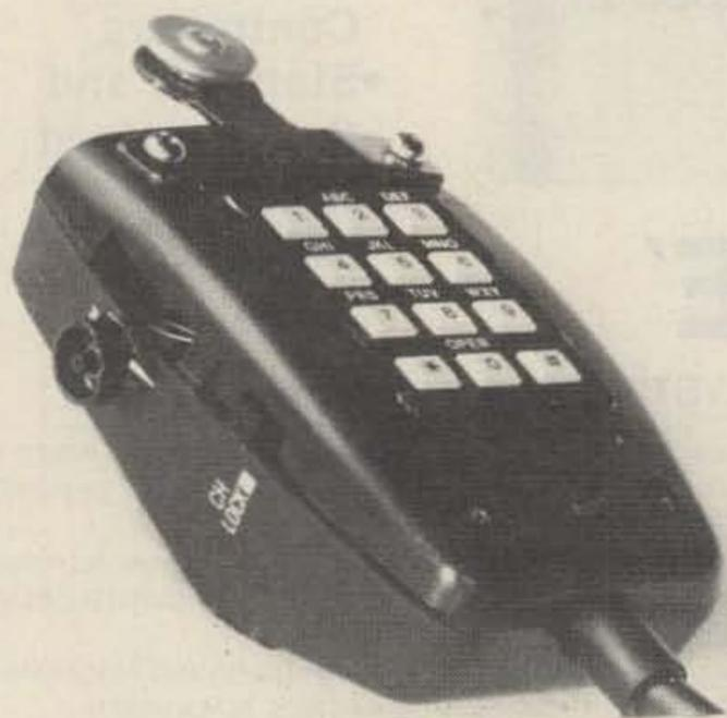
Photo A. The speed-dial switch mounts on the side of the microphone near the area where the remote volume control used to be. A protection ring around the dial button eliminates any accidental dialing sequences while handling the microphone.
