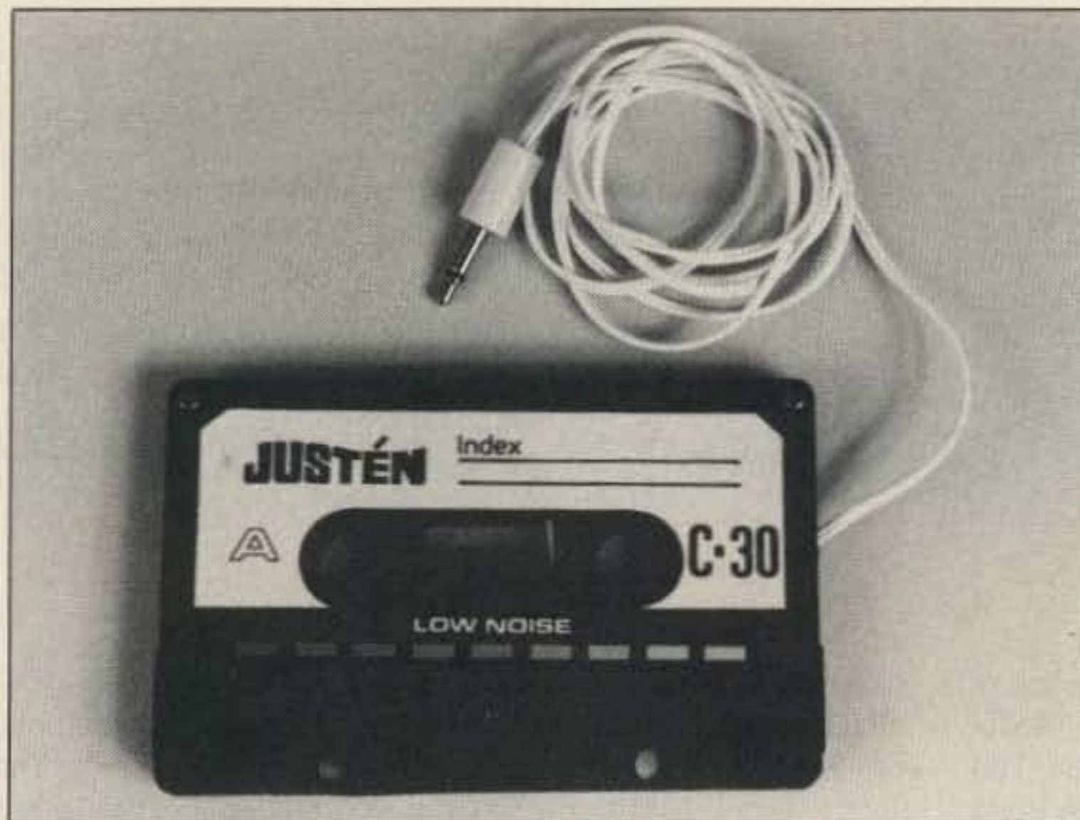
Photo A. The assembled unit to pipe your rig's AF to your car speaker system via the cassette tape pickups.
