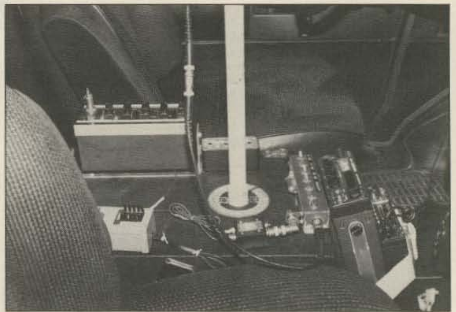
Photo D. The home-built console holds one or more transceivers of any size on its sloping front, along with the bearing indicator, attenuator, preamp, and HT battery charger.
