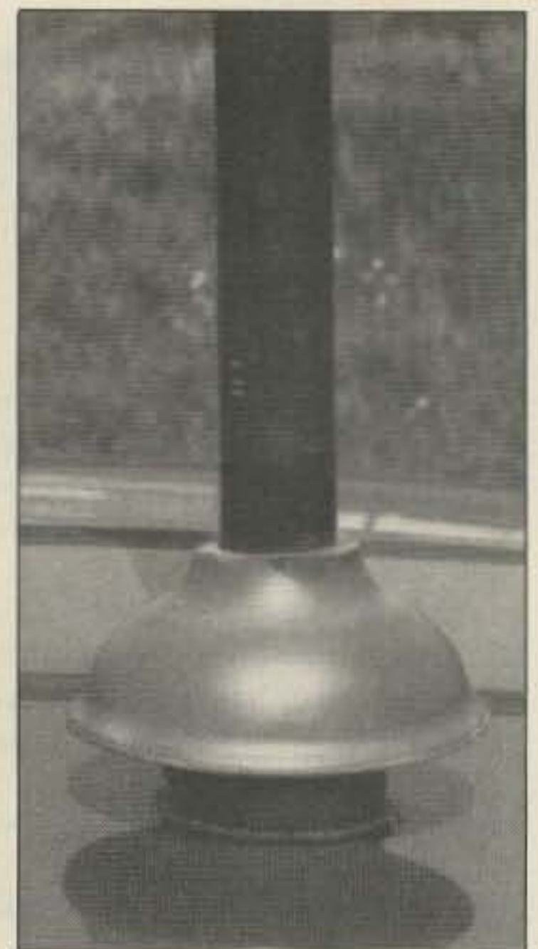
Photo B. It's not beautiful, but the plunger/rain deflector does the job, and you can move it from mast to mast.
