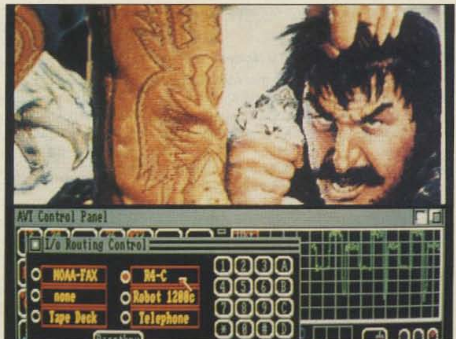
Photo C. The AVT control panel with I/O window open. The six icons on the screen are coupled to the six input jacks on the AVT interface board.
