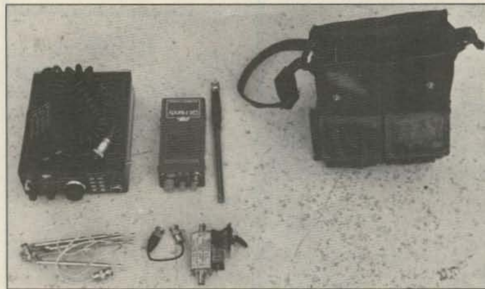
Photo A. Complete Mode-A station. It includes the FT-290 with telescoping antenna, the 10m DX handy, antenna stand with coax, and 10m GaAsFET preamp (with 9V battery and coax).
