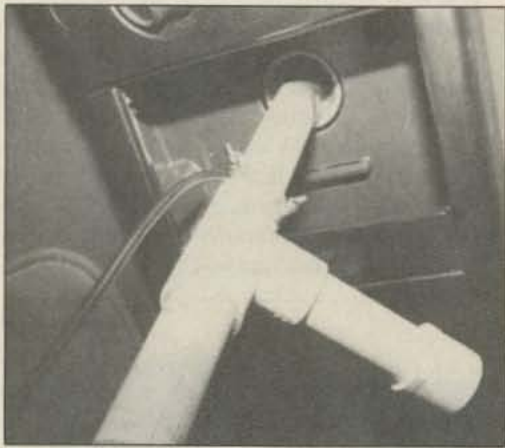
Photo C. The mast comes down through a trap door in the Astro roof console. The 4½-inch handle of PVC pipe allows lots of beam swinging without blisters.
