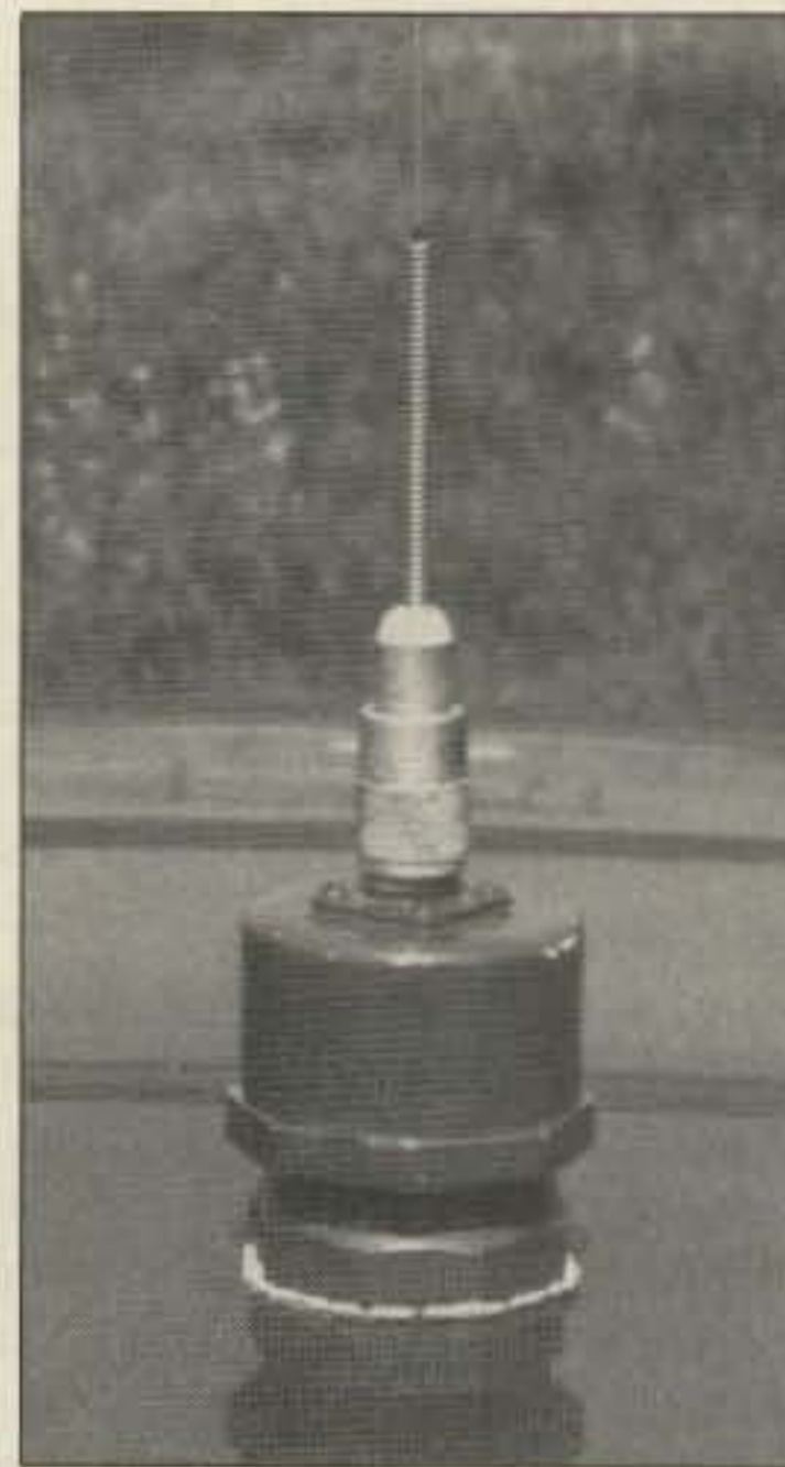
Photo A. When not in use for hunting, the roof hole bushing has a PVC cap. It makes a convenient mount for an extra whip antenna.
