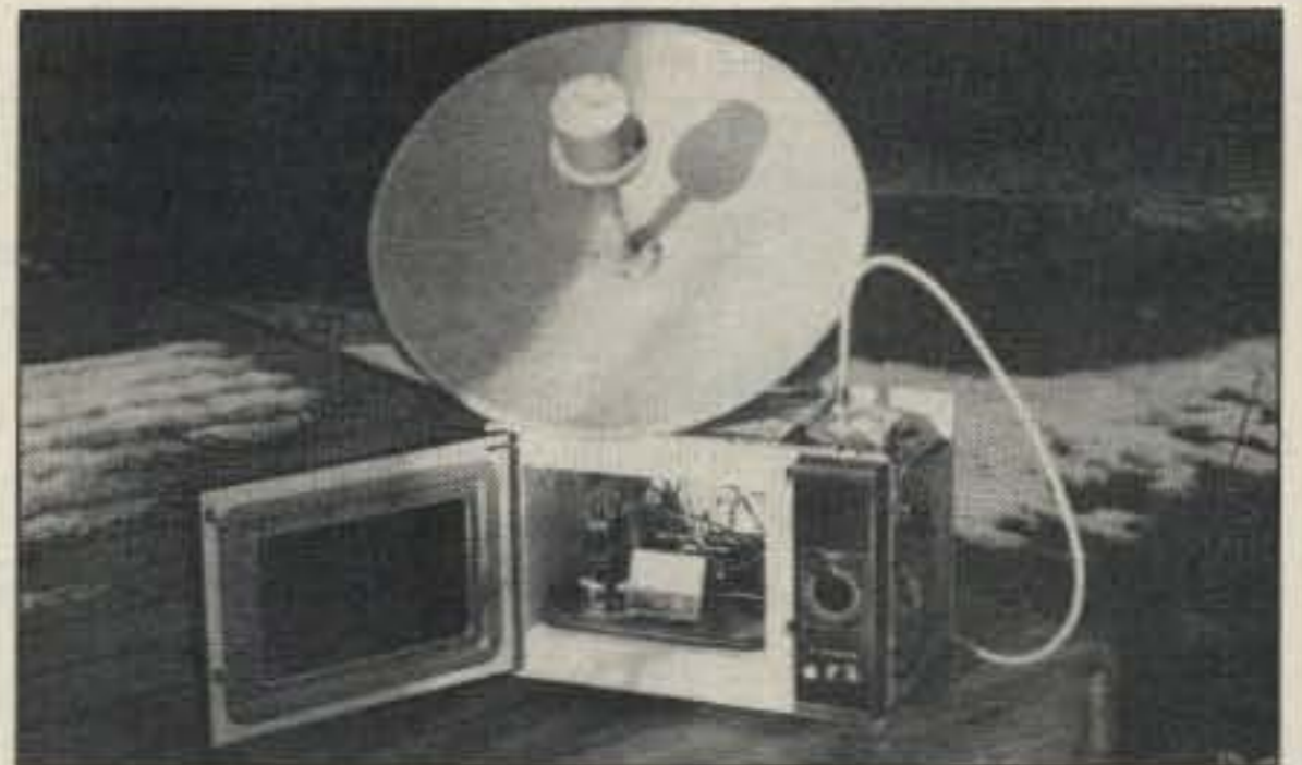
Photo F. The complete microwave oven ATV transmitter unit. The transmitter circuit is located in the oven's cooking chamber.
