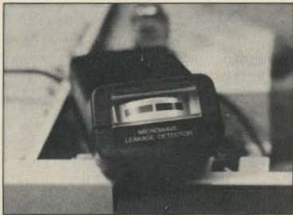
Photo E. Microwave leakage detector—a must for this project!
