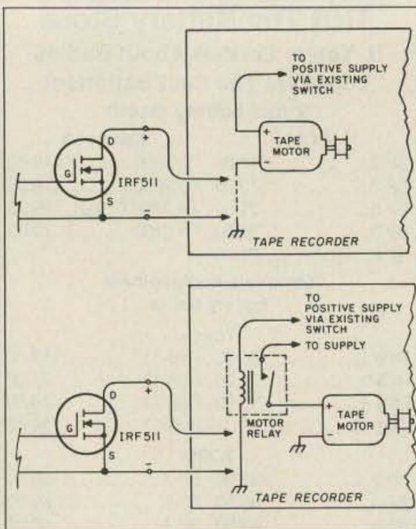
Figure 3. (a) Two methods of connecting the tape recorder controller to the motor of the recorder.
