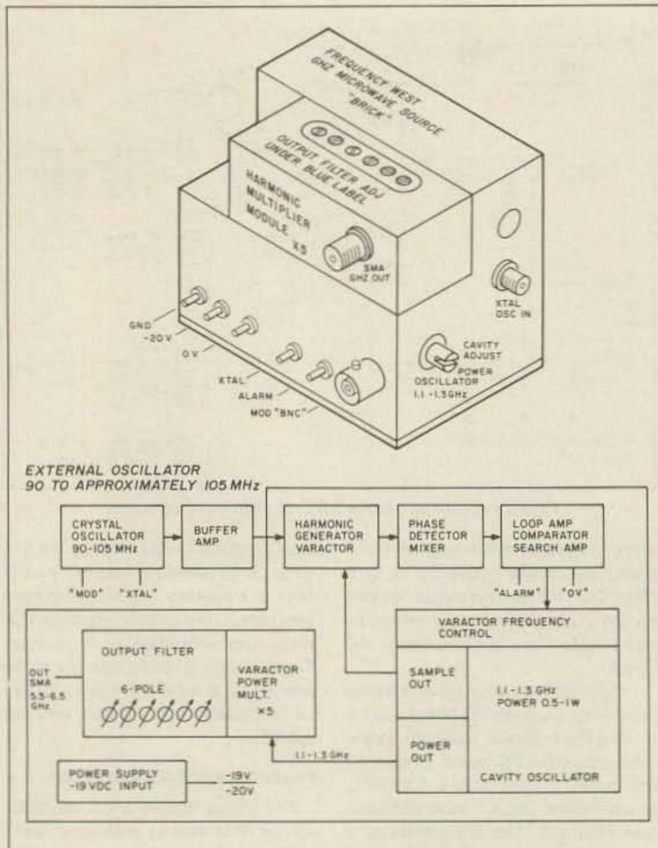
Figure 3. The microwave brick oscillator.
