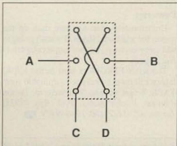
Figure 1. DPDT switch wiring details.
