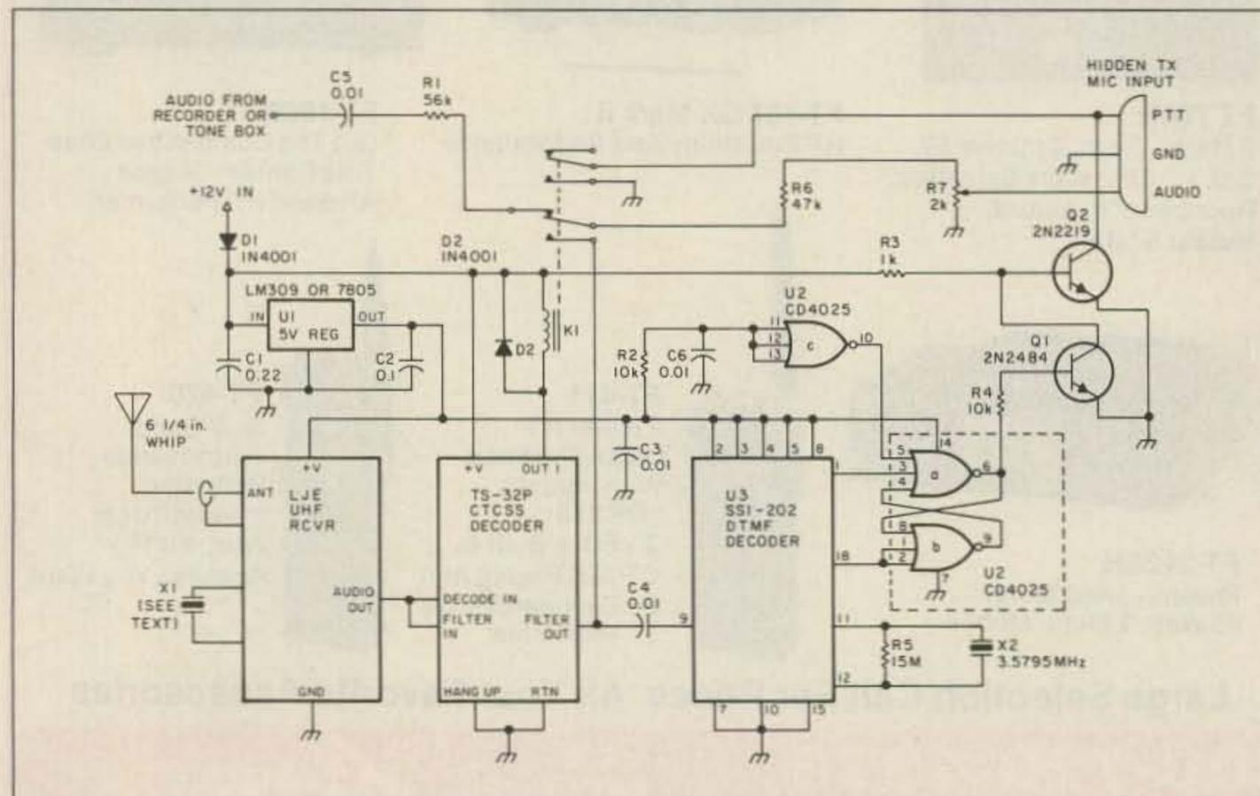
Figure 1. Schematic diagram of the Fox Commander.
