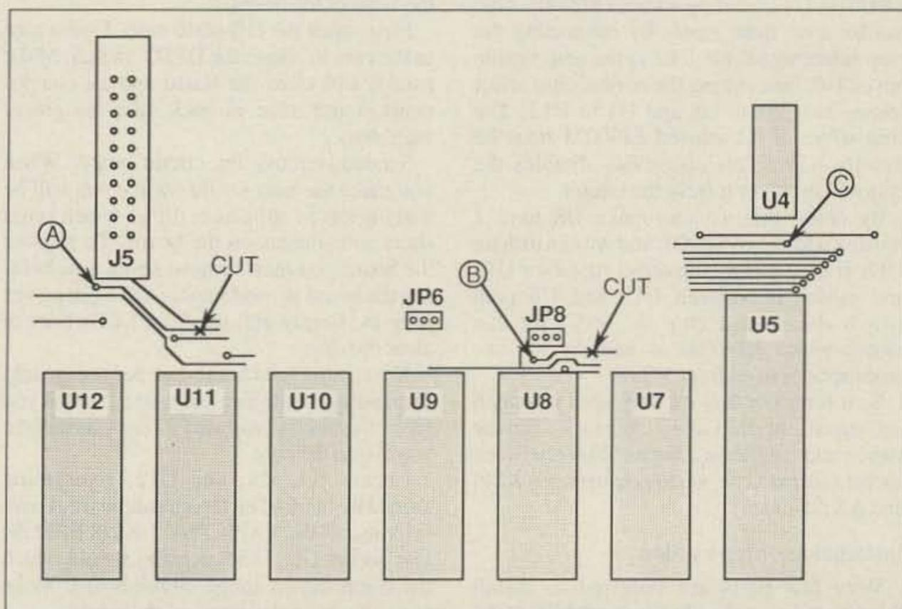
Figure 2. Location of wires A, B, and C on the TNC 1 circuit board (wire D connects to the 5 volt bus).
