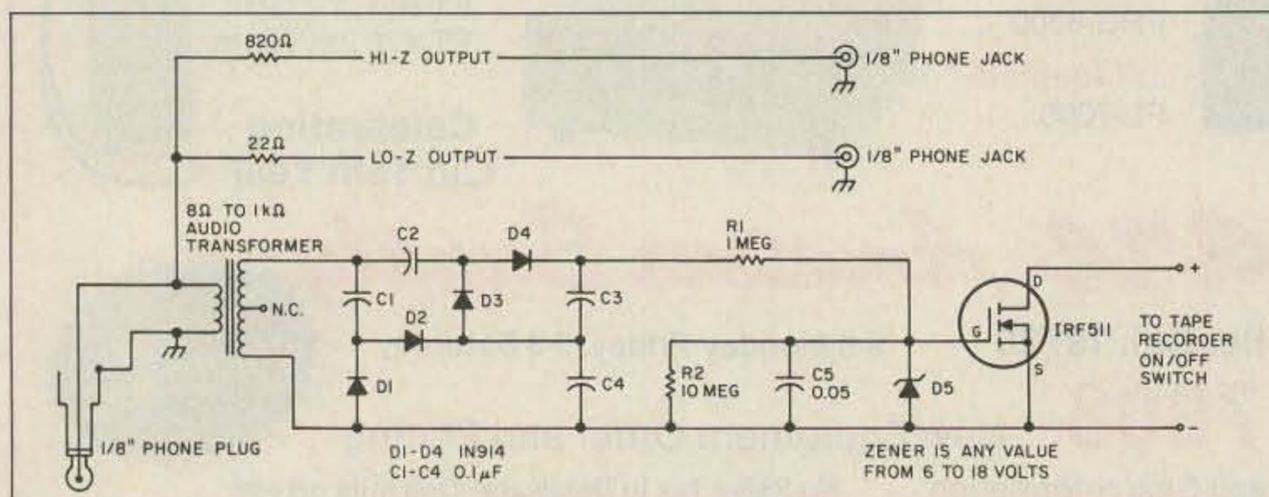
Figure 1. Schematic of the audio-powered tape recorder controller.
