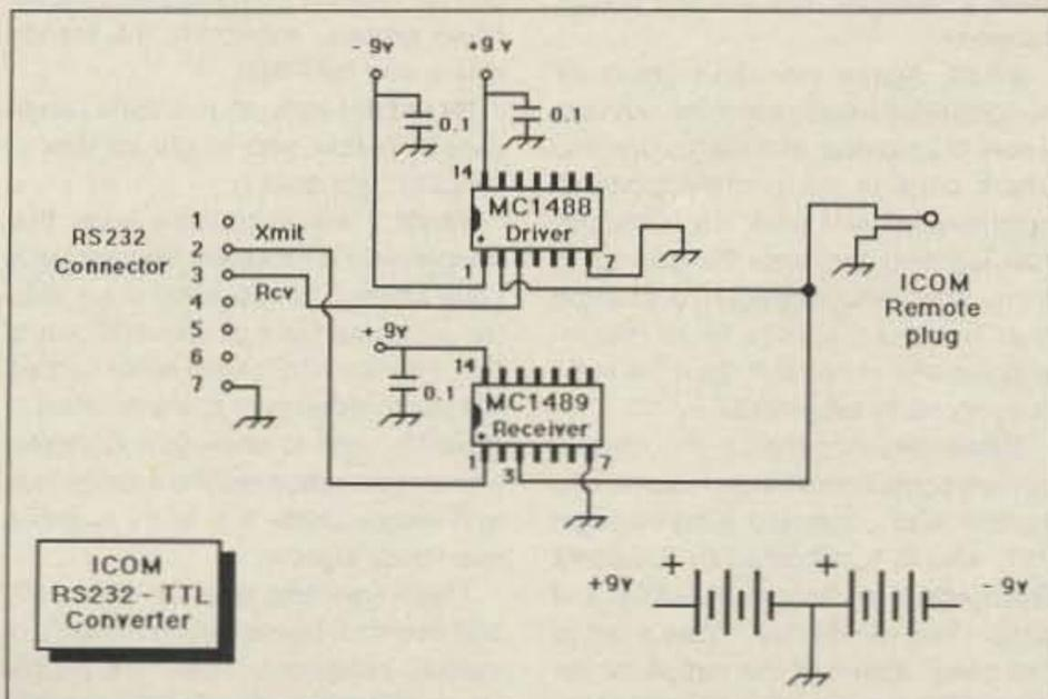
Figure. RS-232 to TTL converter.
