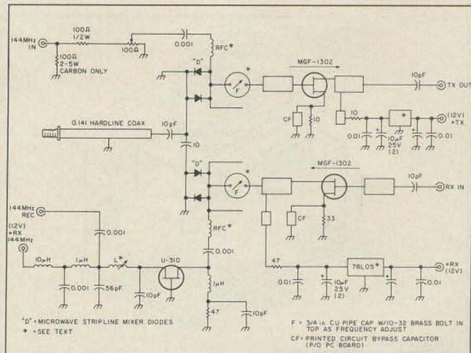
Figure 1. Schematic of the 5.6 GHz microwave converter.
