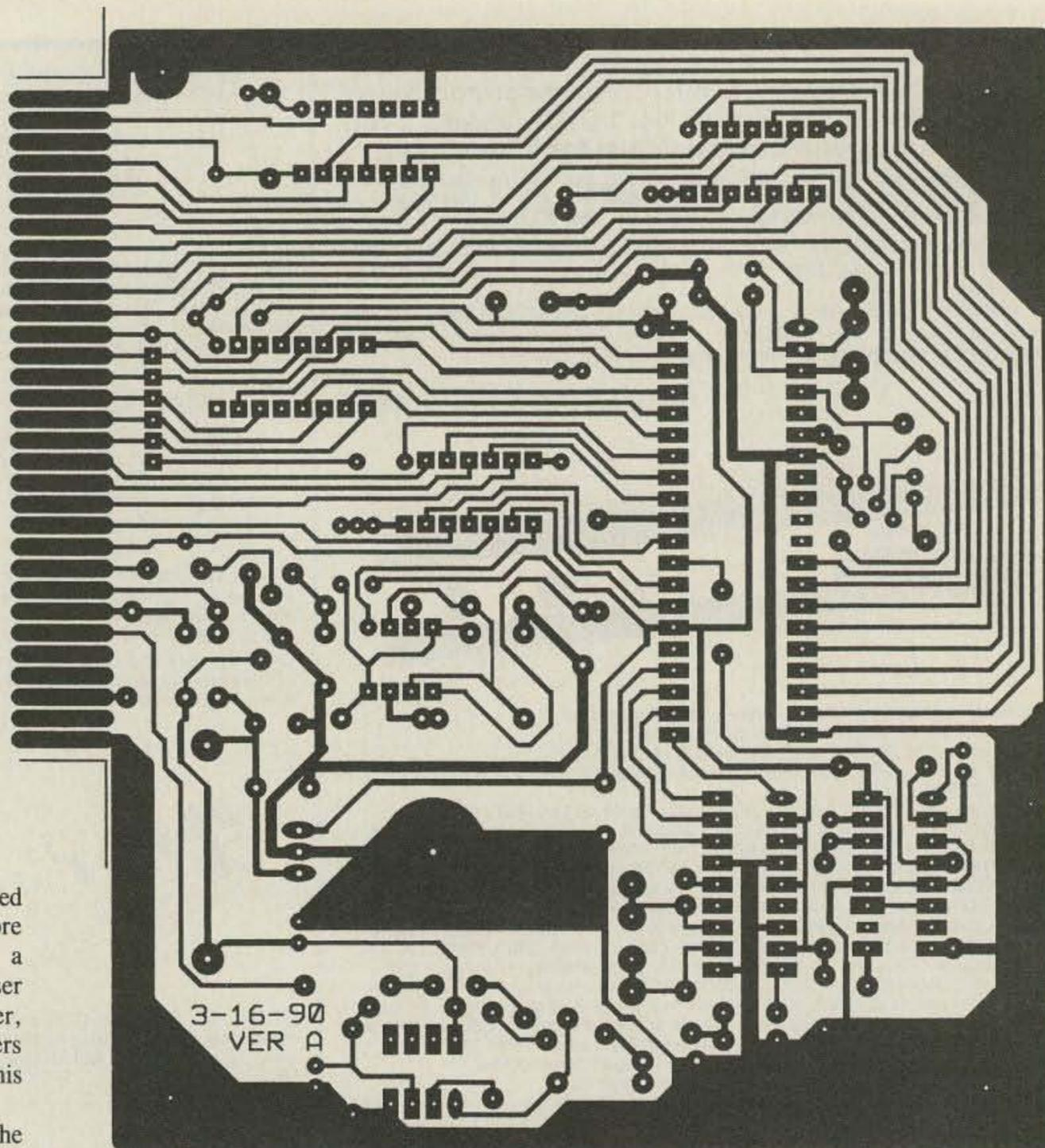
Figure 3. PC foil pattern for the computer board.
