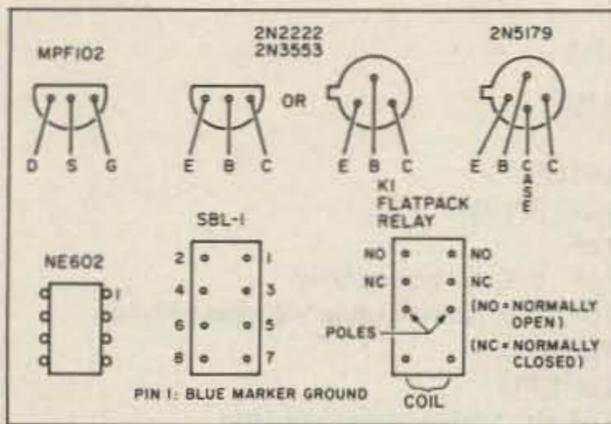
Figure 8. Base diagrams, all bottom view.
