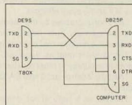
Figure 2. Typical cable connections for computers/terminals with DB-25 RS-232 ports.
