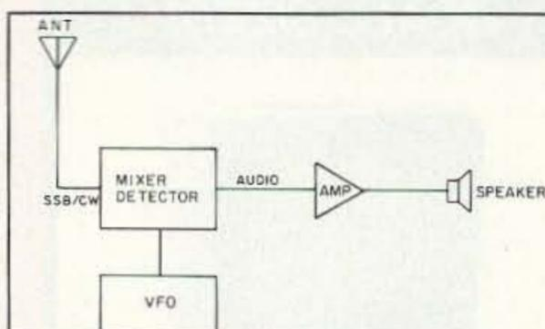
Figure 1. Diagram of the basic direct conversion receiver.
