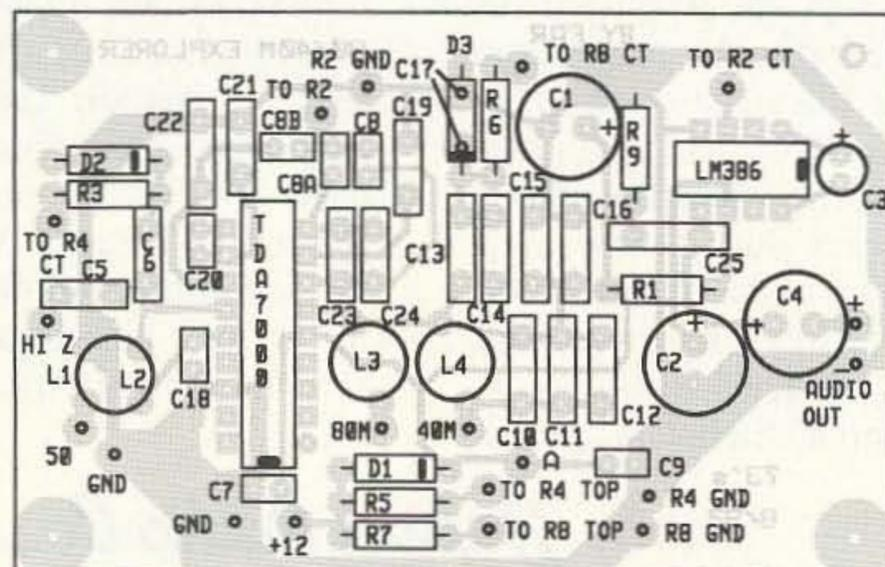
Figure 5. PC board parts placement.
