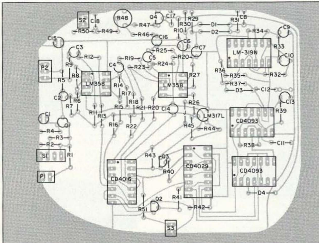
Figure 5b. PC board parts layout.
