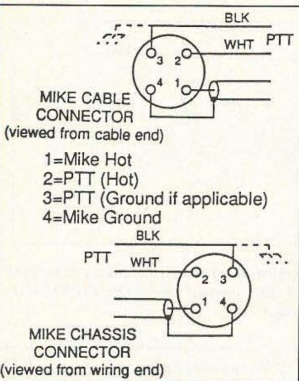
Figure 5. Microphone jack wiring to the SSTV interface.
