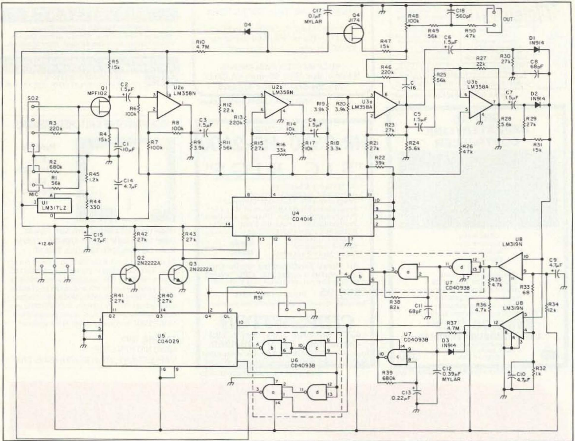
Figure 4. Schematic diagram of the digital ALC.
