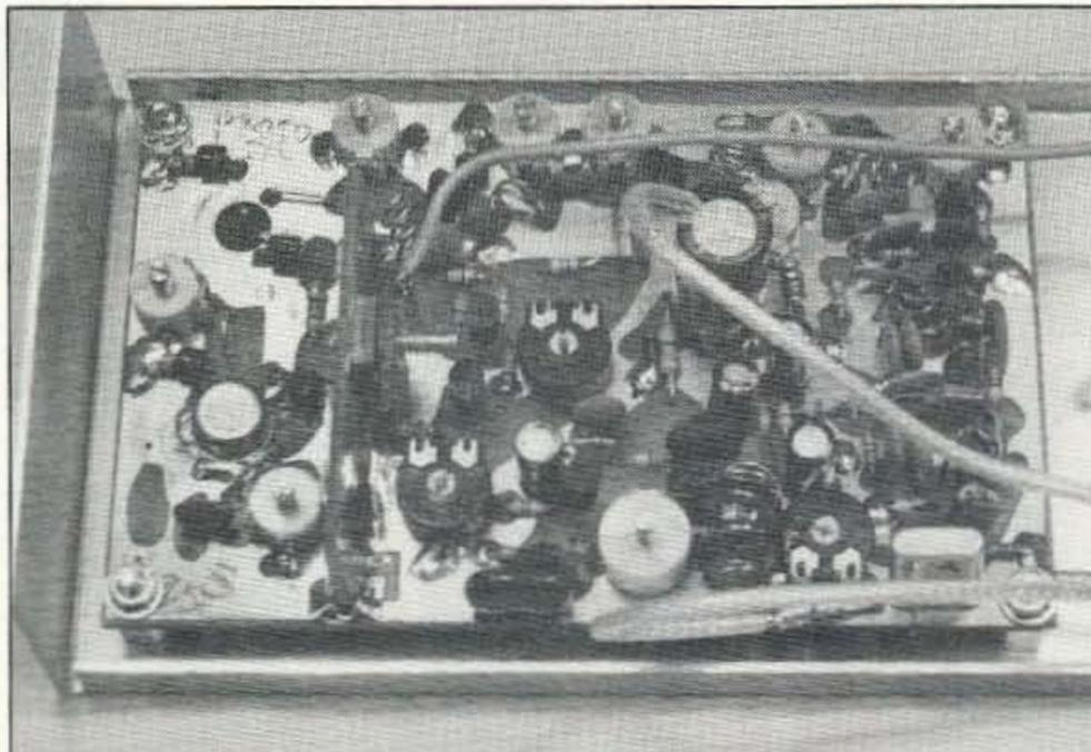
Photo. The 1-watt ATV transmitter.
