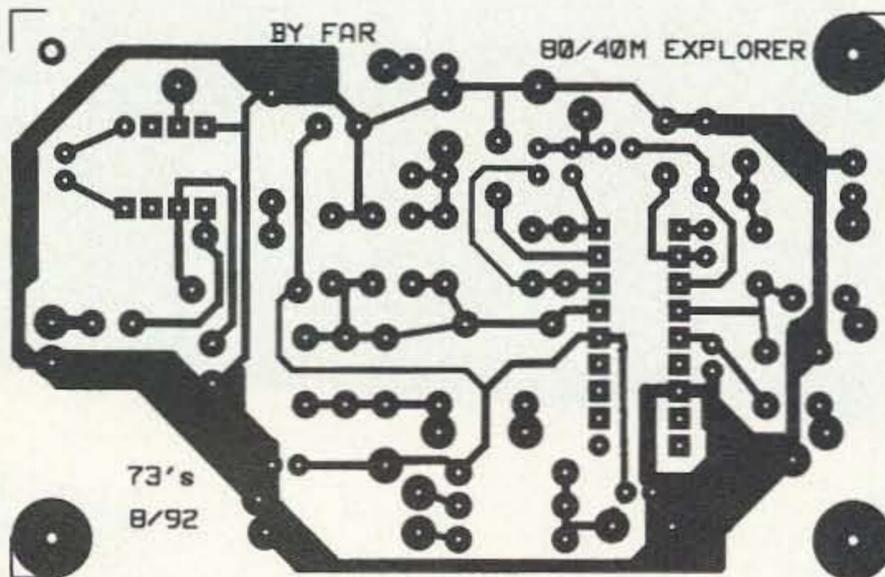
Figure 4. The optional PC board foil pattern.
