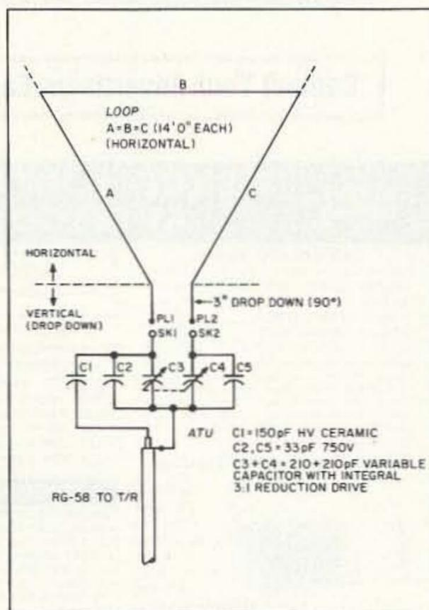
Figure 1. Diagram of the Compact-A-Loop.
