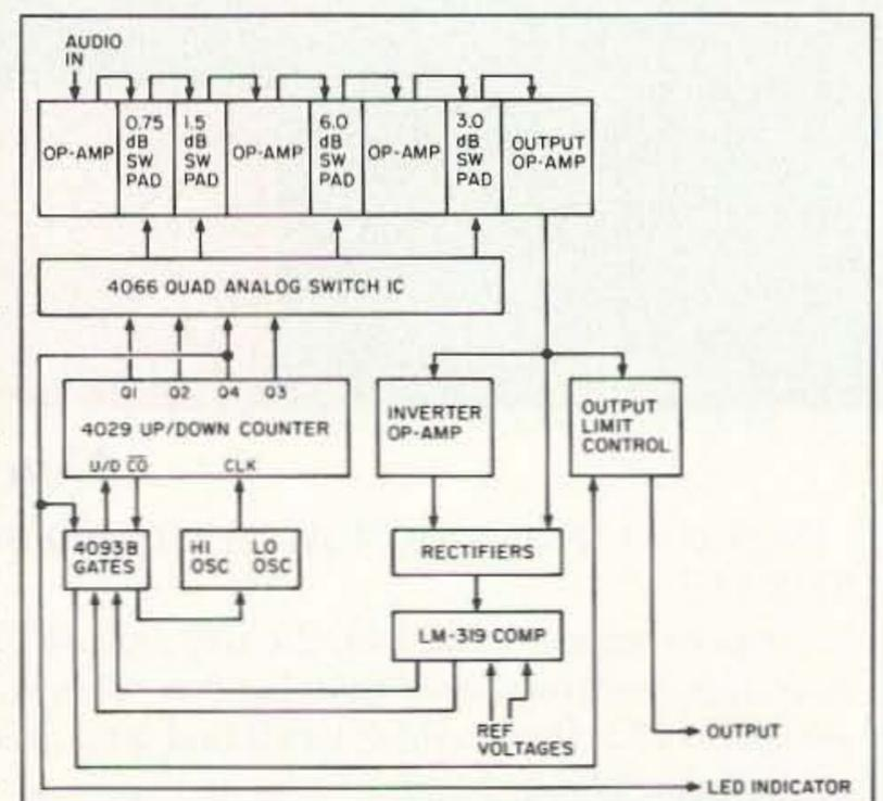
Figure 3. Block diagram of the Digital ALC.
