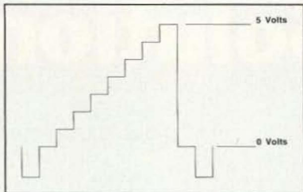
Figure 2. Waveform at TP-3 with gray-scale input.
