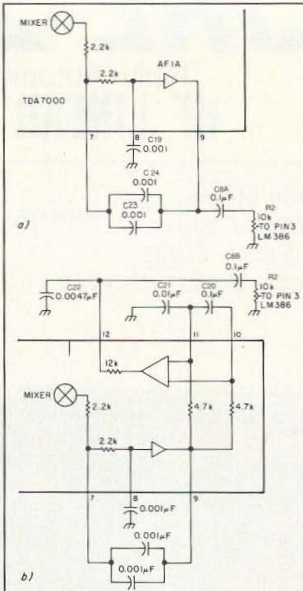
Figure 3. Schematic diagram for alternate audio selectivity using the internal op amps in the TDA7000.
