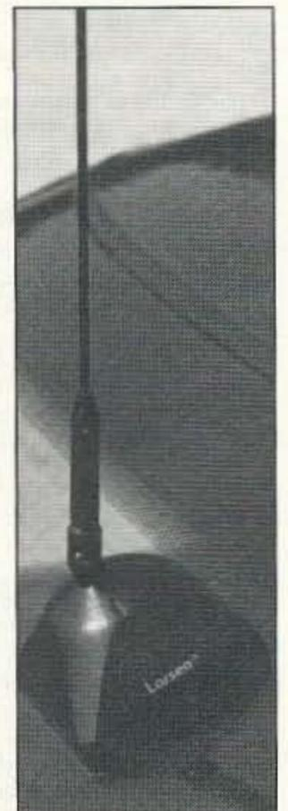
Photo A. the Larsen KG 2/70 mounts directly on glass.
