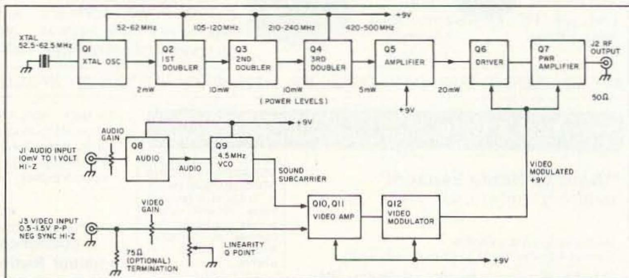
Figure 1. Video transmitter block diagram.
