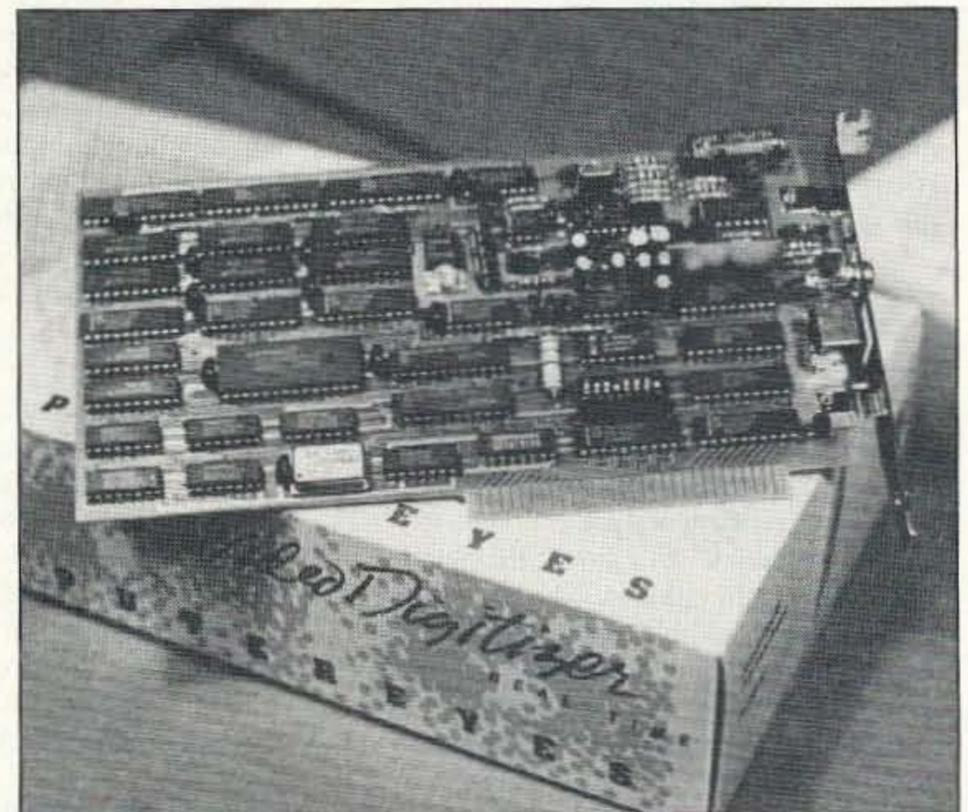
Photo C. The ComputerEyes R/T color frame grabber board from Digital Vision, Inc.
