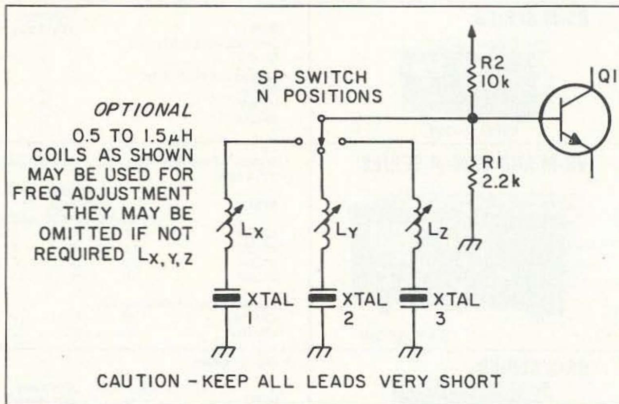
Figure 3. Scheme for XTAL switching.
