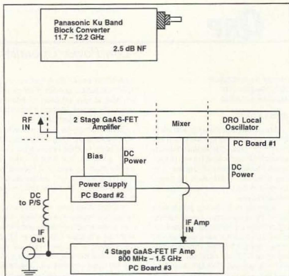
Figure 1. Ku band converter.
