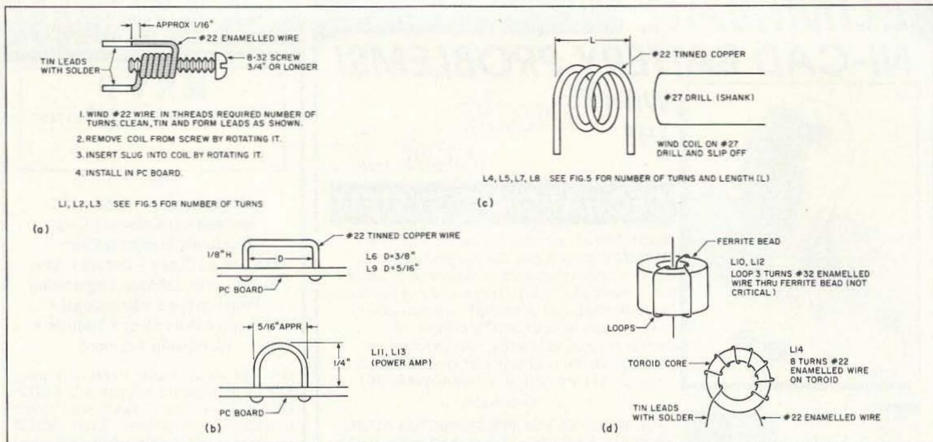
Figure 4. Coil construction.
