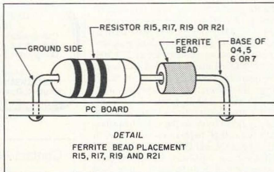
Figure 5. Using an RF choke on resistor leads.
