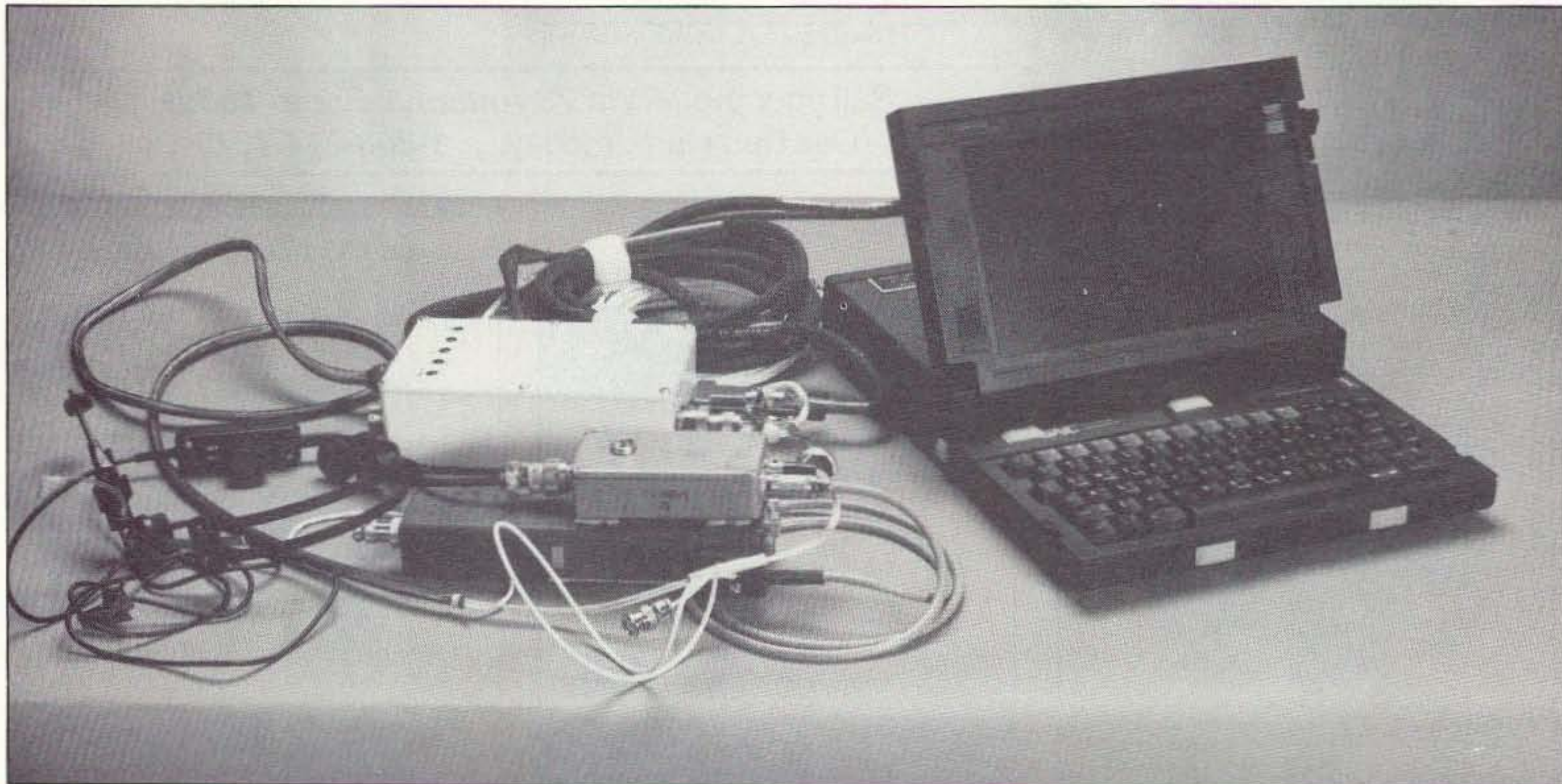
Photo A. Typical configuration "C" for SAREX voice and packet. (NASA photo.)
