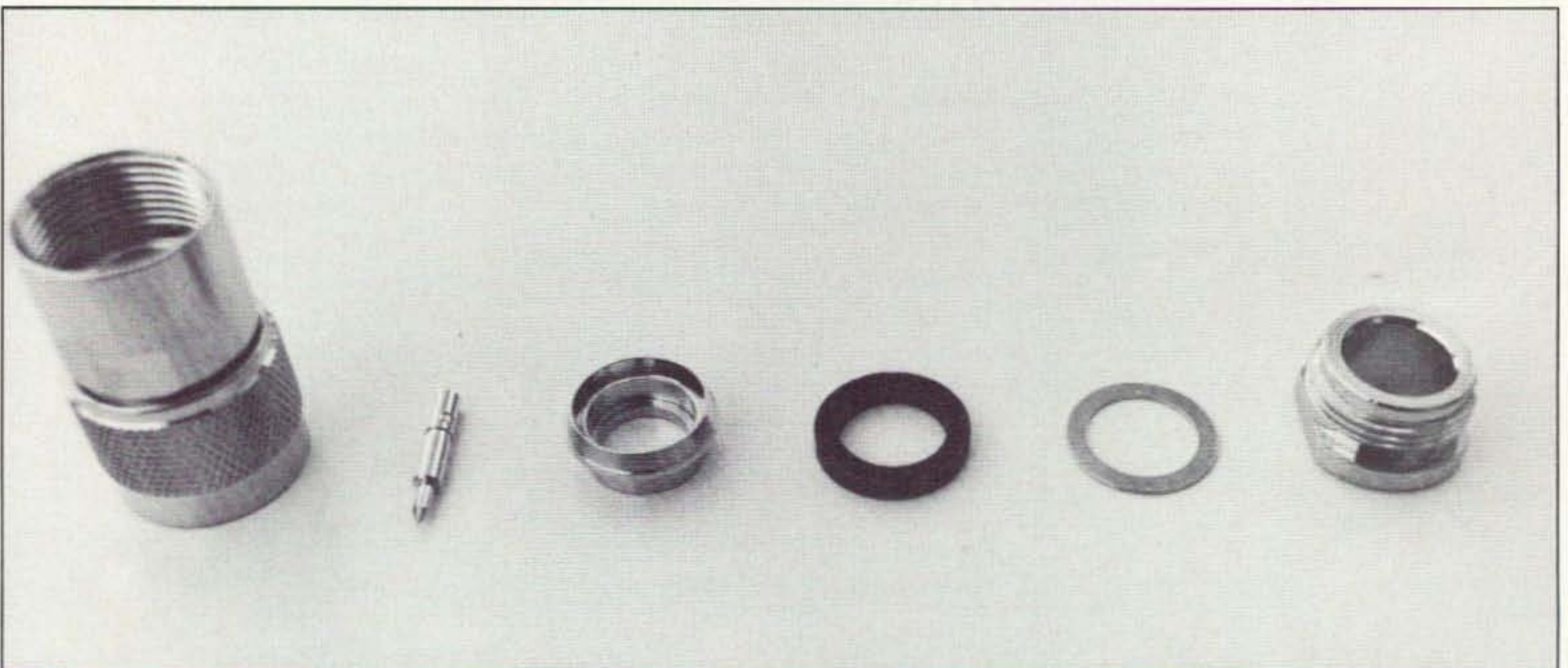
Photo A. Here are the six pieces that make up a standard UG21D/U type N connector (left to right): the body, the center pin (note the gold plating), the braid clamp, the rubber gasket, the washer, and the nut.
