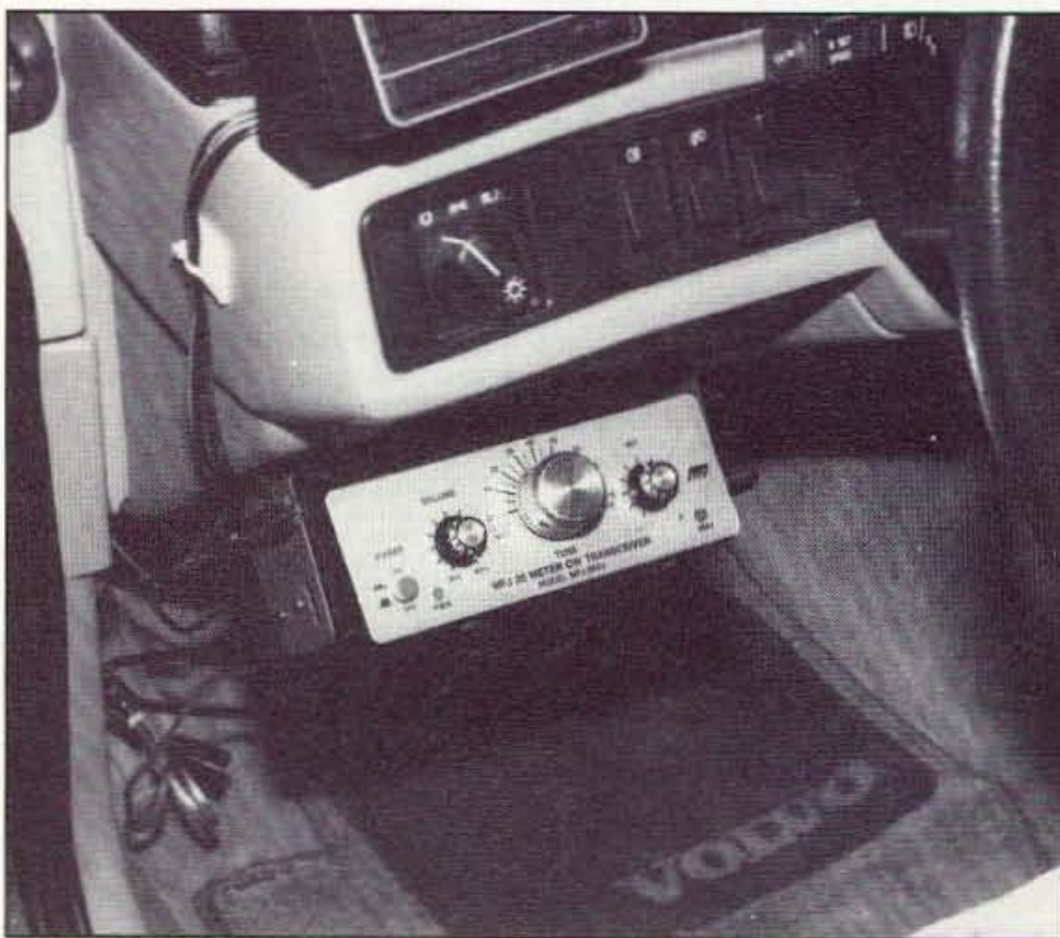
Photo A. The little MFJ QRP-CW rig will mount just about anywhere, and is so light that a plastic dash will hold it just fine. I used an old bracket from a Radio Shack CB rig (or something), modified slightly for the MFJ rig.
