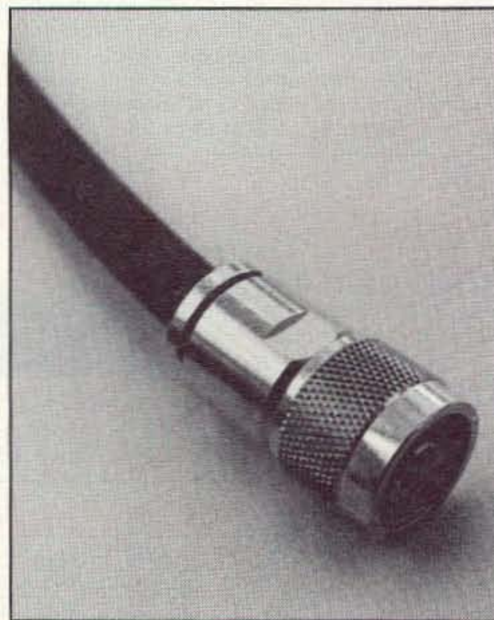
Photo D. The completed, installed type N connector. When the rear nut was tightened a very small space remained between the nut and the connector body. This is perfectly normal. Using high-quality, open-end wrenches for final assembly avoids scratching or nicking the connector plating and leaves a shiny, weatherproof surface.
