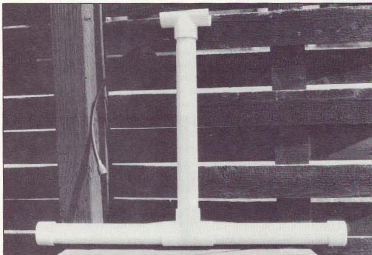
Photo E. The completed 440-450 MHz antenna, ready for mounting.
