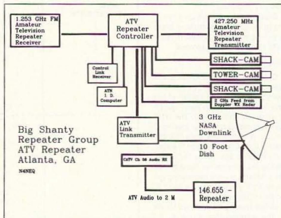
Figure 5. Block diagram of the BSRG's ATV Repeater.
