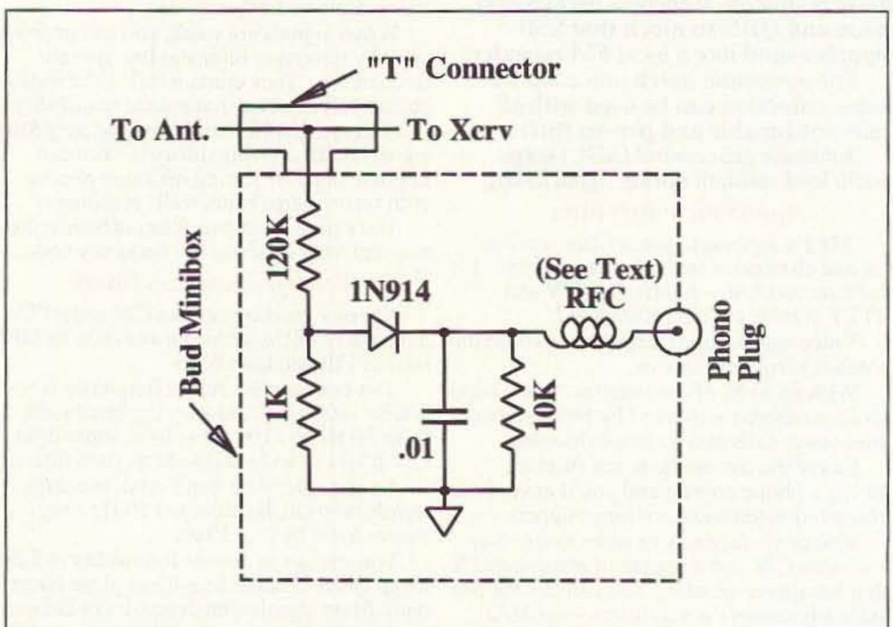
Figure 2. Schematic for the RF Sampler.
