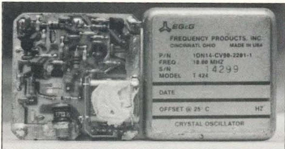
Photo A. TCXO oscillator: 10 MHz, temperature controlled.
