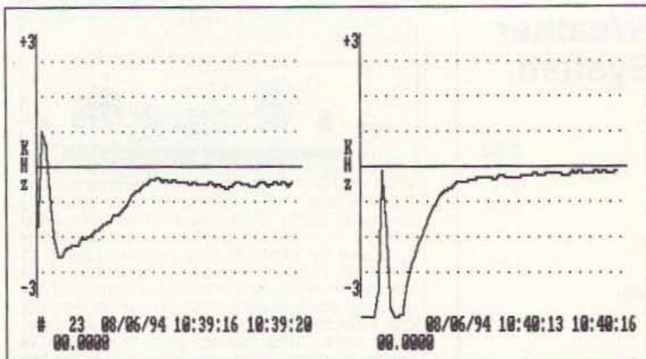
Figure 3. These two HTX-202 transceivers were bought at the same time, but have distinctly different fingerprints. They were set for the same power level on the same frequency.
