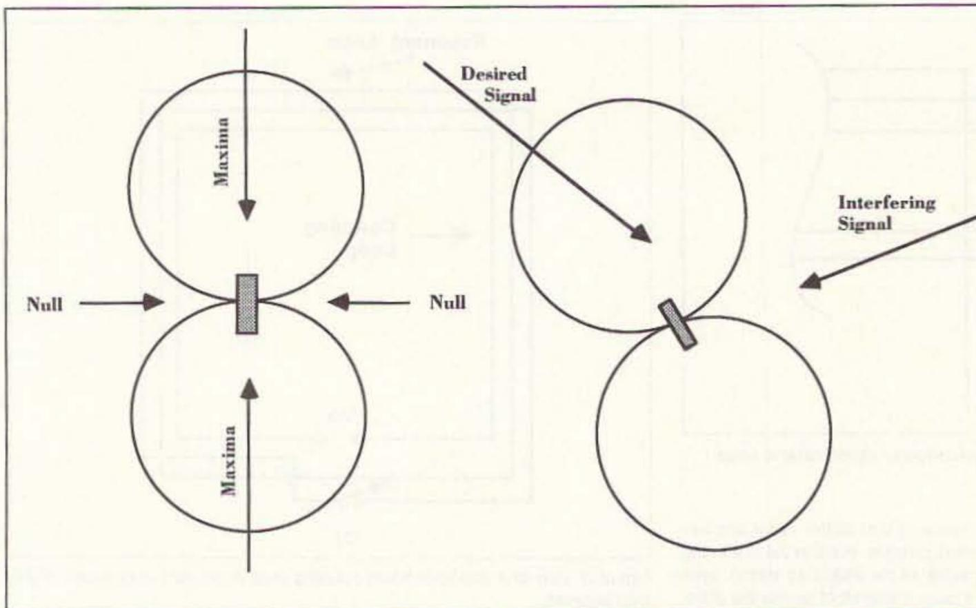
Figure 4. A) Azimuthal pattern of the loop (shown from above). Note that the nulls are broadside to the loop winding. B) Use of the loop's nulls to reduce an undesired signal.
