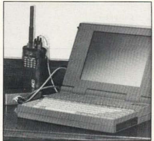
Photo B. The author has installed a Poor Man's Packet modem in a case and added a TTL/RS-232 converter to operate the modem through the PC serial port.
