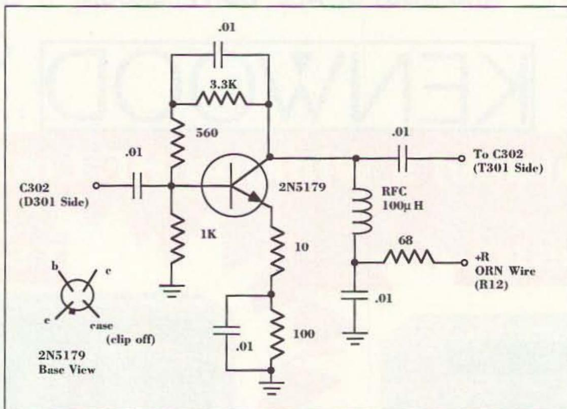
Figure 1. Preamp schematic.
