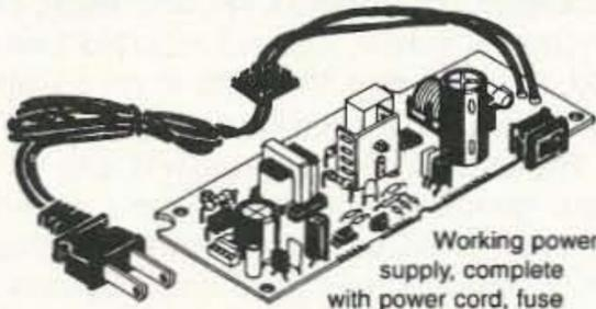
Working power supply, complete with power cord, fuse and on/off switch. Removed from Seikosha # SP-2400 dot matrix printer. We don't have the official specs on these, but they appear to have two outputs providing 5 and 24 Vdc. Great for educational and experimental projects. The parts alone are well worth the price. 6.25" X 2.69" X 1.45".
