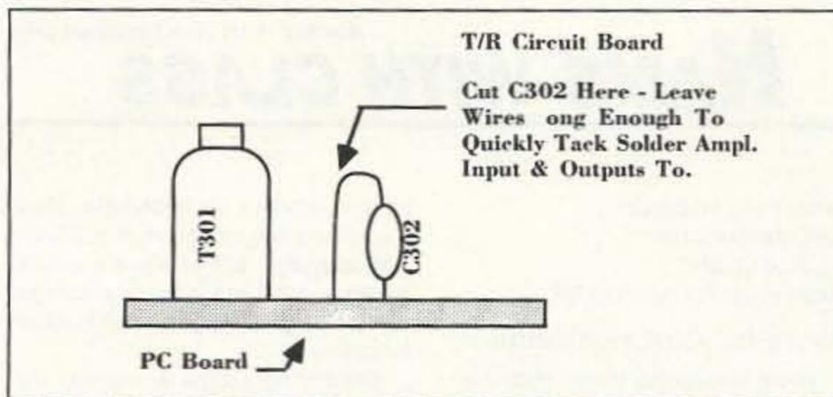
Figure 2. Connecting the preamplifier.
