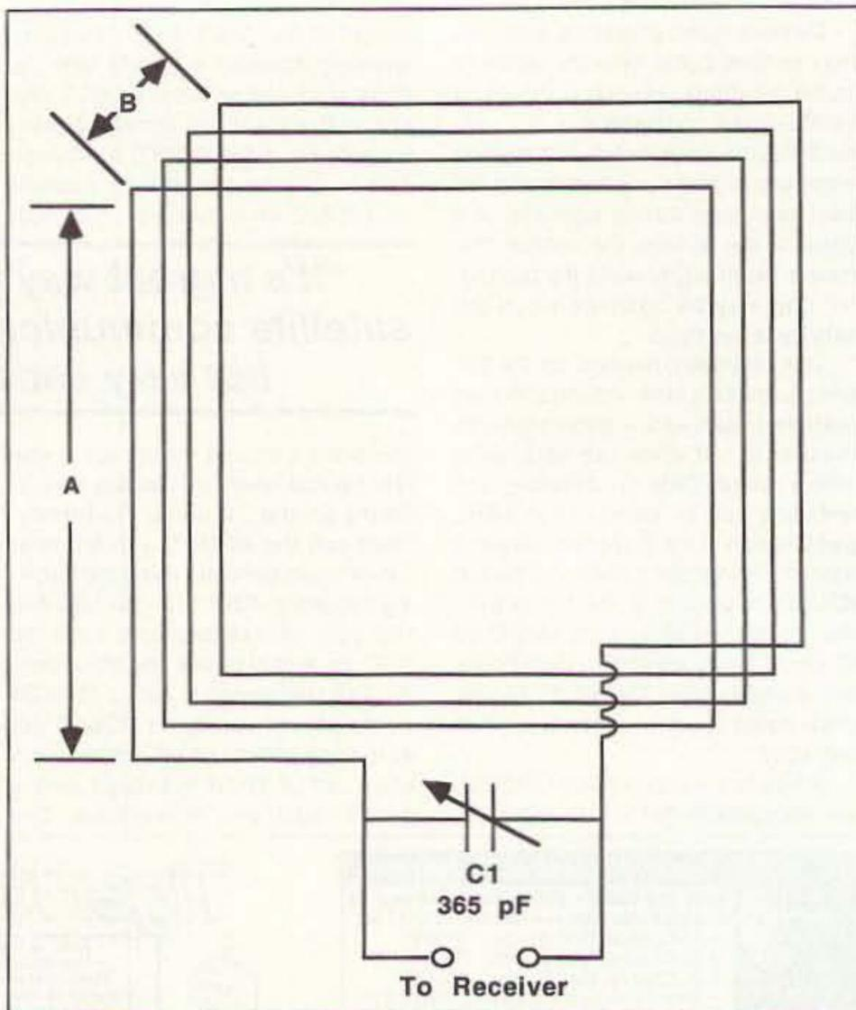
Figure 1. Schematic of the square loop antenna.
