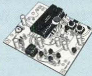
**TD-4 SELECTIVE CALLING Module.** Versatile dtmf controller with 1 latching output. Mutes speaker until someone calls by sending your 4-digit tt code. Or use it with a long tt zero digit to alert anyone in club. Also may be used to control autopatch or other single device. ....kit \$49, w&t \$79
