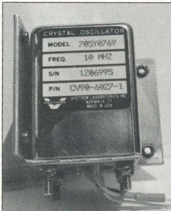
Photo B. OCXO oscillator: 10 MHz, oven controlled.
