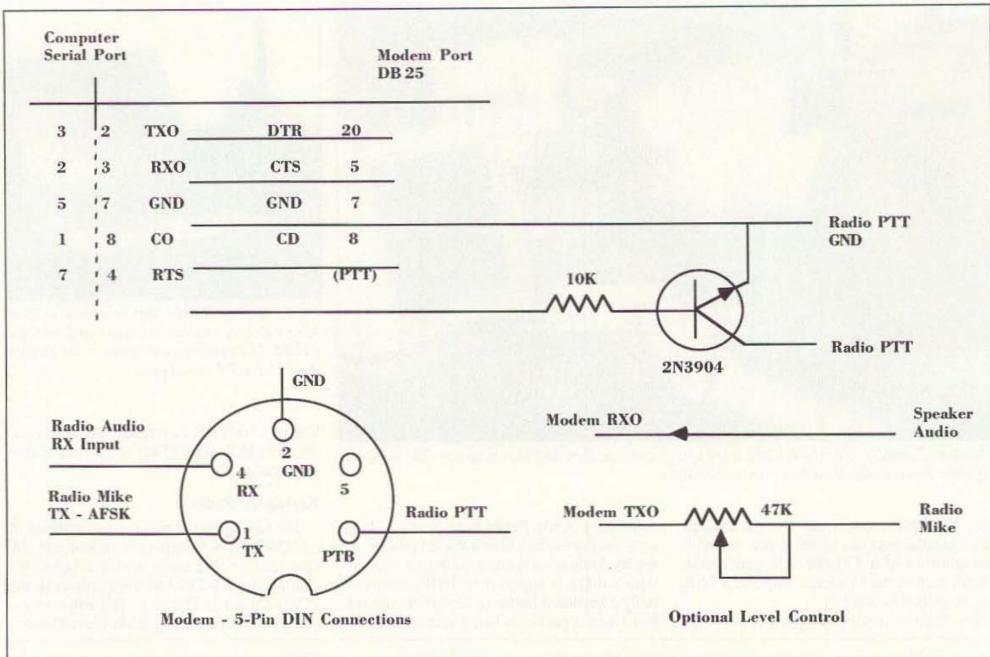
Figure 1. Wiring diagram. This circuit and computer connections will adapt Bell 202 modems for use with PMP, Baycom, or SoftTNC. A variable resistor in the transmit output may be added to reduce audio level into the radio transmitter.
