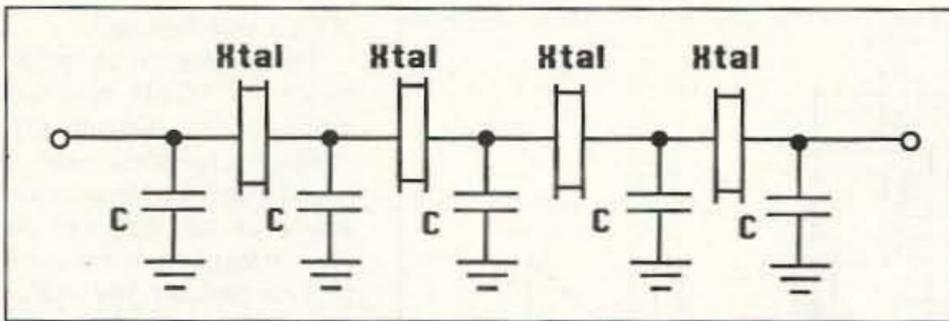
Figure 2. Crystal ladder filter, constructed from four matching crystals. Capacitor values are approximately 15 to 30 pF.
