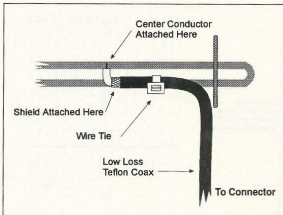
Figure 2. Feedline assembly.
