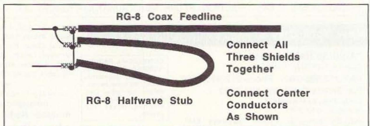
Figure 2. Half-wave phasing section detail.
