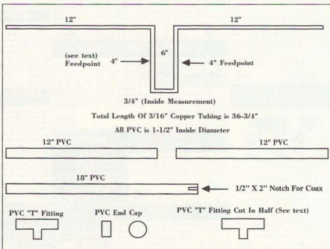
Figure 1. 440-450 MHz PVC base or repeater antenna.
