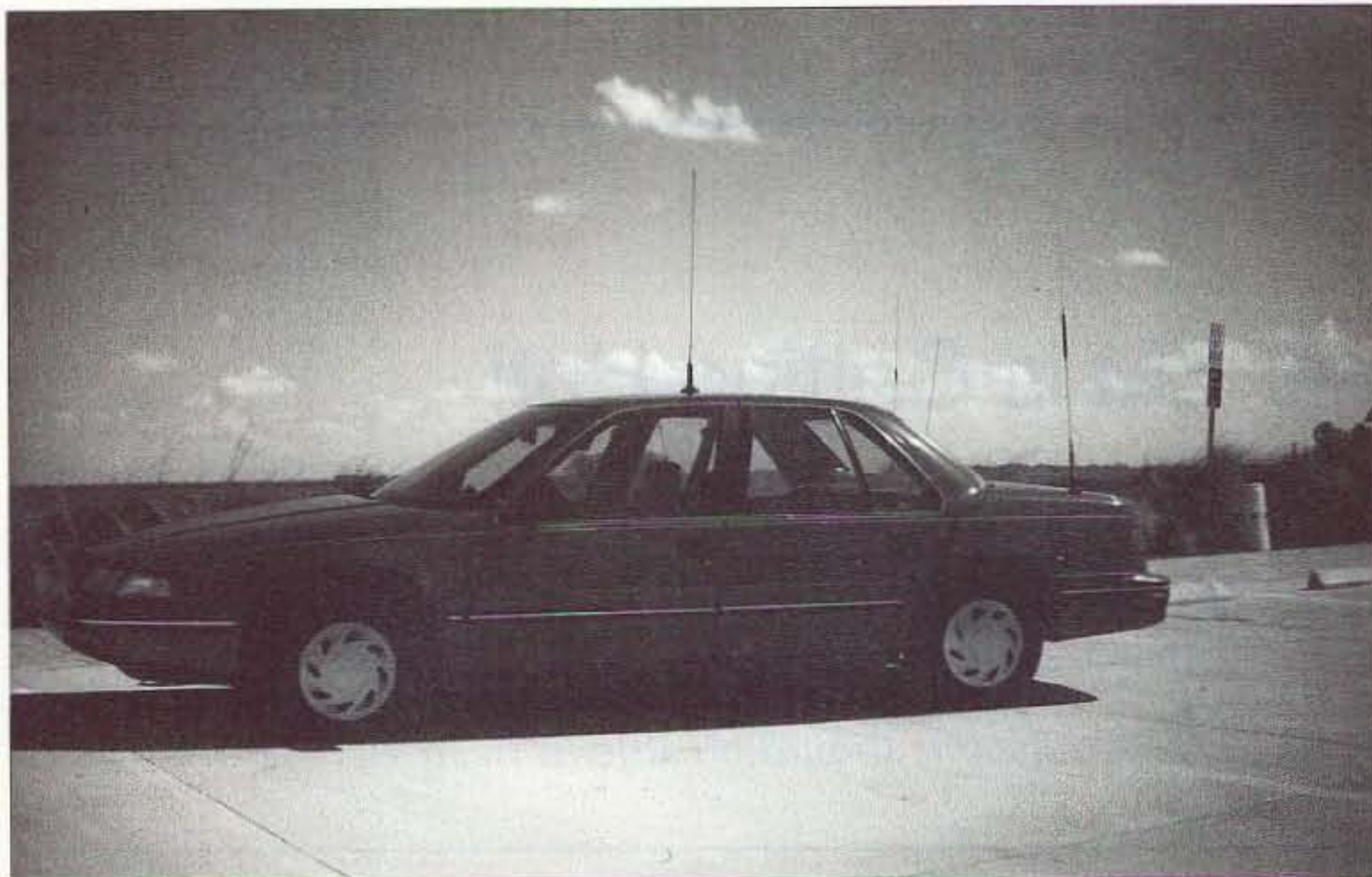
Photo B. 10 meter antenna mag-mount on roof complements 20 meter and VHF/UHF antennas on trunk lid.
