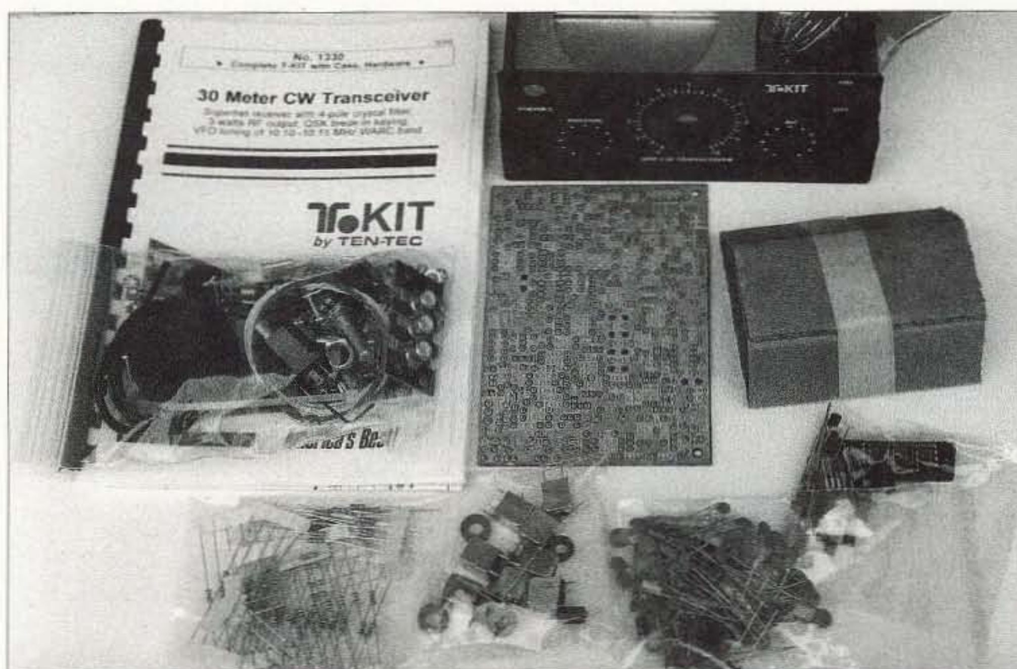
Photo A. If you like building kits, you will love QRP. Here, a Ten-Tec QRP transceiver kit is laid out and ready for assembly. The little gem has approximately 200 parts, and thus requires around 15 hours for assembly and checkout. Then it is ready to work the world! Now, who could resist such an attractive challenge?! (Photo courtesy of K4TWJ)
