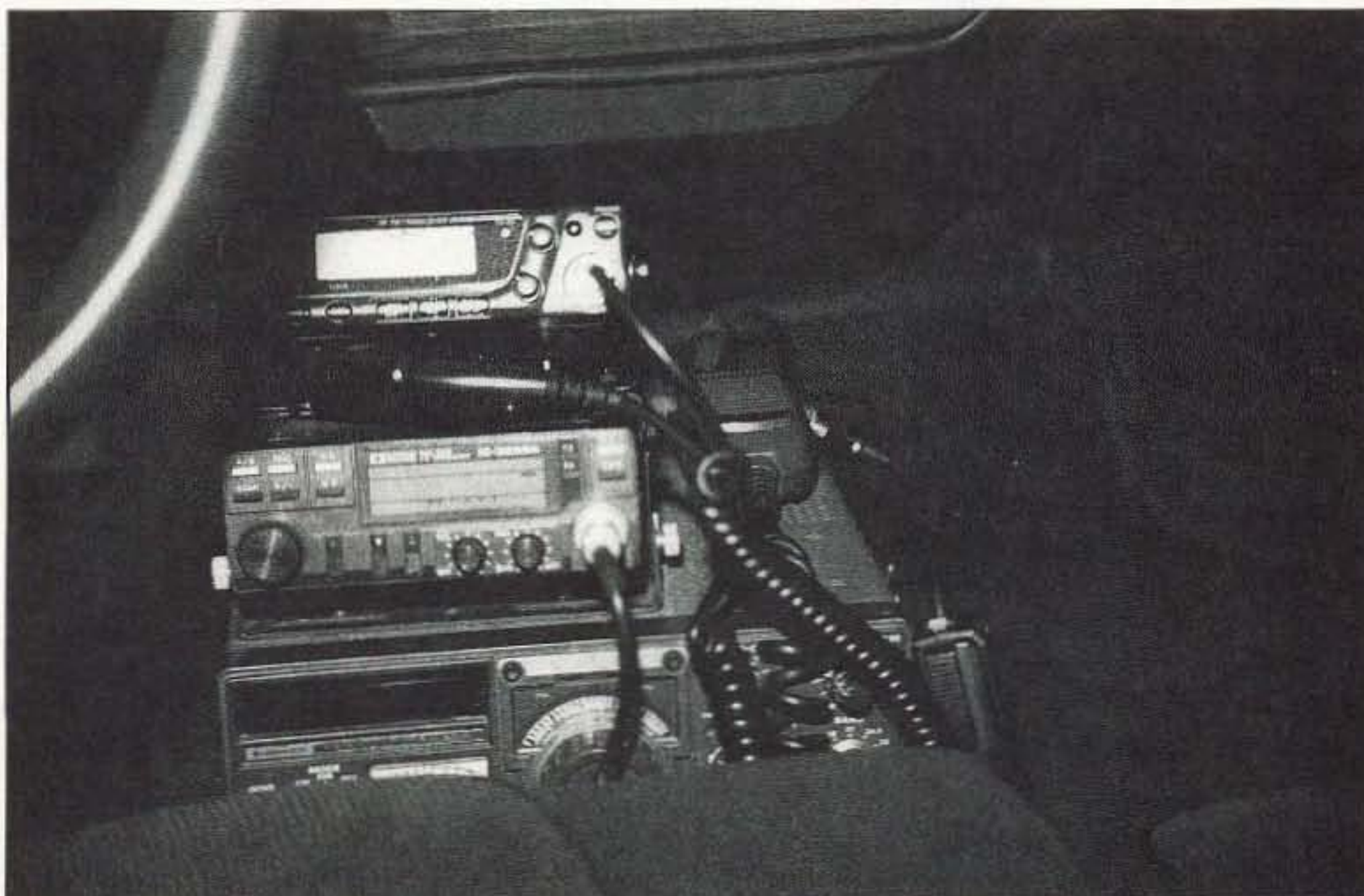
Photo A. Room for one more — Alinco DR-M03 mounted on top of 2m/440 and HF rigs.
