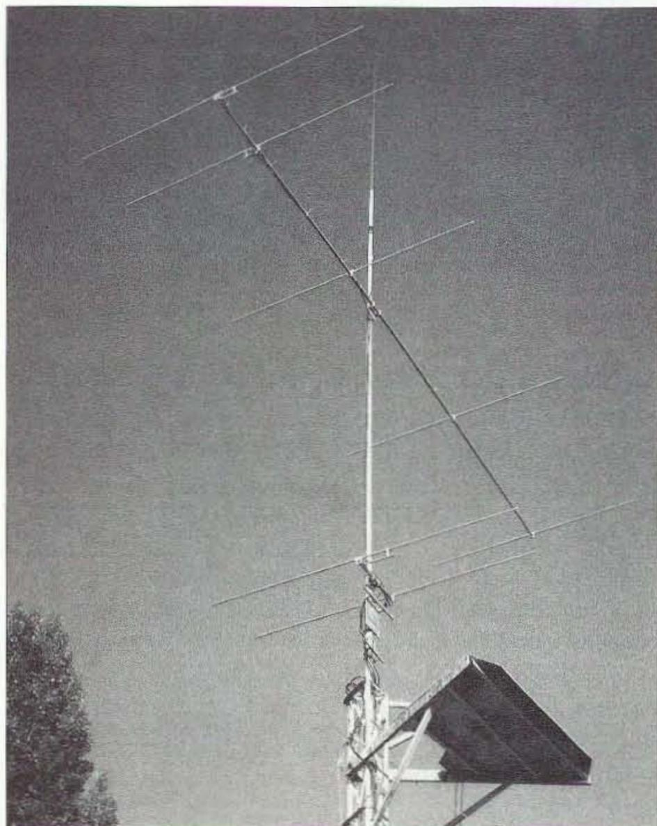
**Photo D.** 5- over 2-element 6m Raibeams with 1/2-wave vertical on top used as a listening antenna. These two beams can be selected individually or both together in phase. Various configurations are being tried to obtain different angles of radiation individually or phased together, or differences in polarization to create different angles of radiation to compensate for polarization shift.
