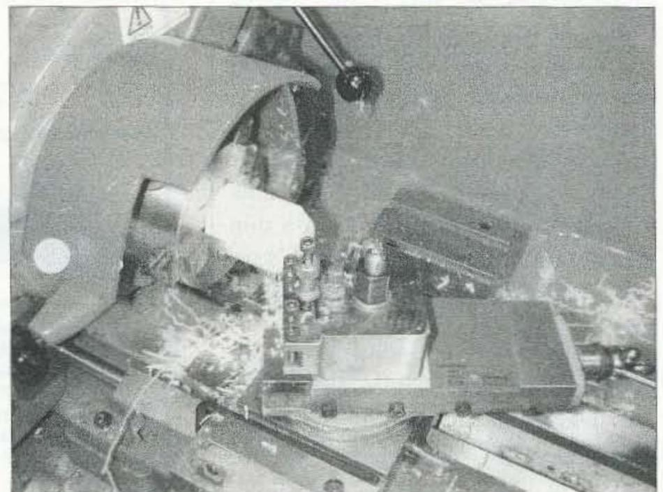
*Photo I. Turning the large mandrel cones.*
