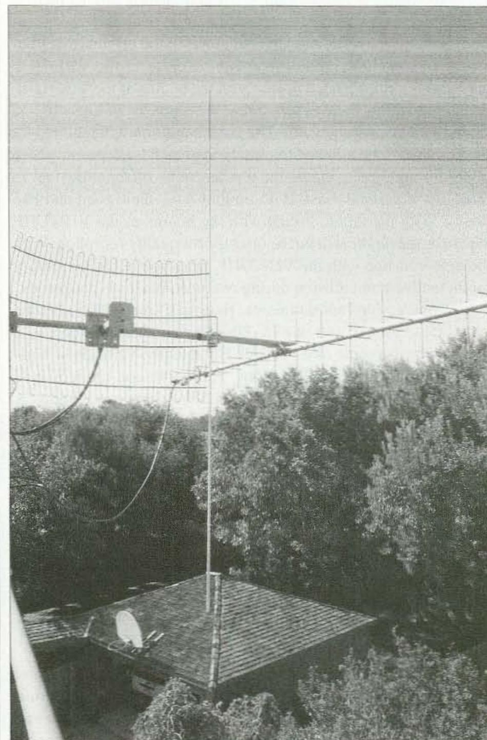
**Photo G.** The finished short 10-meter dipole mounted between the 70-cm yagi and the 13-cm semi-dish/downconverter.
