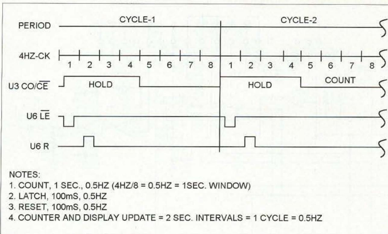
Fig. 6. Timing diagram counter section.
