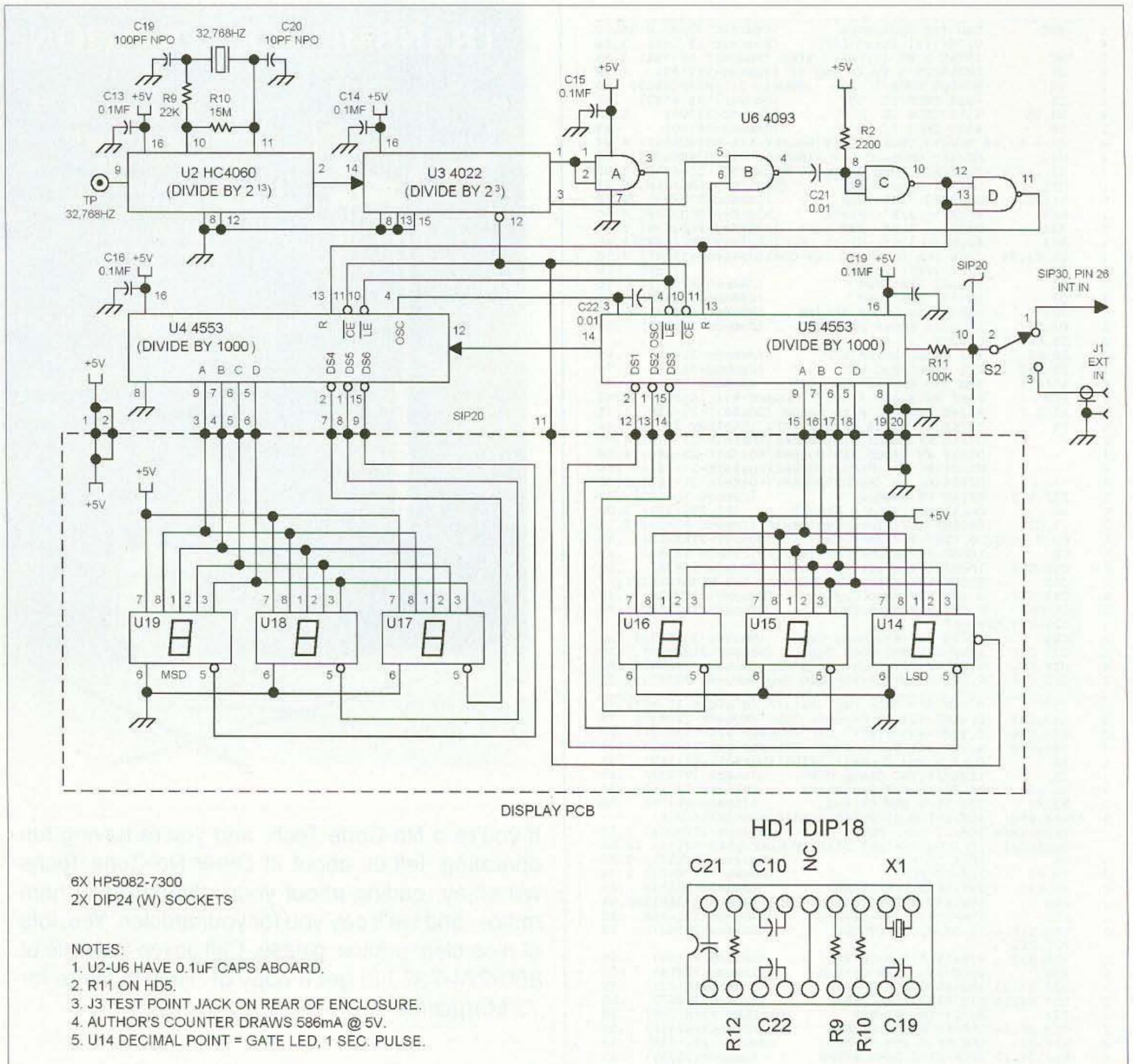
Fig. 4. Schematic, counter section.
