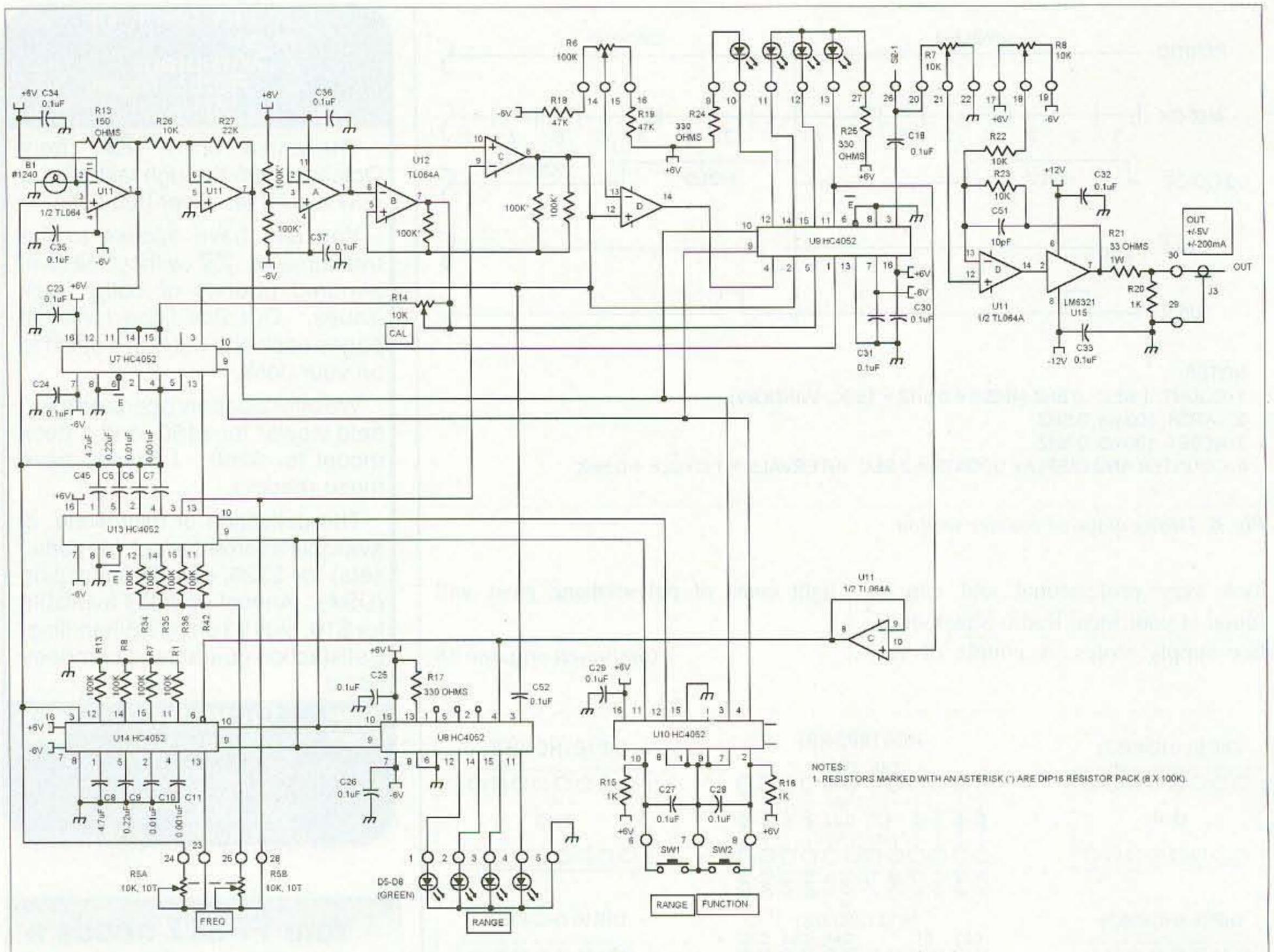
Fig. 8. Schematic, function generator section.
