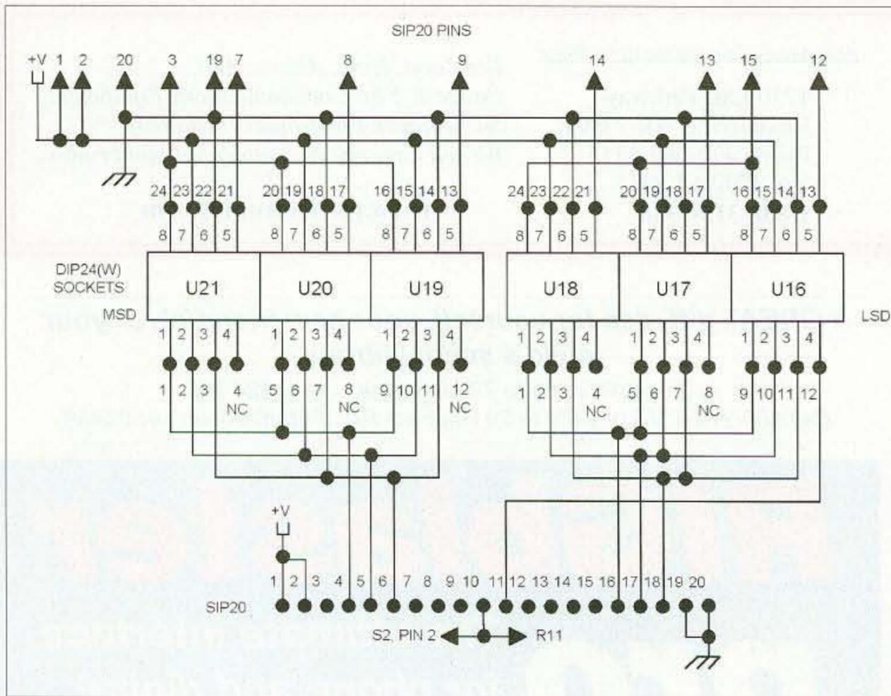
Fig. 5. Schematic, counter display section.
