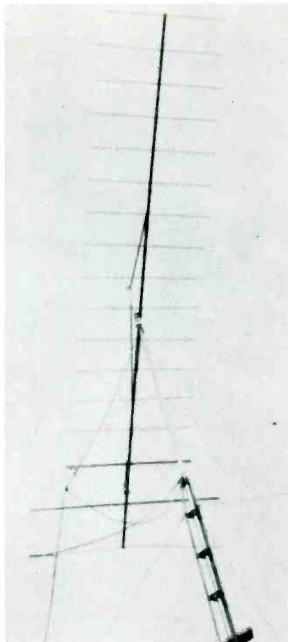
Hosken's 17 element low band (2-6) yagi. 15 db. gain.
