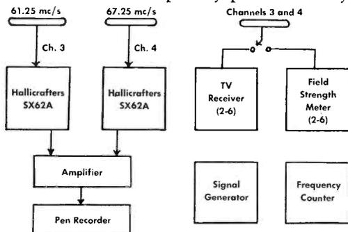
source of signal at the frequencies where Es is of marginal effectiveness. In the light of this, it was thought worthwhile to attempt to obtain some statistical data on the frequency of occurrence of Es, using a system of continuous monitoring of television channels. In the Calgary area Channel 2 could not be used for observation because of a local station. However, surveys indicate there are 18 stations on Channel 3 and 19 stations on Channel 4 within a 500 to 1,500 mile radius of Calgary.
