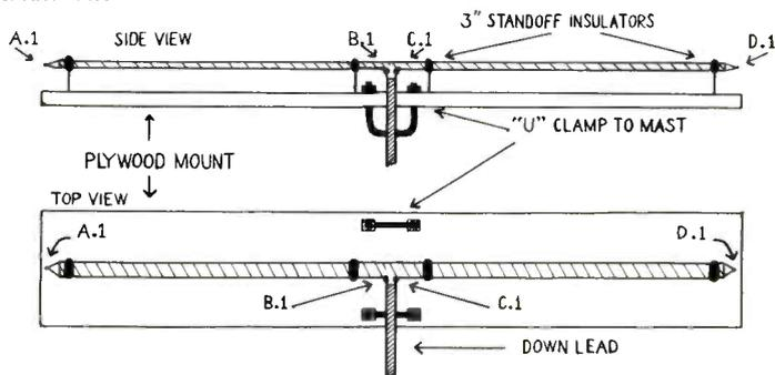
wires for each. If you can only build one Dipole, and are having trouble with more than one low band local, always cut the Dipole to the lowest channel you are experiencing trouble with.)
