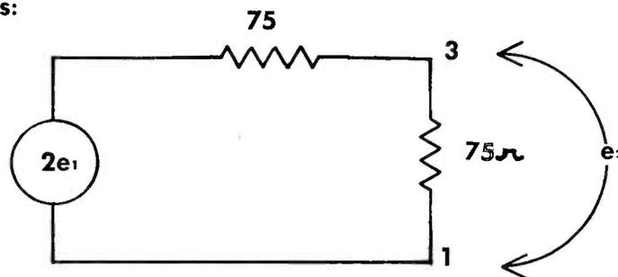
3 Therefore, in the four antenna array load voltage  $e_2 = \frac{2e_1 \times 75}{150} = e_1$
