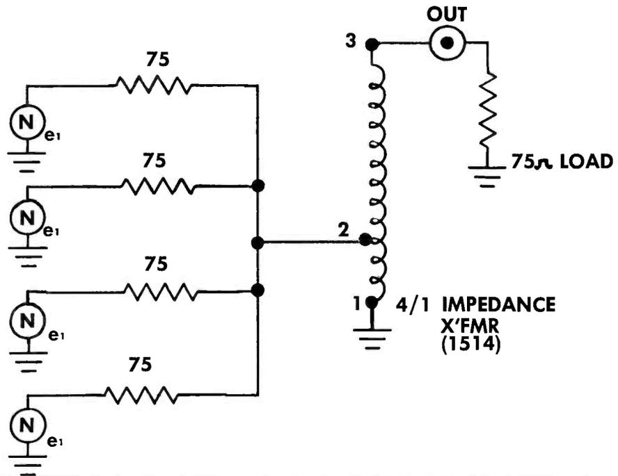
2 Using Thevenin's theorem the equivalent generator (antenna) voltage and impedance looking into terminals 1-3 appears as:
