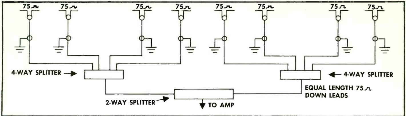
**FIGURE 3** EIGHT ELEMENT ARRAY (VERTICAL AND/OR HORIZONTAL STACKS)
