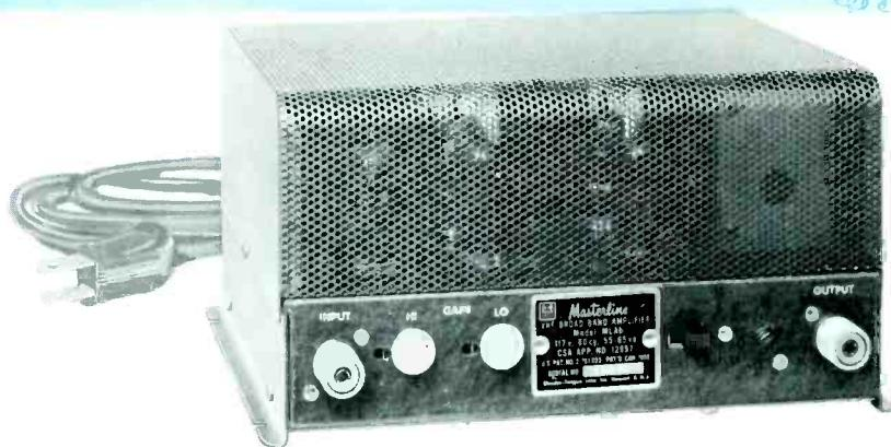
head-ends. In figure 3, the **MLA-b** is shown being used as a line extender. Up to 1700 feet of RG-11/U foam cable can be used between amplifiers (at channel 13). An **MAC** should be used every 3rd amplifier, to compensate for temperature changes, aging components, etc.
