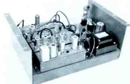
Unit must be ordered for specific channel. Operates from 115 vac, 60 cycles. 19 inch rack mounting. Output level, 60 dbm. **User net price: \$562.20 (channels 2-6); \$752.60 (channels 7-13).**
