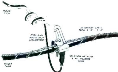
tective neoprene boot. Complete attenuation range from (highest) 41 db at channel 2 to lowest (7 db) at channel 13 available. Insertion loss varies from .04 db at channel 2 to 1.3 db at channel 13. **User net price: Model 900 (single), \$2.75 each complete. Model 901 (double) \$2.75 each complete.**
