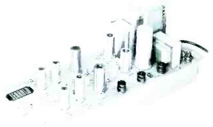
19-25 db gain, compensates for excessive losses in long cable runs; built in tilt control with automatic and manual gain controls. Cascadable, for industry use. **User net price \$219.50.**
