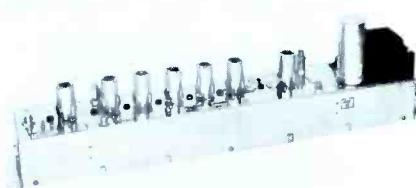
60 db. Indoor or outdoor (in housing) mounting. AGC. Unit can be cascaded for head end applications. **User net price: \$141.00.**
