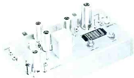
range 4-47 and 174-216 mcs. 15 db gain. Locates at bridging amplifier location in distribution systems. Converts signals in the 4-47 mcs. region to VHF channels 7-13 and then amplifies the converted signal to an appropriate distribution level. Plug in pads for cable equalization. **User net price: \$115.50.**
