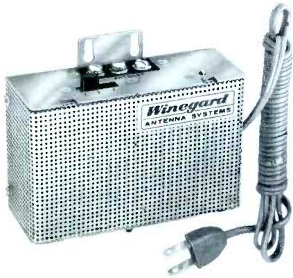
band. 300 ohm output, with 75 ohm tap. 3 position gain control. Drives up to six TV and/or FM receivers. Preamplifier application. **User net price: \$34.95.**
