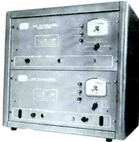
mounting. Operating voltages, 220 vac; 105-125 vac, 60 cycles. Input sensitivity for full output, 50 uV on 75 ohm line. AGC-30 db input variation produces less than 1 db output variation for signals in the 50 uV to 50,000 uV range. User net prices on request as customer requirements vary.
