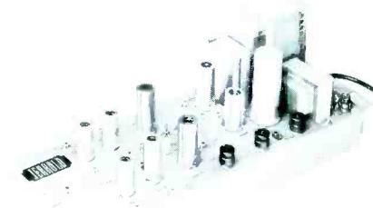
19-25 db gain, compensates for excessive losses in long cable runs; built in tilt control with automatic and manual gain controls. Cascadable, for industry use. **User net price \$219.50.**
