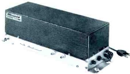
Unit has seven tubes, including two 6DJ8 type in cascade input stage. High and low band gain, 45 db. For use in driving up to 150 TV-FM receivers. Low band output, 1 volt. High band output, 1 volt. **User net price: \$154.95.**
