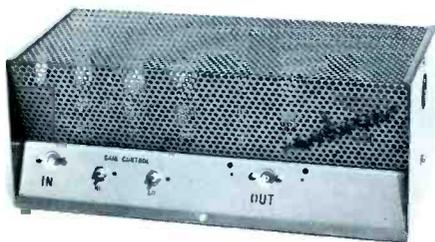
108 mcs., 174-216 mcs. 38 db gain, both high and low bands. Separate gain controls. Unit operates from 115 vac, 60 cycles. **User net price: \$113.40.**
