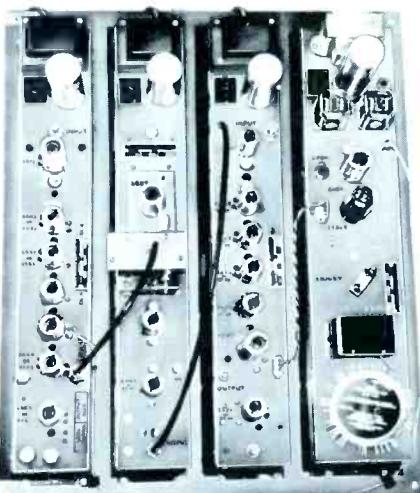
watt. Final transmitter tube is 6939 type. FCC type accepted. RC-1 remote control available. Operates 115 vac, 60 cycles. Automatic shut-off when originating station leaves air. Metal mounting base. **User net price: \$845.00.**
