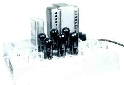
**JERROLD ELECTRONICS**—model AGC-213 Bandwidth 0.5 mcs. at — 3 db over 5-220 mcs. Used in connection with Jerrold model SCA-213. Has two inputs, 1 for xtal control carrier gen., 1 for video carrier control. Stabilizes and maintains signal levels throughout entire distribution system. **User net price: \$128.50.**
