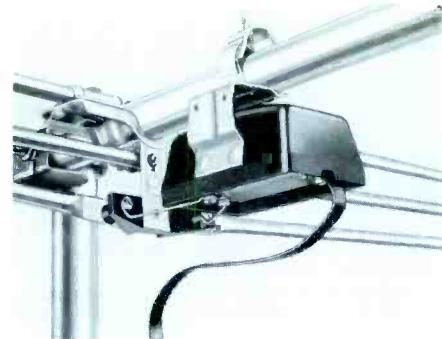
power is fed up to amplifier on feedline.
