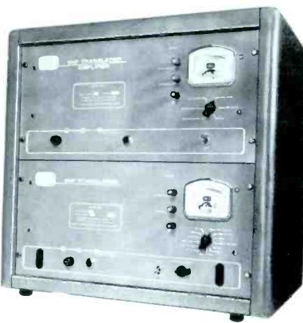
mounting. Operating voltages, 220 vac; 105-125 vac, 60 cycles. Input sensitivity for full output, 50 uV on 75 ohm line. AGC-30 db input variation produces less than 1 db output variation for signals in the 50 uV to 50,000 uV range. User net prices on request as customer requirements vary.
