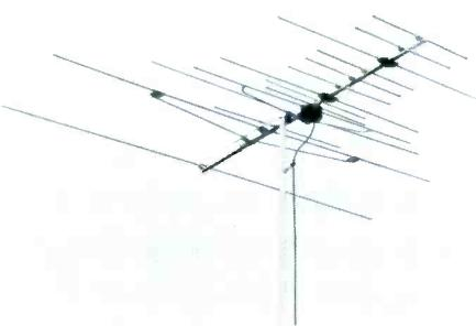
tion, 24 db. Feed impedance 300 ohms through Tapered T driven element. Amplifier and antenna integral unit. Antenna gold anodized. All transistorized models have 75 and 300 ohm outputs at antenna and 75/300 ohm input-output at remote power supply. 10,000 uV maximum signal, with three position gain switch. Tube types 300 ohm only, maximum signal input of 60,000 uV. **User net price: \$74.95.**
