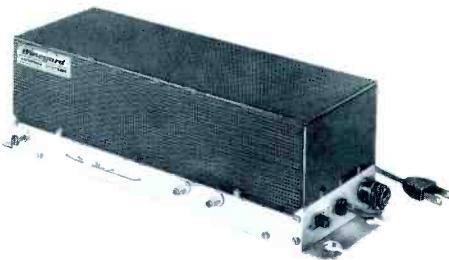
Unit has seven tubes, including two 6DJ8 type in cascode input stage. High and low band gain, 45 db. For use in driving up to 150 TV-FM receivers. Low band output, 1 volt. High band output, 1 volt. **User net price: \$154.95.**
