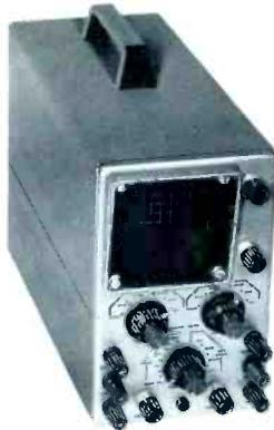
in four ranges. External capacity binding posts for lower sweep rates. Small, compact size measures only  $7\frac{1}{8}$  inches by  $4\frac{1}{8}$  inches by 11 inches. **User net price:** Kit, \$79.95.
