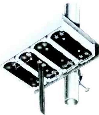
with broadband antenna; mixes or separates VHF and UHF signals; mixes or separates TV and FM signals; separates individual channels on broadband antenna. Allows up to 9 antennas to be grouped on single down lead. **User net price: \$3.57.**
