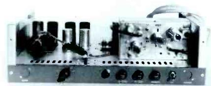
unit, employs two tubes for single conversion, 4 for double conversion. Gain varies from plus 2 db to minus 4 db for single-double conversions, low or high band. **User net price: \$145.00 per converter less power supply. 1 power supply will operate two converters.**
