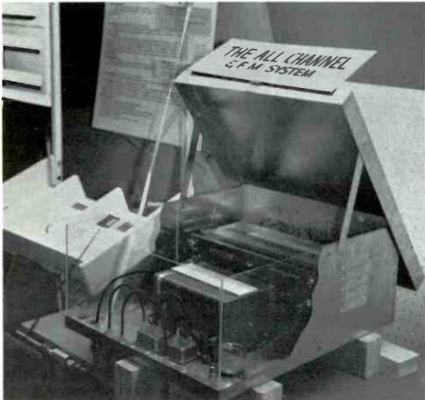
Telesystem Services Corporation of Glenside, Pa., displayed this chain distributed type all-channel trunk amplifier with separate external bridging ... feeding coscode type distributor amplifier.
