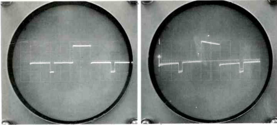
Figure 9. Oscilloscope presentation of square wave response in system with poor low-frequency response. Waveform at left is reasonably good (note tilt of sync pulse). Picture at right illustrates very bad low-frequency response. Streaking would be severe.
