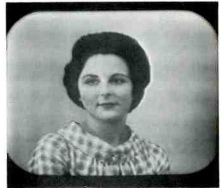
Figure 10. "Ringing" shows in picture as echoes displaced to the right of transitions between dark and light.
