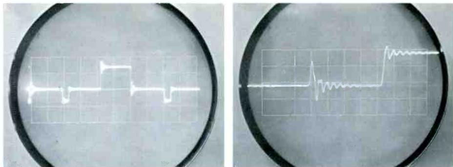
Figure 11. Same amount of ringing as in Figure 10 produces severe distortion of window signal (A) and sine-squared test pulse (B). Note severe oscillations at beginning and end of square wave. Sine-squared test is the more sensitive of the two, but is harder to evaluate qualitatively. Next month's article discusses this test in detail.
