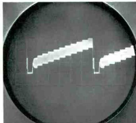
Figure 6. Stairstep test signal with superimposed 3.58-mc color subcarrier can be used to measure differential phase or gain. Differences in amplitude of modulation reveal differential gain. Differential phase measurements require synchronized phase detector.
