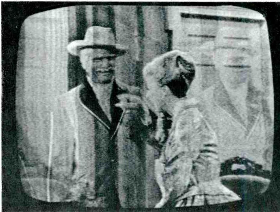
Figure 2. Poor frequency response or other irregularities lead to distortion of various sorts in the reproduced picture. Echoes usually result from non-linearities in baseband frequency characteristics, or from multipath transmission. Since transmission errors are rarely as bad as this exaggerated example, sensitive test methods are required to permit accurate evaluation of quality.
