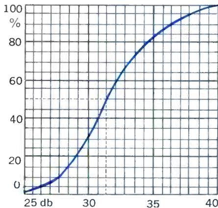
Minimum STRUCTURAL RETURN LOSS Distribution Curve
