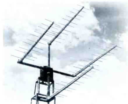
Because of the inherent broadband characteristics of these arrays, only three sizes are required to cover all VHF channels, the manufacturer reports. A single array can be used to receive all channels within its band provided their directions fall within the main lobe beamwidth. Single antenna elements are also available offering the same band, VSWR, and front-to-back ratio figures as the arrays.
