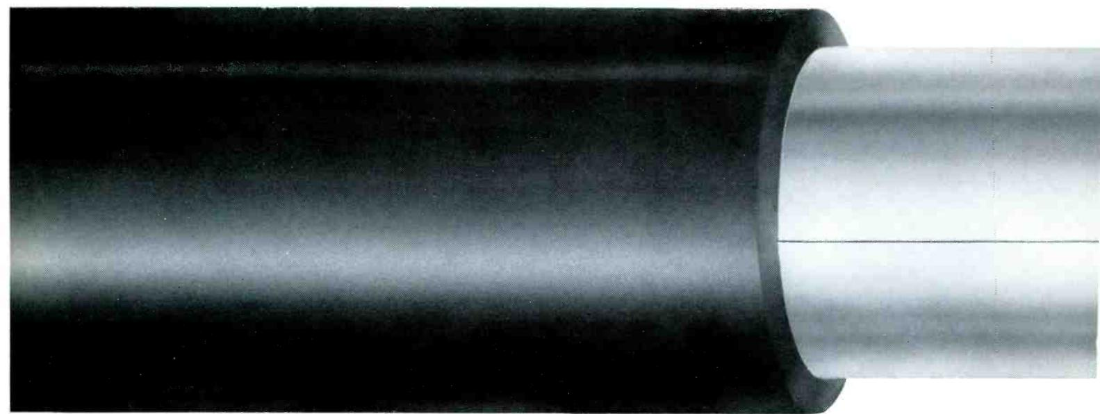
**Sealmetic's positive moisture barrier makes the big difference.** The Sealmetic sheath is hermetically sealed at the shield overlap, and is bonded between the entire outer conductor and the polyethylene jacket to form a unitized sheath. Moisture or humidity can't get between the shield and the jacket nor enter the core. The core stays dry and maintains the electrical characteristics of the cable.
