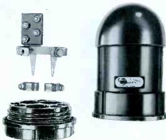
These terminals are the first to be specifically designed for direct burial under ground, or installation in a man-hole or vault, according to the manufacturer. Since unit is hermetically sealed, the entire housing maintains pressure, hence terminations do not need to be potted in epoxy, or dammed off and by-passed.
