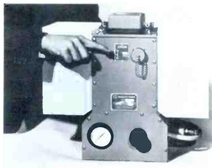
The small (22 to 125 pounds) automatic power plants produce low-cost, 24-hour-a-day electricity from the flameless combustion of commercial LP (propane) gas. The smallest (6 watt) generator uses \$23 worth of gas a year; the largest (50 watts), \$159 worth. They are designed for a wide range of commercial and industrial power uses.
