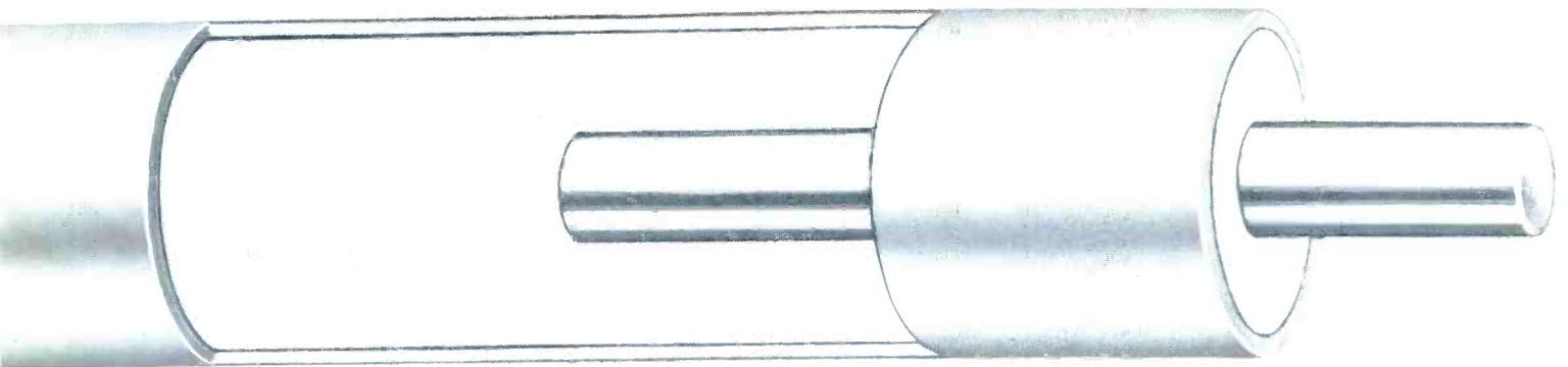
■ Now, the availability of 75 ohm Foamflex coaxial cable in four diameters — .412", 1/2", 3/4" and 1 5/8" — fills the needs of all-band CATV systems for rugged, high-performance cable in all required sizes. Foamflex, the original foam polyethylene dielectric cable, offers unequalled low loss for superior operation in community antenna and closed circuit television. Foamflex has a proven record in demanding applications in telemetry, missile guidance and microwave in addition to CATV.
