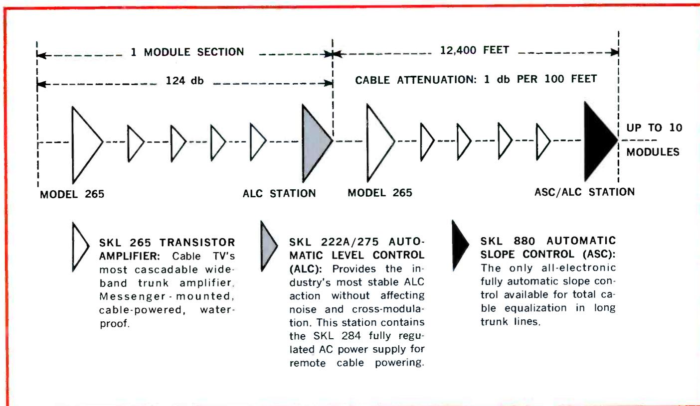
Each module section comprises five Model 265 Transistor Trunk Amplifiers cascaded in alternate sections with an ALC or ASC/ALC station. The module section length totals 124 db of cable. SKL's exclusive TEMPERATOR provides both thermal gain control and cable equalization at every Model 265 Amplifier. The
