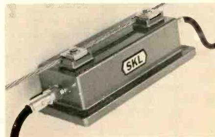
The nominal gain is 22 db at 216 mc, with a 7 db slope across the 54 to 216 mc band. Manual gain and tilt controls complete the compensation for the average cable losses encountered in feeder lines. Low noise and cross-modulation allow the Model 263 to be used even at the most remote ends of a distribution system.
