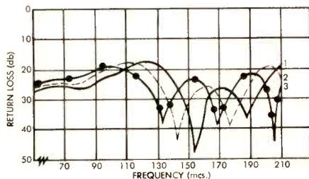
RETURN LOSS VS FREQUENCY FOR VARIOUS LENGTH JUMPER CABLES CONNECTED THROUGH HALFSTEP EQUALIZER (SKL 499) TO AMPLIFIER INPUT (SKL 222A) (1) 12" SOLID PE DIELECTRIC JUMPERCABLE (2) 18" SOLID PE CABLE, (3) 24" SOLID PE CABLE
