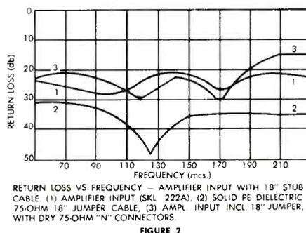
The combination of moist connectors and amplifier terminals can produce some startling effects. Figures 2 and 3 are drawn from data measured on actual jumper cable-amplifier combinations. The amplifier specifications indicate better than 20 db return loss, a fact which was substantiated by measurement. However, results as poor as 17 db (Figure 2) were obtained with jumper cable-connector combinations which measured 32 db minimum be-
