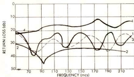
RETURN LOSS VS FREQUENCY — AMPLIFIER OUTPUT WITH 24" JUMPER CABLE. (1) AMPLIFIER OUTPUT (SKL 22A), (2) SOLID PE DIELECTRIC 75-OHM 24" JUMPER, (3) AMPL. OUTPUT INCL. 24" JUMPER, WITH DRY 75-OHM "N" CONNECTORS, (4) SAME AS (3), EXCEPT CONNECTOR MOISTENED WITH WATER
