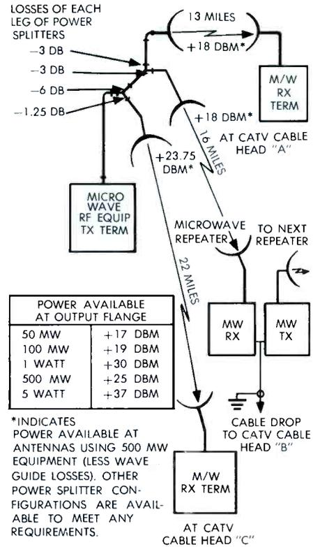
TYPICAL POWER SPLITTER ARRANGEMENTS FOR SIMPLEX ETV OR CATV APPLICATIONS
