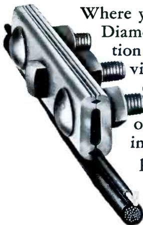
Where you're running Figure 8 distribution wire, Diamond Support Clamps with their positive action and unique metal to metal contact provide the greatest gripping strength! The clamping jaws have grooves for .109" messenger on one side, .134" on the other, plainly marked to insure proper installation. Two types are available—pole mounted and cross-arm mounted, as shown. For further information, contact:
