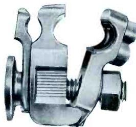
Tele-Tap "A" for .412 cable. A solid aluminum block that will not cause electrolytic action on aluminum cable. Uses stainless steel pins and insert. An inbuilt rubber gasket gives perfect water-proofing.
