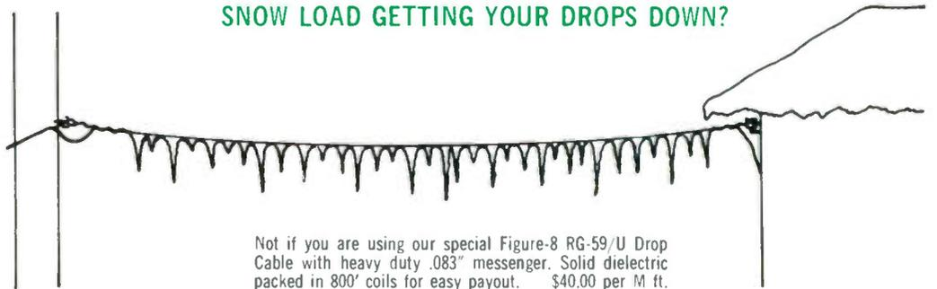
Not if you are using our special Figure-8 RG-59/U Drop Cable with heavy duty .083" messenger. Solid dielectric packed in 800' coils for easy payout. \$40.00 per M ft.
