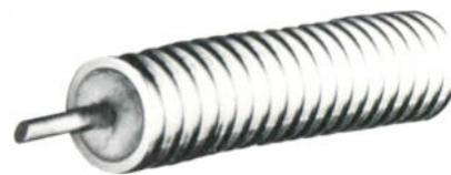
pression tests are said to prove it to be 30 percent stronger than non-corrugated solid-jacketed cable because the impact stress is spread evenly over a wider area instead of causing a sharp bend or kink.
