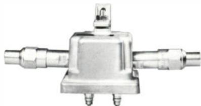
against RFI leakage is provided by the unit's die-cast housing. It is also protected by moisture resistant strip-line construction. According to the manufacturer the tap has a tilt design for each of eight values from 6db to 34db, insertion loss is said to be less than 0.3db for the 18db model. The unit can be used with both .412 and .500 cable with pedestal mounting available. Cost of the standard .412 model is \$7.90. Outlet plates range in cost from \$1.58 to \$5.80.
