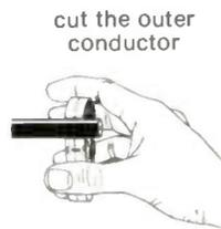
cut the outer conductor
