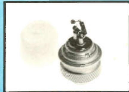
Just like regular Cascade Trunk Amplifiers, this new Line Amp has Temperature Level Control (TLC). The Thermistor Probe monitors the weather, and relays temperature information to an interstage varicap diode which increases or decreases gain to compensate for changes in cable attenuation. Result: constant levels, happier subscribers and fewer trips up the pole!
