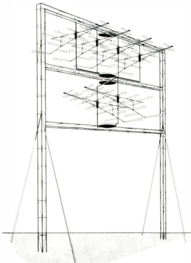
*H-frame mounted Expo antennas are said to provide optimum reception. Two antennas can be tower-mounted, as well.*
