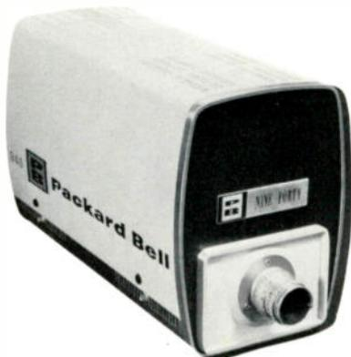
els offerings either 525 or 875 scan lines. It can also be operated crystal-controlled random interlace at 525, 625, 675, 735 and 875 scan rates or driven with an external EIA sync generator for full EIA compliance.
