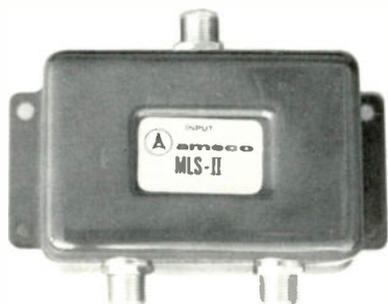
maximum insertion loss with typical insertion loss of 3.75 dB, and an input return loss of 16 dB. The device accepts F-59 connectors and is available for immediate delivery. Price of the MLS-II is \$2.50.
