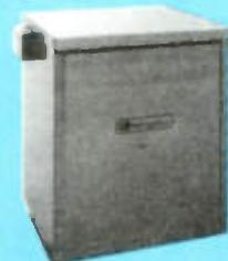
Weatherproof power supply housing of welded sheet aluminum. Supplied complete with externally-operated primary switch/circuit breaker, internal duplex receptacle and crossarm mounting bracket. 14 1/2 x 13 1/4 x 11 1/4 ins. 11 lbs.
