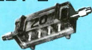
Available in tap values from 12 to 36db, the CEDT provides four output taps with high directivity and isolation. The waterproof housing is of corrosion-resistant aluminum alloy.
