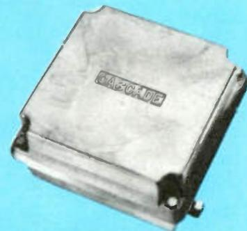
Weatherproof power supply housing of cast aluminum alloy for pole, cross-arm or underground installation. Clamshell design and silicon rubber sealing gasket provide complete sealing and radiation protection. Includes primary switch/breaker and AC convenience outlet. 12 x 12 x 7 3/4 inches. 17.5 lbs.
