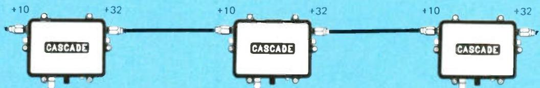
Now, run the thermometer up to 120° F (in the sun). The thermistor probe on each amplifier will sense the change and turn up the gain. Levels will now look something like this:
