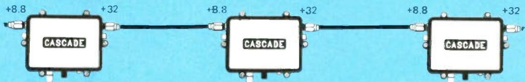
*Or, swing the temperature to twenty below, and watch the thermistors drop the gain to avoid cross mod. Again, outputs are at +32.*
