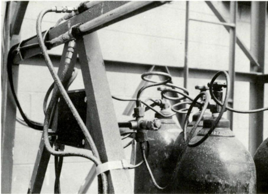
A typical hook-up using bottled, dry nitrogen to pressurize a system.
