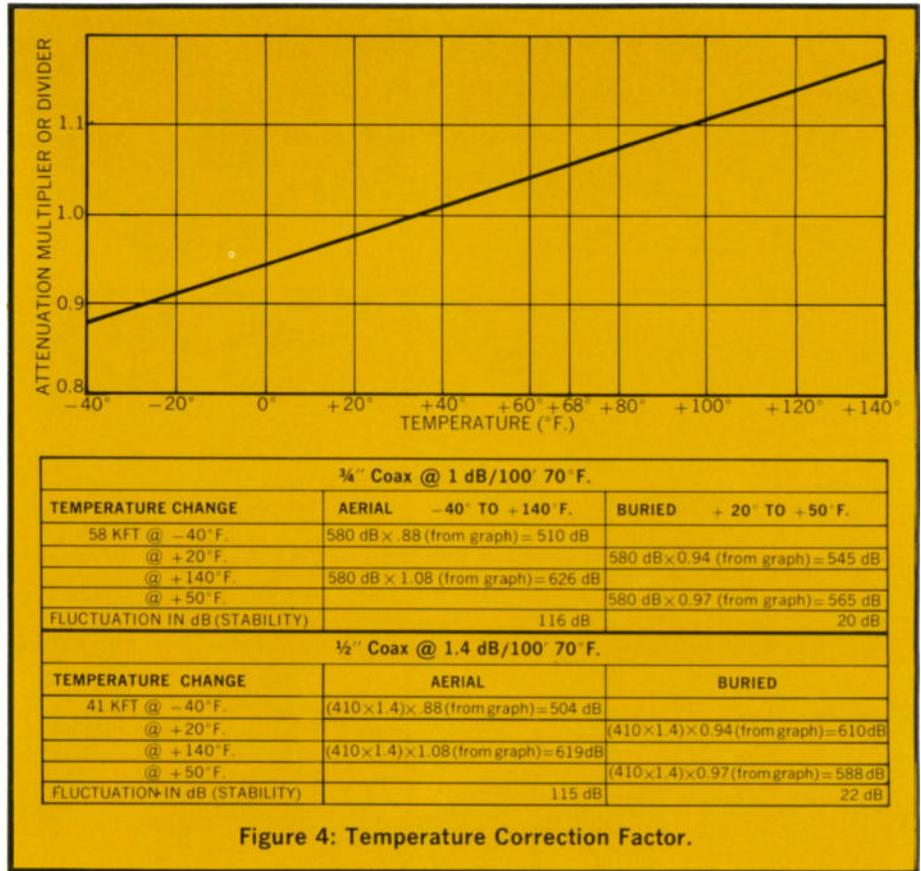
Figure 4: Temperature Correction Factor.
