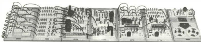
Davco's "Functional Design" head-end packages are completely assembled and checked out at the Batesville plant. Above is a 12-channel signal processing system which also provides for two taped-music and two FM channels.
