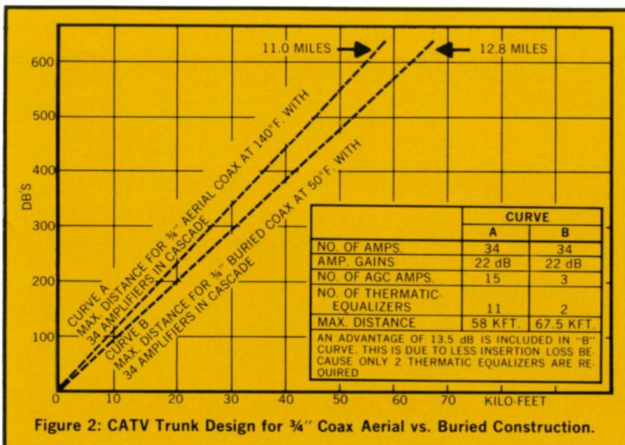
Figure 2: CATV Trunk Design for  $\frac{3}{4}$ " Coax Aerial vs. Buried Construction.
