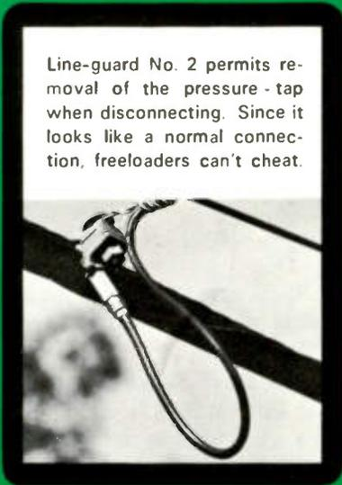
Line-guard No. 2 permits removal of the pressure-tap when disconnecting. Since it looks like a normal connection, freeloaders can't cheat.
