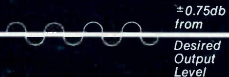
4. Long time constant of AGC circuit does not respond to short term signal variations, reacting only to cable attenuation changes caused by temperature.
