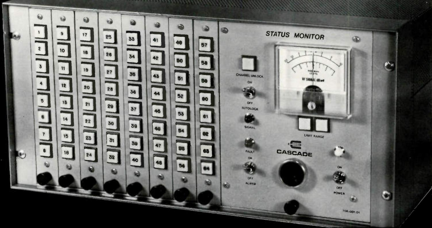
Cascade's two-way facilities allow status monitoring, signals and locally originated programmes to pass simultaneously along the CATV cable in opposite direction to the VHF band signals from the head end.
