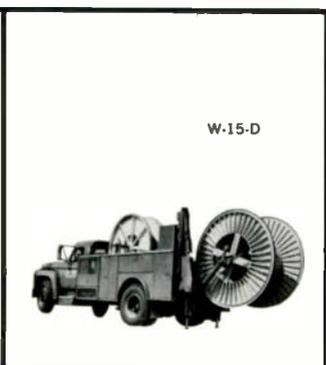
Servi-Loader loads and handles reels 84" dia. x 46" wide. Servi-Drive delivers pull on drum to 15,000 lbs.
