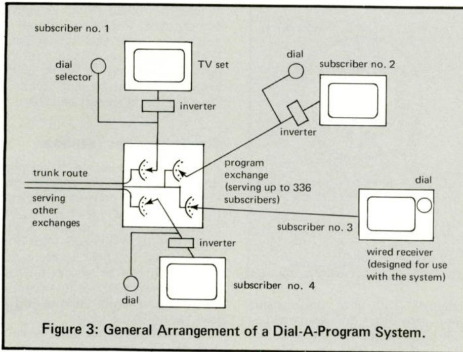
Figure 3: General Arrangement of a Dial-A-Program System.
