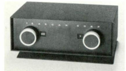
Packaged in a cabinet of modern design, these attenuators feature low VSWR and flat frequency response. Calibration data is supplied with these instruments to increase their usefulness. Calibrated attenuation data is supplied at 30 MHz, 500 MHz, 1000 MHz and 1500 MHz. These attenuators are useable to above 2000 MHz, with slight degradation in the performance specified at 1500 MHz.
