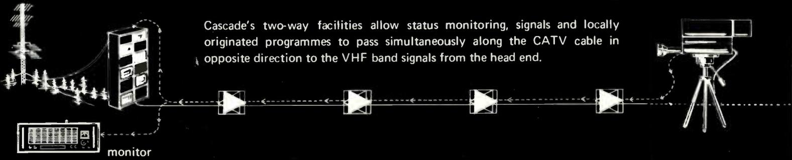
The output level of individual trunk amplifiers may be monitored constantly, day and night, at the head end or at any control point along a trunk line.
