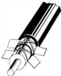
The Lamiglas Tape Design Center at Facile has perfected 3-ply shielding tapes constructed of foils, laminated to both sides of insulating films.
