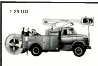
29' telescope model specially designed for self-supporting and CATV. Handles strand-wire medium cable.
