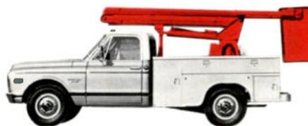
Provides a working height of 29' mounted on a ¾ ton chassis. Auxiliary engine generator supplies hydraulic power and 2500 w of 110v in the bucket. Hundreds in use world wide.
