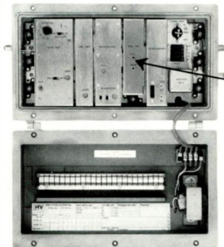
Sub VHF amplifier or Jumper Module. (Separation filters under base plate.)
