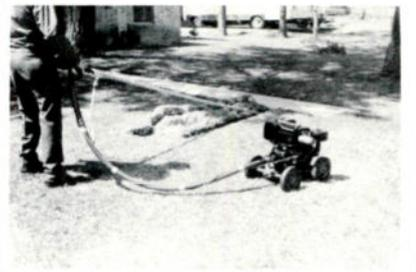
Using our swivel unit and special water bit will enable you to drill under driveways. The drill stem is standard 3/4" water pipe.
