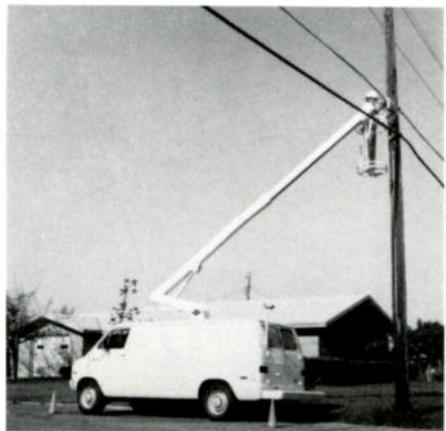
offers a working height of 30 feet, full 360° rotation and an elevation range of -6° to +84°. Rated bucket capacity is 300 pounds, and the VAN-TEL meets all OSHA standards without ballast, outriggers or stabilizers, even
