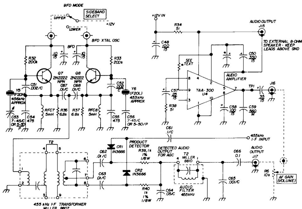
fig. 5. Bfo, product detector and audio amplifier circuits.
