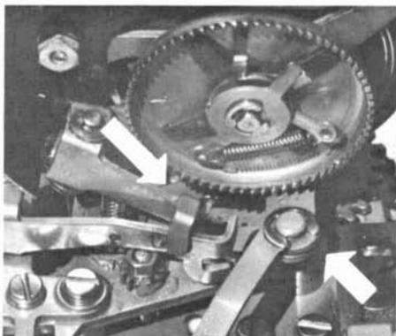
fig. 7. The bottom side showing the retaining ring (right) that is removed to take off the ribbon holder and (left) the manner in which the ratchet levers are unhooked.
