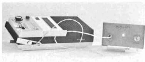
Complete memo-key with cassette recorder. System is compact and offers easy storage of data for the active operator.
