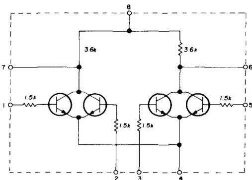
fig. 12. HEP580 MRTL dual-input NOR gate.
