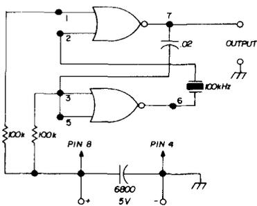
fig. 13. 100-kHz crystal oscillator using the HEP580.
