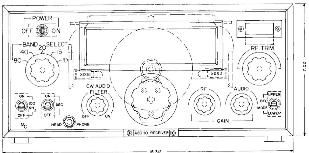
fig. 10. The complete parts layout for the A80-10 is shown on the facing page, the printed-circuit layout is shown in fig. 13 and the construction and panel layout of the receiver is shown above.
