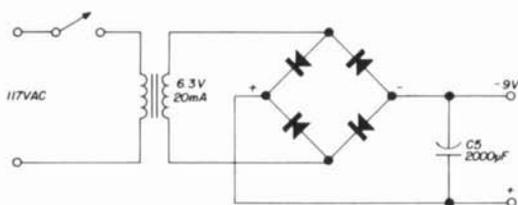
fig. 4. Suggested power supply circuit.
