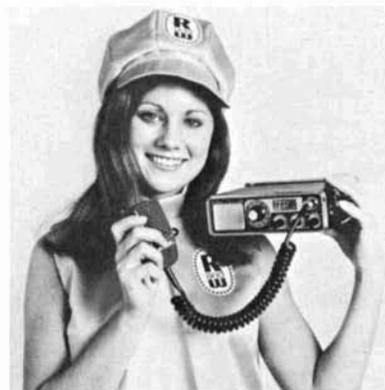
SAROC featured the introduction of Ross and White's new two-meter fm transceiver with built-in tone-burst encoder. The new RW-Bnd transceiver offers twelve-channel operation (four crystals supplied), three power levels of 0.1, 1 and 10 watts, all solid-state design, and the three-tone encoder. The tones are factory set for the three most common tone-burst frequencies, but they are easily changed in the field.
