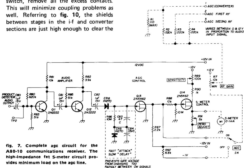
fig. 7. Complete agc circuit for the A80-10 communications receiver. The high-impedance fet S-meter circuit provides minimum load on the agc line.
