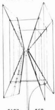
A two element fibre glass quad antenna designed for better signal discrimination & directivity on 10, 15 & 20 meters!
