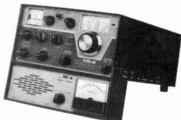
Adding an MC-4 Mobile Console, with its excellent wattmeter and built-in speaker, is the only way to improve a Drake TR-4.
