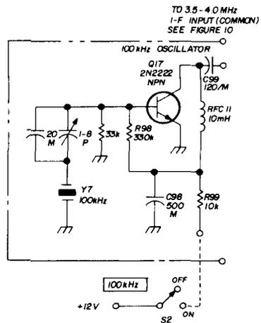
fig. 9. Circuit for the 100-kHz marker oscillator.
