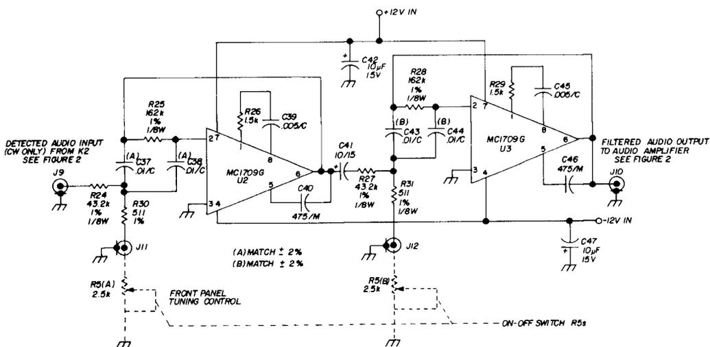
fig. 4. Audio filter provides excellent selectivity for CW communications.
