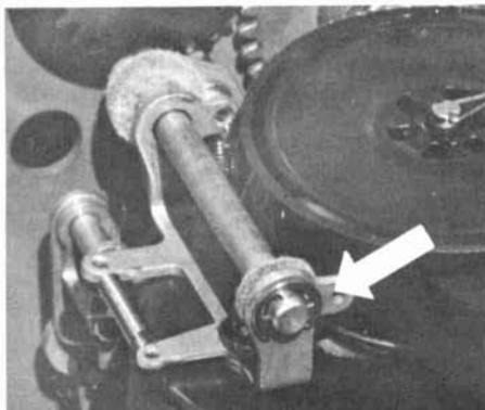
fig. 8. The retaining ring at the rear of the left spool is also removed to take off the ribbon holder.
