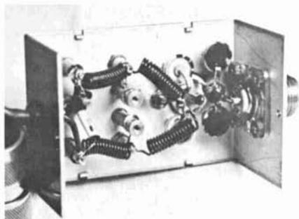
Interior view of the rf head. Readily visible are the various components and their placement within the minibox. The three 150-ohm resistors must be placed to ensure shortest possible leads. Low-loss ceramic socket for the 5722 keeps losses low at higher vhf ranges.
