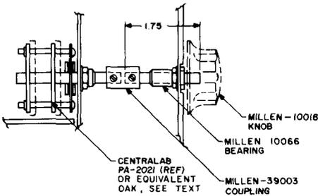
fig. 11. Construction details of the band-selection switch.
