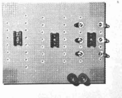
W3FQJ's breadboard for IC experiments uses IC sockets and solderless binding posts for quick circuit changes while still protecting the delicate IC wire leads.
