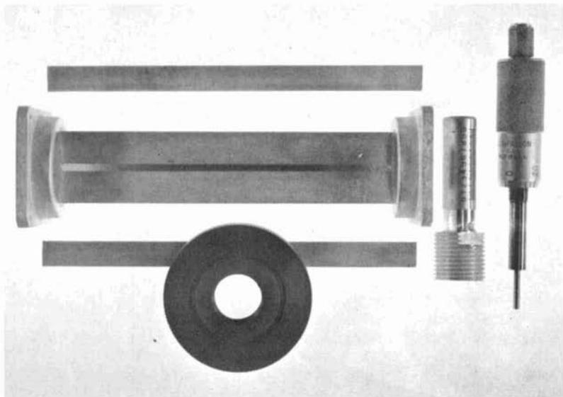
fig. 4. The homemade slide screw tuner. The tuning mechanism is a Sears micrometer body. In this version the threaded cylinder which holds the micrometer is  $\frac{3}{4}$ -inch OD instead of the specified 1 inch. The 1-inch piece is better electrically as it presents a larger surface area upon which to slide. It is included in fig. 5.
