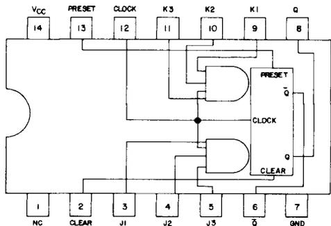
**fig. 3. Universal flip-flop (A) and the actual pin connections of the 7472N (B).**
