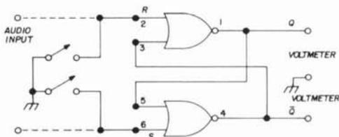
fig. 10. NOR gates arranged into a flip-flop.
