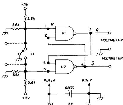
**fig. 7.** NAND gates in flip-flop. U1 and U2 are each  $\frac{1}{4}$  of an SN7400N. Dashed lines show connections for an audio input.
