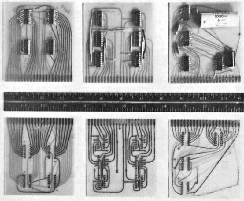
Front and back views of the three circuit boards. On the left, the buffer/driver board; in the center a typical board with two switching modules; on the right the control module.
