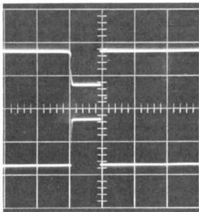
fig. 4. Oscillograph of the 15 Hz scanning pulse.
