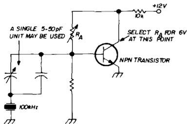
fig. 18. When initially adjusting the bfo or 100-kHz oscillators using other than the recommended transistors, it may be necessary to select the base-to-collector resistor  $R_A$  to compensate for variations in transistor gain and crystal impedance. Adjust  $R_A$  for 6 volts at the collector of the transistor.
