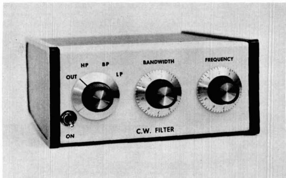
Tunable audio filter built by WIDTY is housed in Ten-Tec JW-5 enclosure. Input and output jacks are on rear panel.
