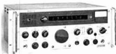
The Racal RA6700 is a fully synthesized, tunable, solid-state communications receiver designed for all modes of reception over the frequency range of 15 kHz to 30 MHz. The internal synthesizer provides single-knob frequency control that allows rapid tuning across the complete frequency range with the feel and smoothness of a VFO, while retaining the accuracy and stability of the in-
