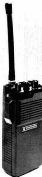
A compact new 1-watt, 2-meter handheld amateur fm transceiver is now available from Standard Communications Corp. of Carson, California. This transceiver, designated C-118, is approximately the height and width of a dollar bill, and permits the user to transmit up 600 kHz, down 600 kHz, or receive and transmit on the same frequency with just one crystal. This provides 18-channel capability with only six crystals.
