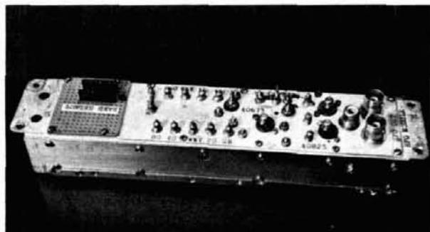
**High-frequency oscillator module.** The band-select signals are connected through the DIP socket.
