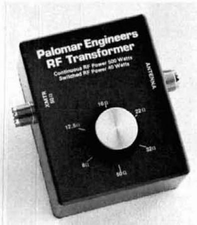
Palomar Engineers has a new broadband rf transformer. It matches vertical and mobile antennas to 50-ohm coaxial cable. Impedance values of 8, 12.5, 16, 22, 32, and 50 ohms can be selected by a convenient switch.
