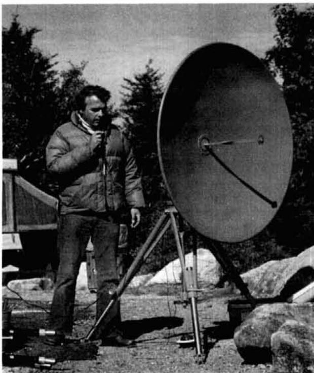
10-GHz Gunnplexer system setup by the W1FC group on Pack Monadnock in New Hampshire during the September vhf/uhf contest. Two-way communications were established with Gunnplexer-equipped stations in Maine, New Hampshire, and Vermont.
