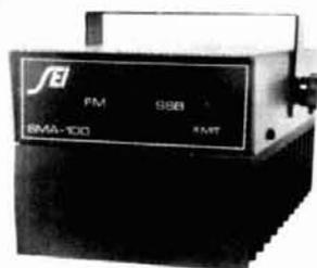
**SMA-100** 2m Mobile Linear Amplifier. 13.6VDC. Solid State, Strip Line construction. FM or SSB. 5-15w input, 75-80w output. 25 watts maximum drive FM, 20w PEP SSB. 100% Duty cycle. VSWR protected. No tuning. LED indicator. 4" w x 9" d.
