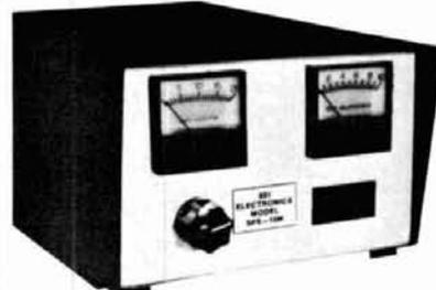
Power supplies designed for precise regulation. IC regulator. Automatic current limiting, overvoltage and short protection. 115VAC input/13.6VDC output. Metered models are variable 3-14VDC. Available with 10, 20, or 30 AMP CONTINUOUS rating.
