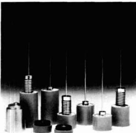
A completely new line of mobile antennas has been introduced by Signals Communications Corporation. The new line covers 30 through 512 MHz. These high-performance, low-profile antennas feature plated whips, high-impact bases, and optional springs. These antennas will fill the needs of most professional and government applications. The Matchmate mobile-mount adapter system permits the mounting of Signals antennas on all popular mounts.
