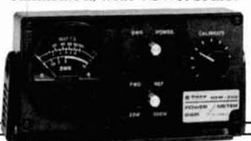
**SWR BRIDGE SWR 1A** with dual reading meters. 1000 watts RF. 3.5-150 MHz. Reads relative power output.
