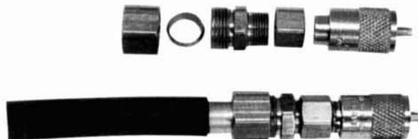
Above, component and assembled view of hardline connector. Smaller compression ring, not shown, is not used. At right, result of trimming shield with tubing cutter. Original ID of 11.43 mm (0.450 inch) was reduced to 8.39 mm (0.330 inch) at right.
