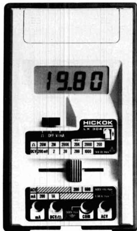
Hickok Electrical Instrument Co. has introduced the LX304, the latest model in their LX series of hand-held DVOM's. Like the LX303, the LX304 features an easy-to-read, 1/2-inch high, 3 1/2 digit LCD display; automatic polarity, zero and over-range indica-
