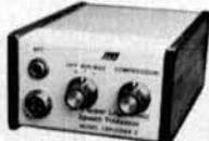
**MFJ-525 RF Speech Processor** gives you up to 4 times more average SSB power on all bands. Powerful, natural sounding speech punches through QRM and DX piles up. A true RF processor, the 525 works with any rig, any mic. No internal connections needed. **Two color VU meter** aids in setting clipping. **Full controls:** clipping level, output level, On-Off/Bypass switch, LED indicator. Shielded cable with PTT line, 4-pin mic. jack & plug, RFI protected. 12-18 VDC
