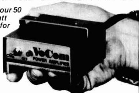
Give your low-power 2-meter rig real punch by delivering a potent 25-watt signal with only two watts of drive (also available set up for 200 milli-watts drive). Compact and convenient to mount VoCom's Model 2C025 is ideal for car, boat, or anywhere you've got a 12 VDC source. At only \$84.95 (\$99.95 for 200 mW drive), it's the perfect companion for your Drake, Encomm, Henry, Icom, Kenwood, Motorola, Standard, Wilson, Yaesu or other 2-meter FM portable!
