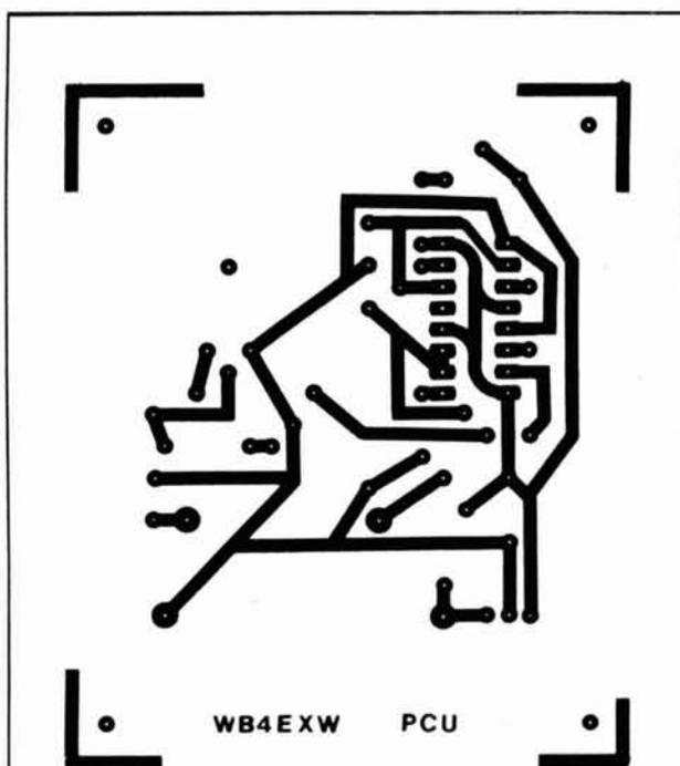
fig. 3. Full-size printed wiring board layout for the pulse-control unit. Wire side is shown.
