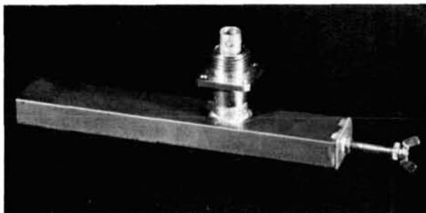
Tunable waveguide diode mount with TWT or BWO N connector.
