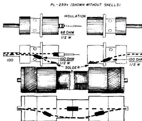
fig. 4. A 10-dB attenuator, again made from coax connectors. Three resistors form a pi network.
