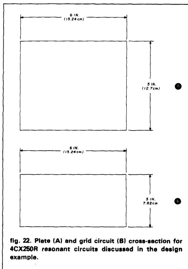
fig. 22. Plate (A) and grid circuit (B) cross-section for 4CX250R resonant circuits discussed in the design example.
