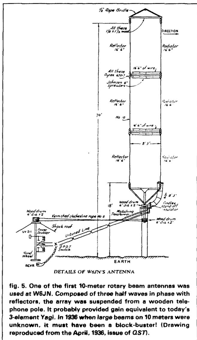
fig. 5. One of the first 10-meter rotary beam antennas was used at W6JN. Composed of three half waves in phase with reflectors, the array was suspended from a wooden telephone pole. It probably provided gain equivalent to today's 3-element Yagi. In 1936 when large beams on 10 meters were unknown, it must have been a block-buster! (Drawing reproduced from the April, 1936, issue of QST).
