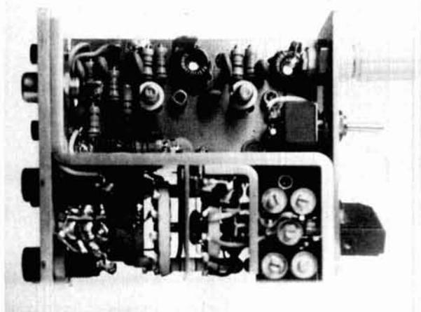
Converter top view. The input toroid is on the printed circuit at upper right, followed by the rf transistor, mixer toroid, and mixer transistor to the left. Oscillator transistor is at the lower left-hand corner of the printed circuit. The central aluminum strip acts as converter chassis and shield. Below it at the right are the trimmers, followed by the two-wafer bandswitch, with shielding between them. The adjustment capacitors are at lower left, as are the power input/output jacks.
