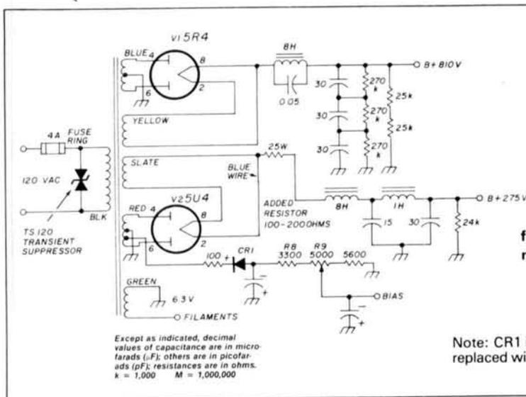
fig. 3. Circuit diagram of 516F-2 power supply with modifications.
