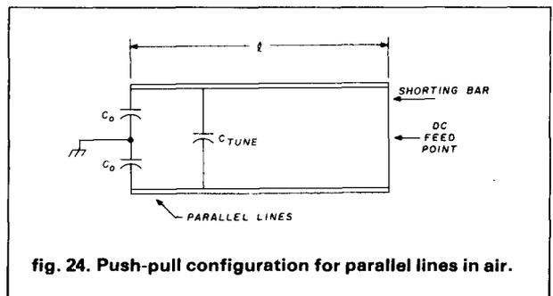
**fig. 24.** Push-pull configuration for parallel lines in air.
