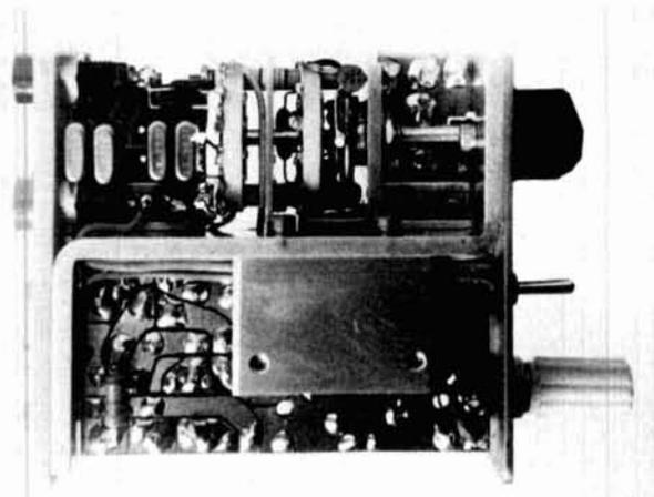
Converter bottom view. At upper right is the printed circuit supporting the rf trimmers, followed by the bandswitch and, at the left, the crystals (the 13-MHz crystal is missing). Below the central aluminum element is the lower part of the main printed circuit together with its supporting bracket.
