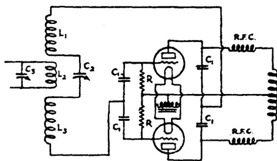
fig. 2. The nu8EX transmitter used for the first two-way 10-meter contact had a pair of 210 tubes in a self-rectified oscillator circuit. Alternating current at line frequency was applied to the plates of the tubes from the transformer at the right of the circuit (secondary only shown). With the low-C tank circuit and ac plate supply, the transmitter note must have been terrible! But it was good enough to do the job. (Drawing reproduced from the August, 1928, issue of *QST*).
