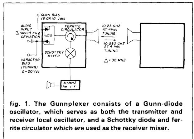
fig. 1. The Gunnplexer consists of a Gunn-diode oscillator, which serves as both the transmitter and receiver local oscillator, and a Schottky diode and ferrite circulator which are used as the receiver mixer.
