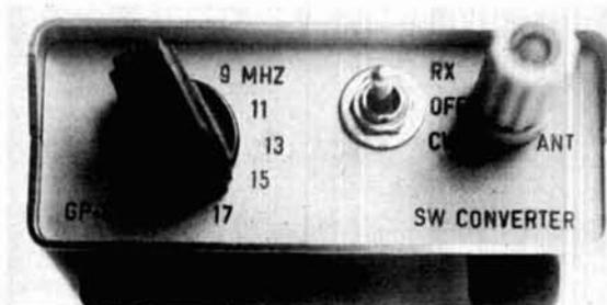
Converter front view. The power switch is a two-pole, three-position affair that switches the converter off and leaves the receiver operating as an independent unit. The converter weighs about 12 ounces (340 grams); current drain is 10 mA at 12 Vdc.
