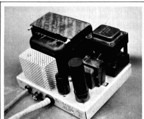
The Collins 516F-2 power supply after modification. The silicon replacement rectifiers substitute for the rectifier tubes.
