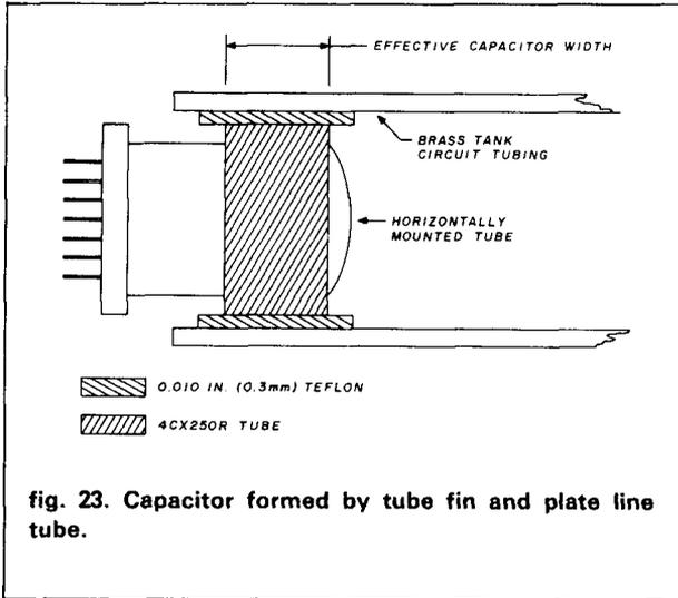
**fig. 23.** Capacitor formed by tube fin and plate line tube.
