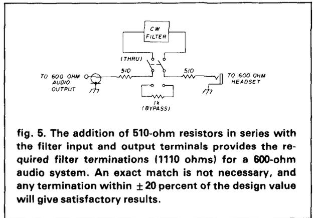
fig. 5. The addition of 510-ohm resistors in series with the filter input and output terminals provides the required filter terminations (1110 ohms) for a 600-ohm audio system. An exact match is not necessary, and any termination within  $\pm 20$  percent of the design value will give satisfactory results.
