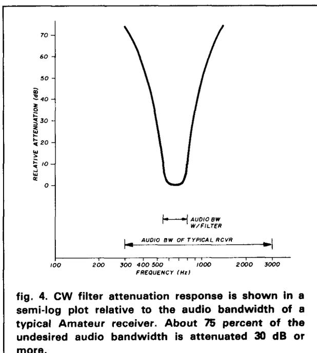
fig. 4. CW filter attenuation response is shown in a semi-log plot relative to the audio bandwidth of a typical Amateur receiver. About 75 percent of the undesired audio bandwidth is attenuated 30 dB or more.
