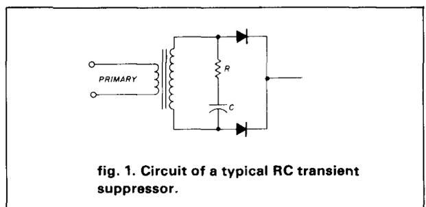
**fig. 1. Circuit of a typical RC transient suppressor.**
