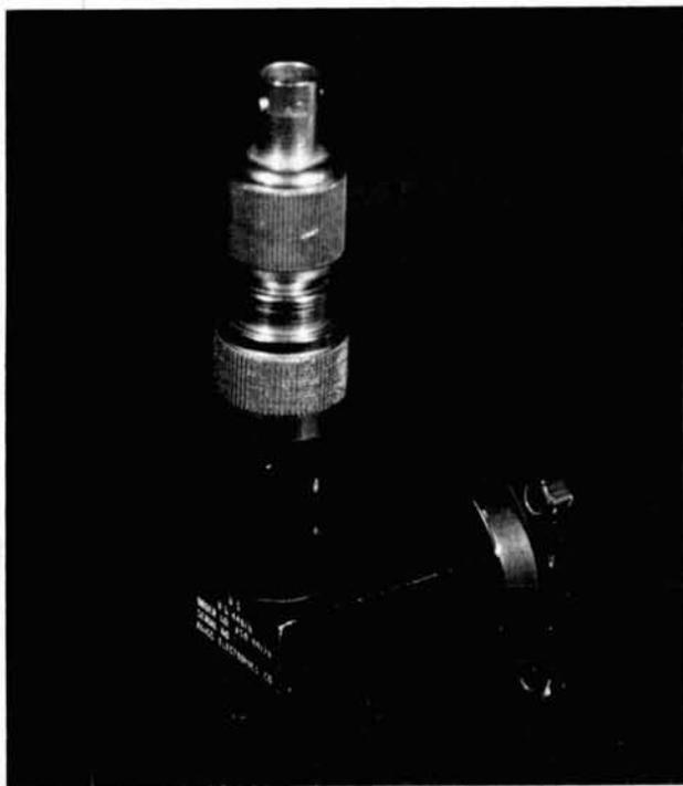
PRD 613M coaxial mount with waveguide-to-N adapter.
