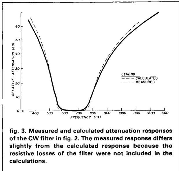
fig. 3. Measured and calculated attenuation responses of the CW filter in fig. 2. The measured response differs slightly from the calculated response because the resistive losses of the filter were not included in the calculations.
