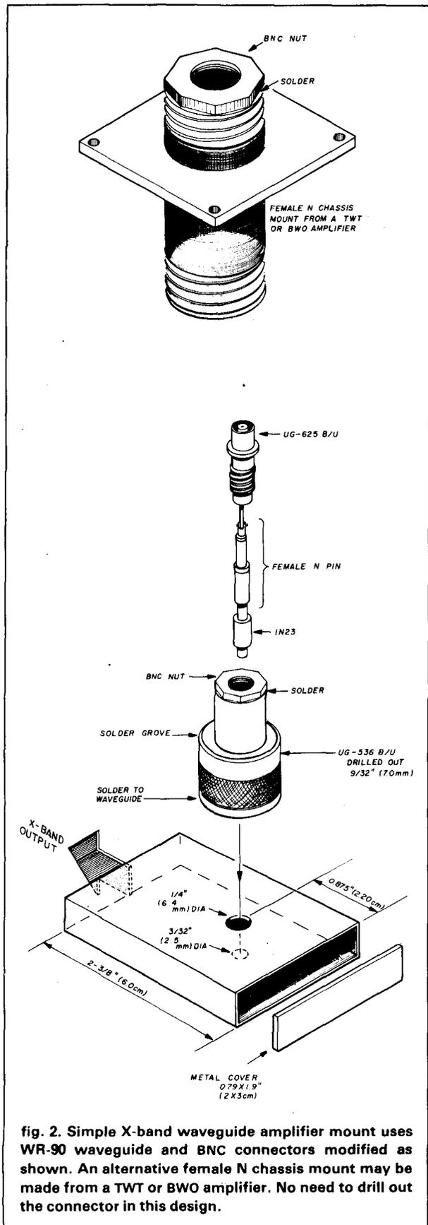
fig. 2. Simple X-band waveguide amplifier mount uses WR-90 waveguide and BNC connectors modified as shown. An alternative female N chassis mount may be made from a TWT or BWO amplifier. No need to drill out the connector in this design.
