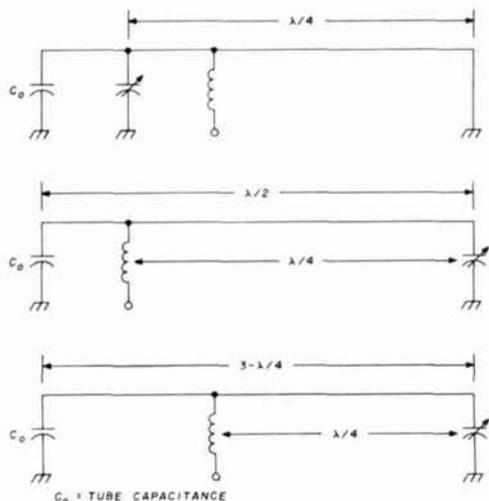
fig. 26. Line feed configuration for multiple  $\lambda/4$  segments.
