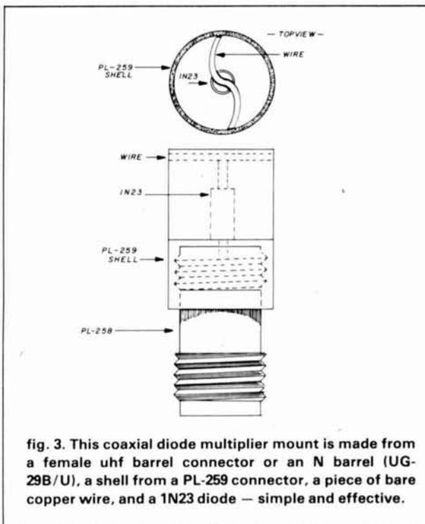
fig. 3. This coaxial diode multiplier mount is made from a female uhf barrel connector or an N barrel (UG-29B/U), a shell from a PL-259 connector, a piece of bare copper wire, and a 1N23 diode — simple and effective.
