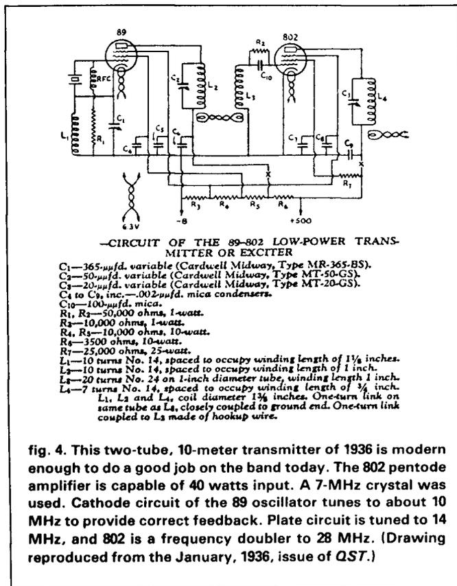
fig. 4. This two-tube, 10-meter transmitter of 1936 is modern enough to do a good job on the band today. The 802 pentode amplifier is capable of 40 watts input. A 7-MHz crystal was used. Cathode circuit of the 89 oscillator tunes to about 10 MHz to provide correct feedback. Plate circuit is tuned to 14 MHz, and 802 is a frequency doubler to 28 MHz. (Drawing reproduced from the January, 1936, issue of QST.)
