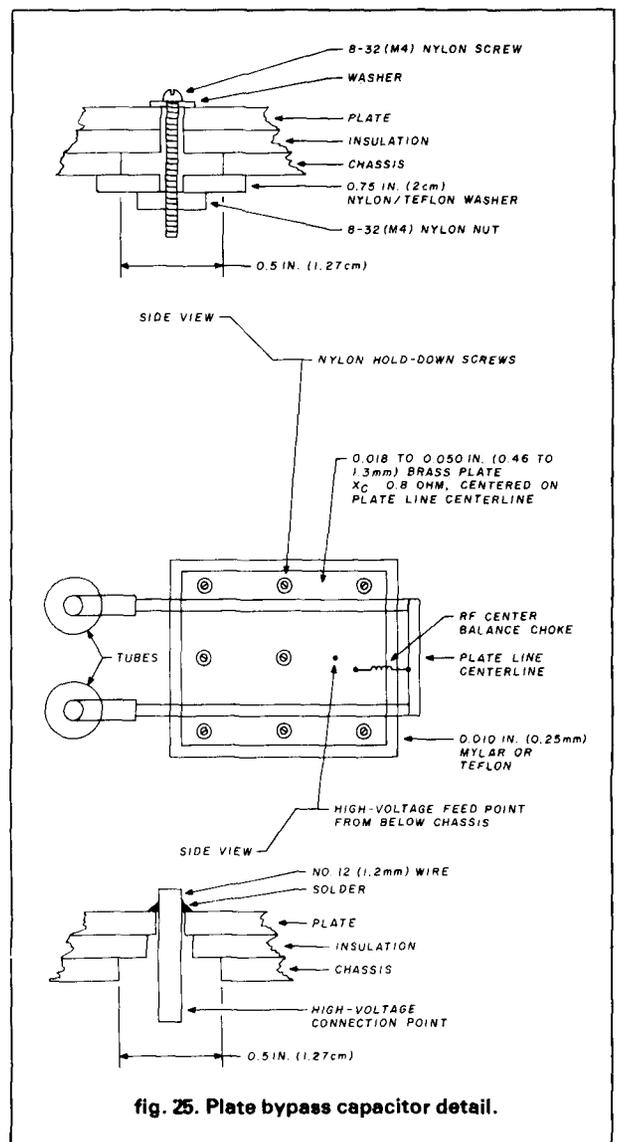
fig. 25. Plate bypass capacitor detail.
