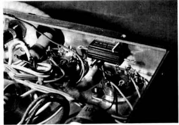
Close-up of underside showing the rectifier sockets and the new 25-watt resistor mounted on the rear apron.
