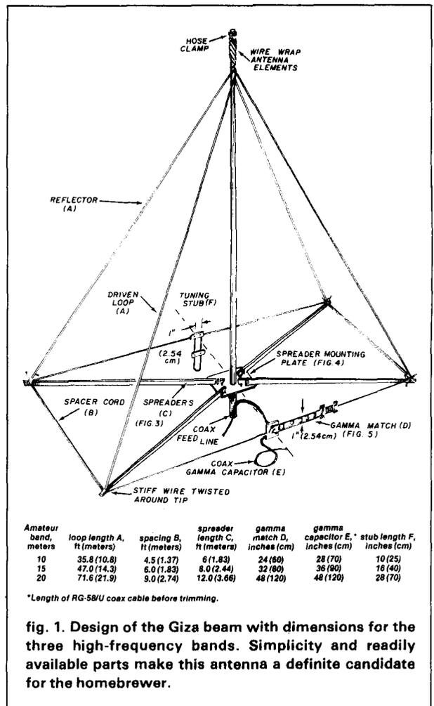
fig. 1. Design of the Giza beam with dimensions for the three high-frequency bands. Simplicity and readily available parts make this antenna a definite candidate for the homebrewer.
