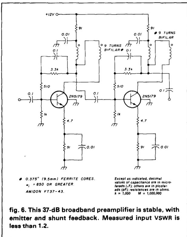
fig. 6. This 37-dB broadband preamplifier is stable, with emitter and shunt feedback. Measured input VSWR is less than 1.2.
