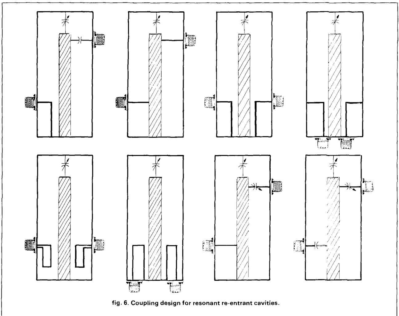
pickup loops are usually used. In some cases, direct connection to low-impedance positions on the inner conductor is used, especially where cavities are connected in cascade. Capacitive probes provide a convenient method of feeding energy to or from high-impedance circuits. Some coupling configurations are shown in fig. 6.
