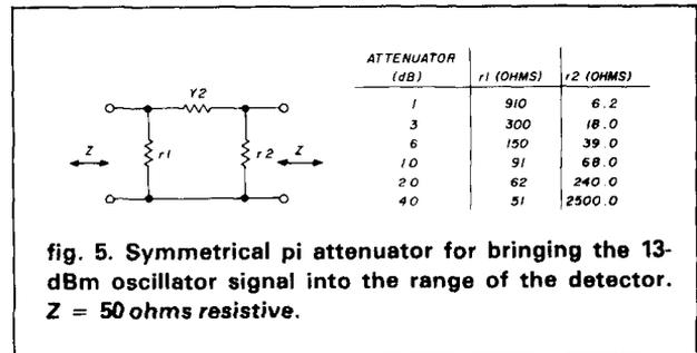
fig. 5. Symmetrical pi attenuator for bringing the 13-dBm oscillator signal into the range of the detector. Z = 50 ohms resistive.
