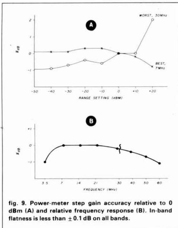
tenuators to attenuate the reference signal and comparing this known level to the power-meter reading. Fig. 9 shows the flatness and step accuracy that I achieved with my power meter.
