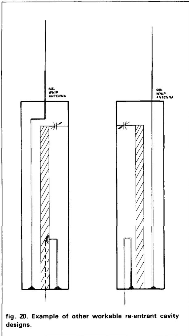
this antenna has a small insertion loss at resonance, which is about the same as the loss in the usual resonator that it replaces. However, there are bandwidth limitations under certain conditions which will be discussed later.
