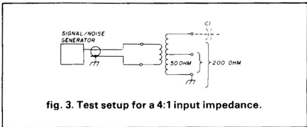
fig. 3. Test setup for a 4:1 input impedance.
