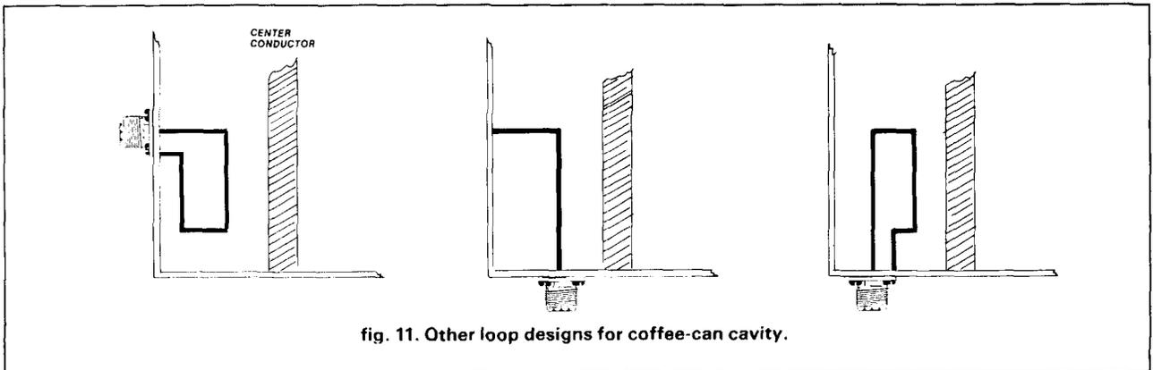
as shown. Other loop configurations that can be used are shown in fig. 11.
