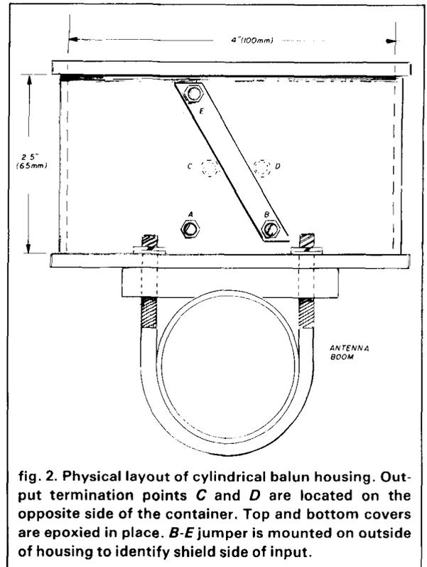
resonant transformer. A functional and inexpensive container may be fashioned from a 4-inch (100 mm) PVC pipe coupling cut down to 2-1/2 inches (65 mm) long. Alternatively, a short length of acrylic tubing, or even some plastic freezer containers, may be used. In any case, be certain that the housing is watertight and that the top and bottom covers have no gaps, once cemented into place.
