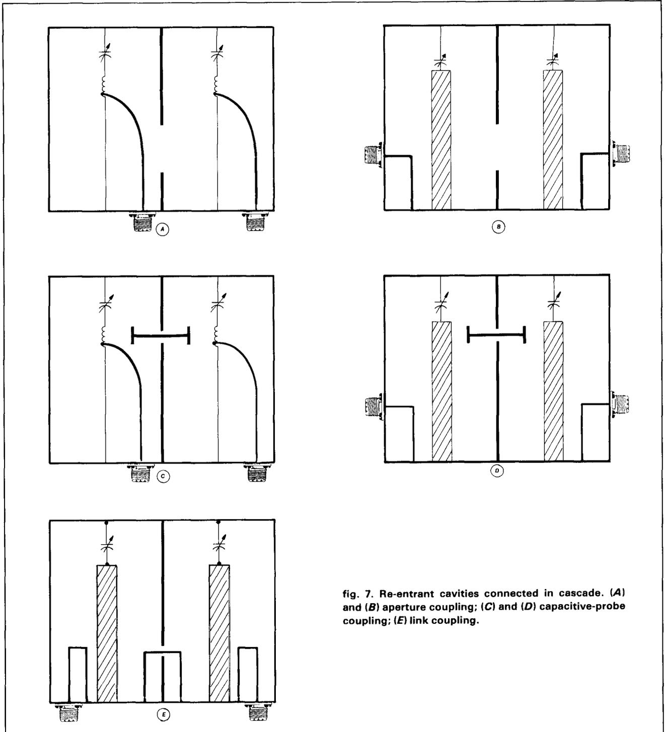
fig. 7. Re-entrant cavities connected in cascade. (A) and (B) aperture coupling; (C) and (D) capacitive-probe coupling; (E) link coupling.
