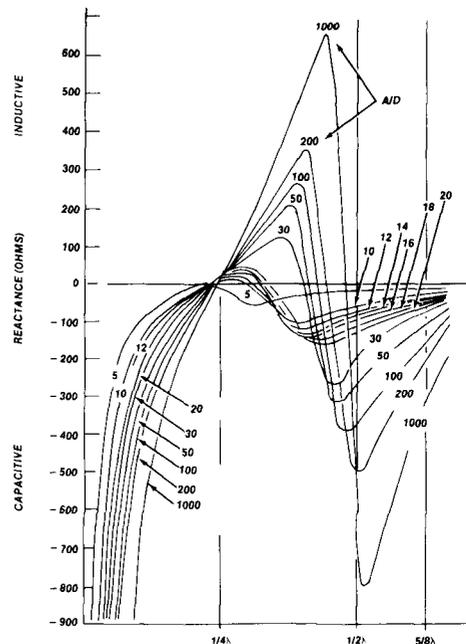
**fig. 16.** Terminal reactance as a function of antenna length. A/D is the length/diameter ratio.<sup>10</sup>
