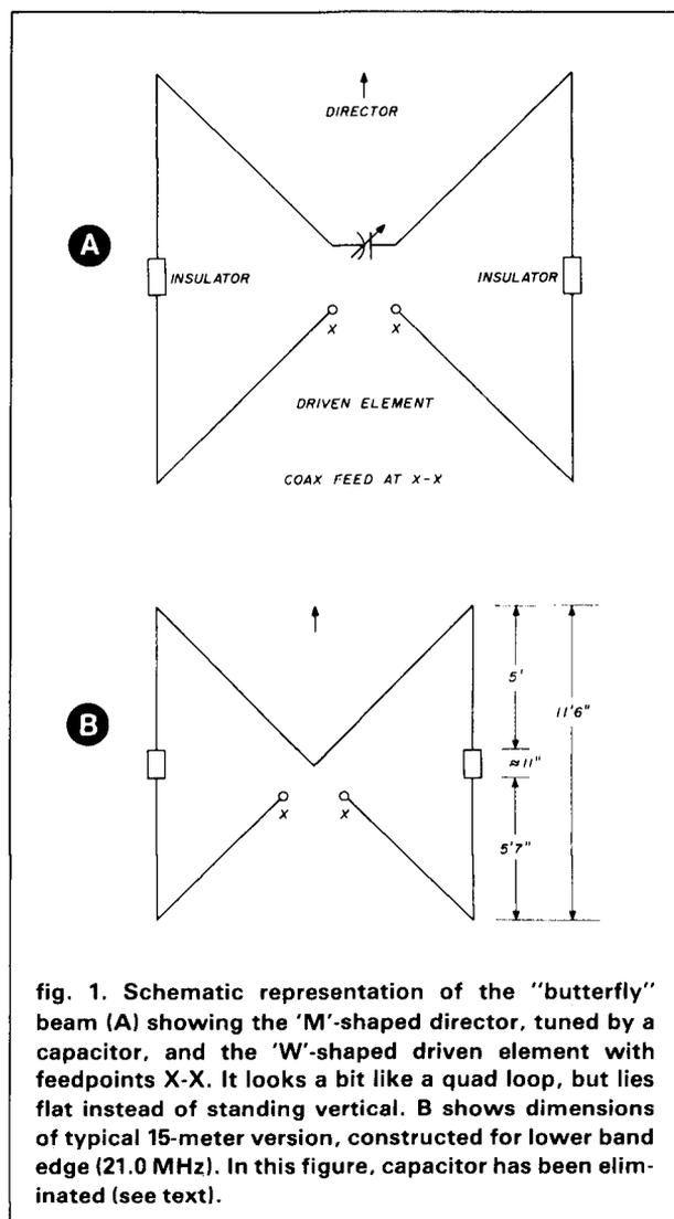
fig. 1. Schematic representation of the "butterfly" beam (A) showing the 'M'-shaped director, tuned by a capacitor, and the 'W'-shaped driven element with feedpoints X-X. It looks a bit like a quad loop, but lies flat instead of standing vertical. B shows dimensions of typical 15-meter version, constructed for lower band edge (21.0 MHz). In this figure, capacitor has been eliminated (see text).
