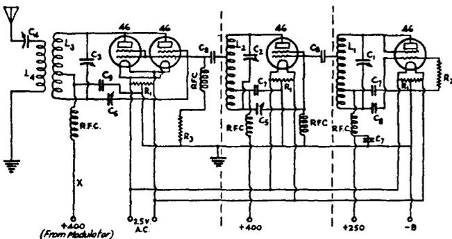
FIG. 1 — WIRING DIAGRAM OF THE RADIO-FREQUENCY END
