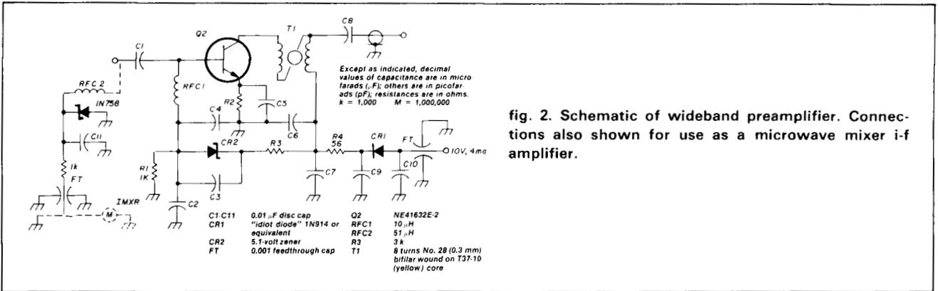
fig. 2. Schematic of wideband preamplifier. Connections also shown for use as a microwave mixer i-f amplifier.
