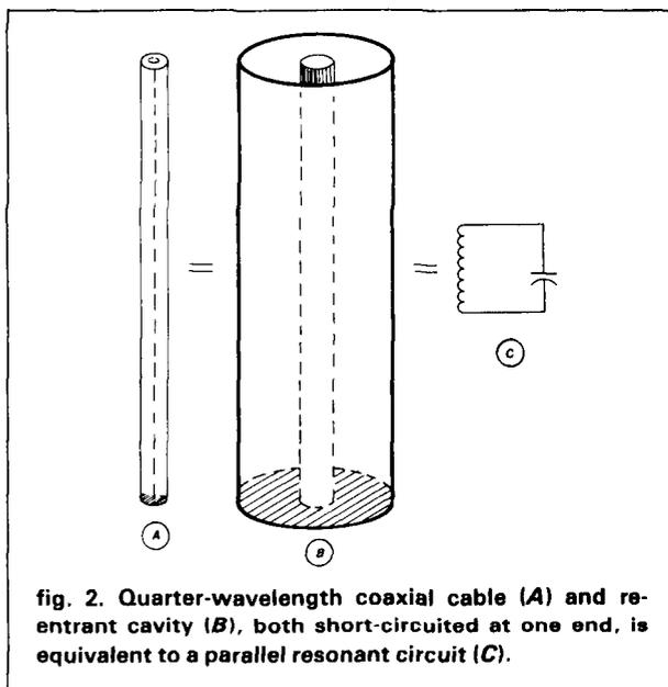
fig. 2. Quarter-wavelength coaxial cable (A) and re-entrant cavity (B), both short-circuited at one end, is equivalent to a parallel resonant circuit (C).
