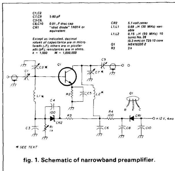
fig. 1. Schematic of narrowband preamplifier.
