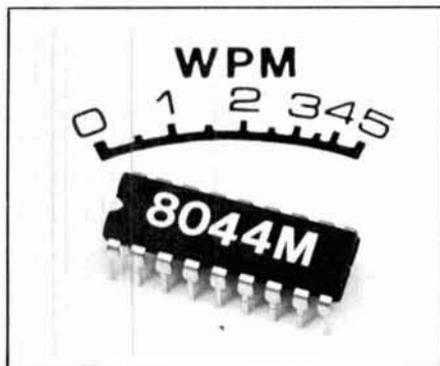
The addition of two extra pins at the end of the package permits a pin-for-pin fit with the standard 8044. One of the pins is used for a timing capacitor and the other pin drives the meter directly. This allows retrofitting in many existing keyers with relative ease. The keyer function of the 8044M remains the same as in the 8044 design, providing dot and dash memories, iambic operation, key debouncing, weight control, monitor oscillator, and extremely low power dissipation.
