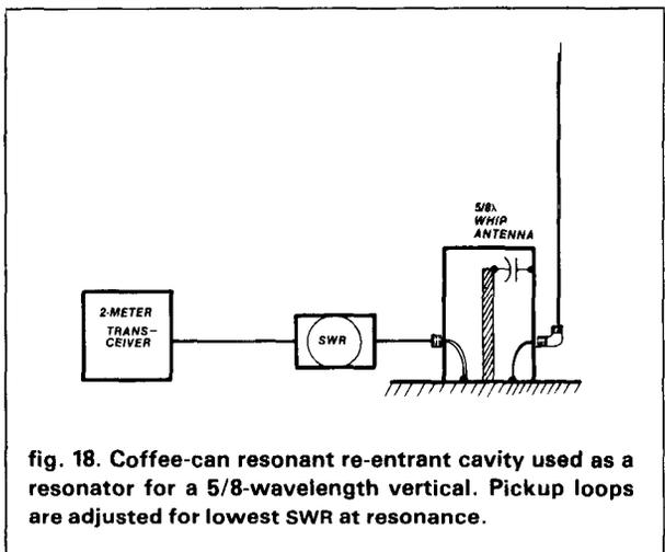
fig. 18. Coffee-can resonant re-entrant cavity used as a resonator for a 5/8-wavelength vertical. Pickup loops are adjusted for lowest SWR at resonance.
