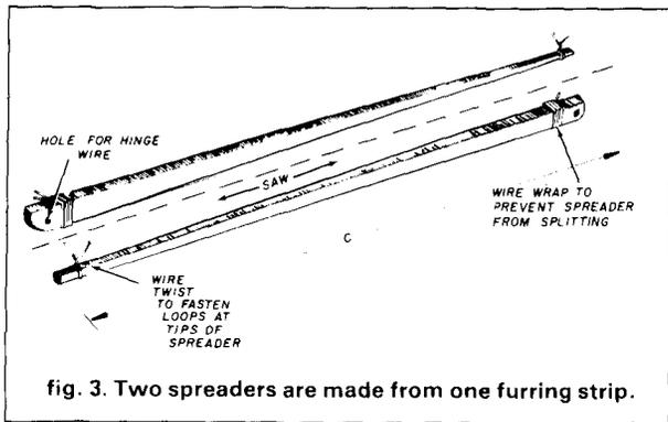
fig. 3. Two spreaders are made from one furring strip.
