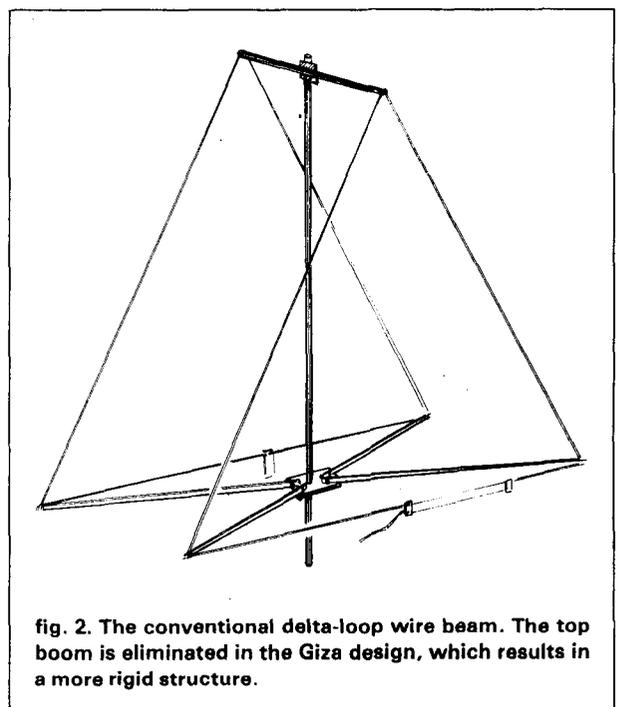
fig. 2. The conventional delta-loop wire beam. The top boom is eliminated in the Giza design, which results in a more rigid structure.
