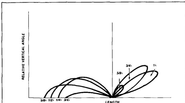
**fig. 14.** Vertical-angle patterns of various lengths of vertical radiators. Five-eighths wavelength, three-quarter wavelength, and full wavelength high-angle lobes are shown on right for clarity. (Note absence of low-angle lobe for full-wavelength vertical.)
