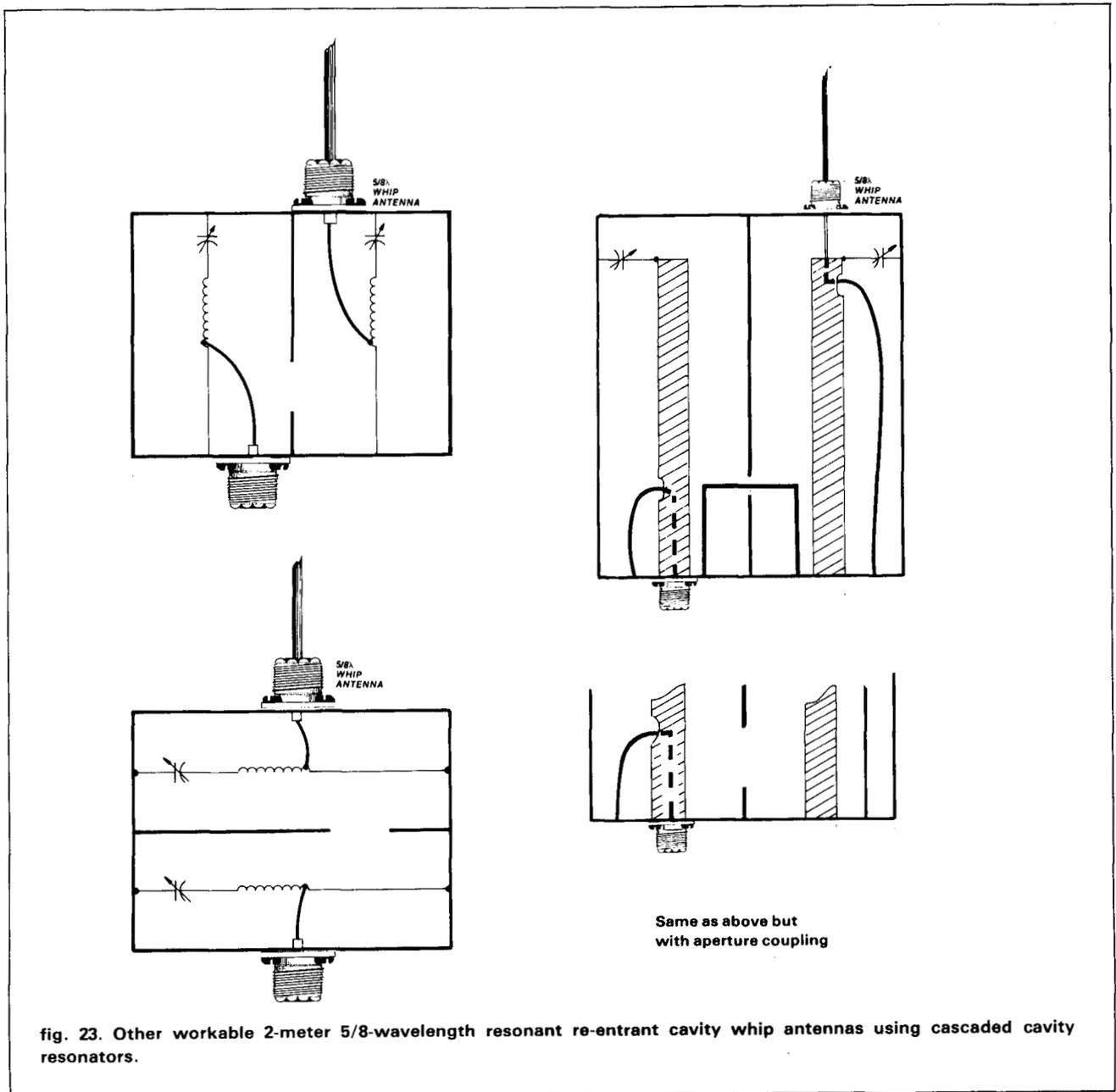
fig. 23. Other workable 2-meter 5/8-wavelength resonant re-entrant cavity whip antennas using cascaded cavity resonators.
