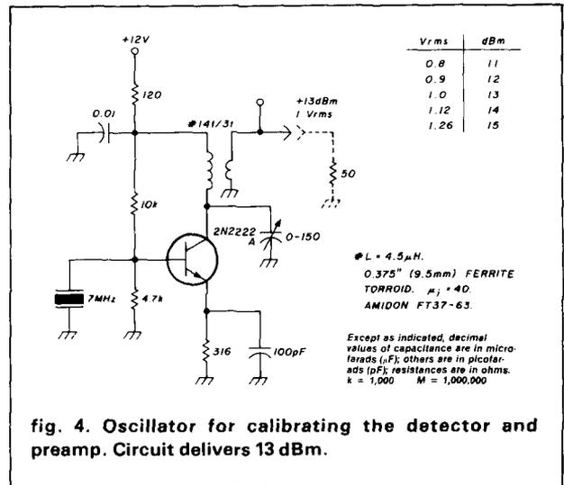
fig. 4. Oscillator for calibrating the detector and preamp. Circuit delivers 13 dBm.
