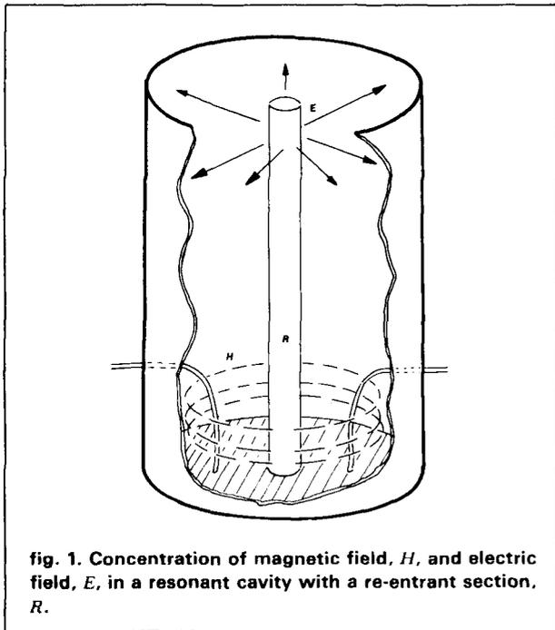
fig. 1. Concentration of magnetic field,  $H$ , and electric field,  $E$ , in a resonant cavity with a re-entrant section,  $R$ .
