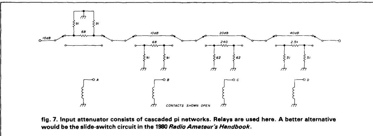
fig. 7. Input attenuator consists of cascaded pi networks. Relays are used here. A better alternative would be the slide-switch circuit in the 1980 *Radio Amateur's Handbook*.
