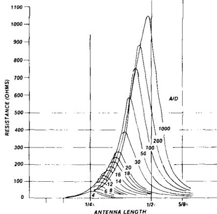
**fig. 15.** Terminal resistance as a function of antenna length. A/D is the ratio of antenna length to diameter.<sup>10</sup>
