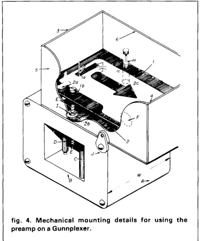
screw **E**; and a ground stud, **H**, almost directly behind screw **E**.
