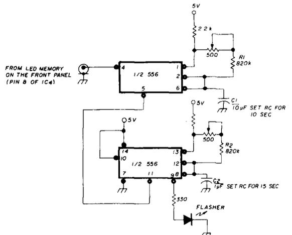
onds. The second, or flashing, section of the 556 was set up as an astable free-running oscillator, frequency modulated through pin 11 from pin 5 of the first monostable section. Timing in both cases was set by the miniature 500k pots.
