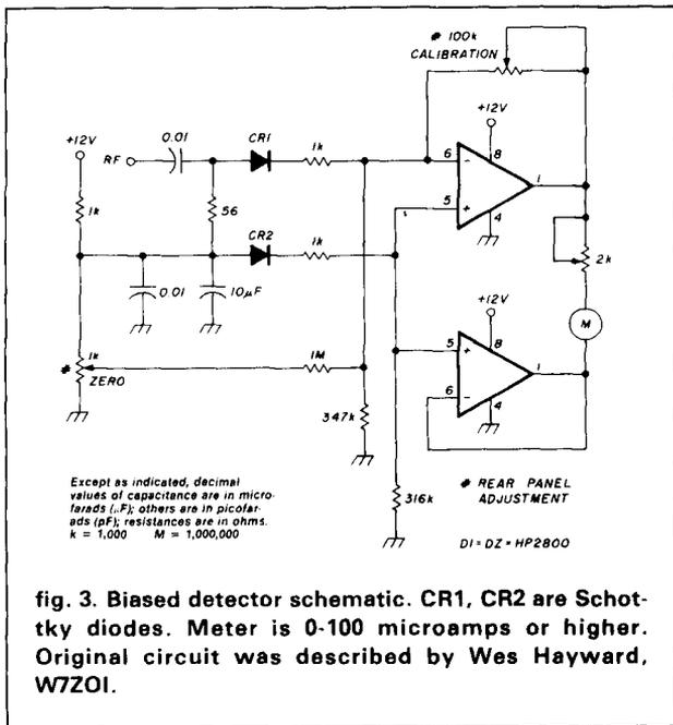
fig. 3. Biased detector schematic. CR1, CR2 are Schottky diodes. Meter is 0-100 microamps or higher. Original circuit was described by Wes Hayward, W7ZOI.
