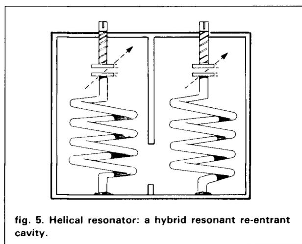
the quarter-wavelength cavity. In the half-wavelength version, the two short-circuited ends are high current areas, while the center is the point of high voltage, where a variable capacitor is used to tune the cavity to resonance. Note that a 3/4-wavelength cavity has characteristics similar to those of the more widely used 1/4-wavelength cavity.
