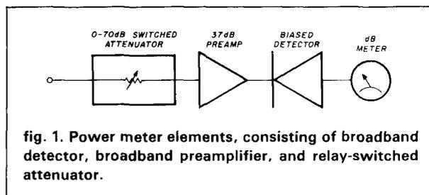
fig. 1. Power meter elements, consisting of broadband detector, broadband preamplifier, and relay-switched attenuator.
