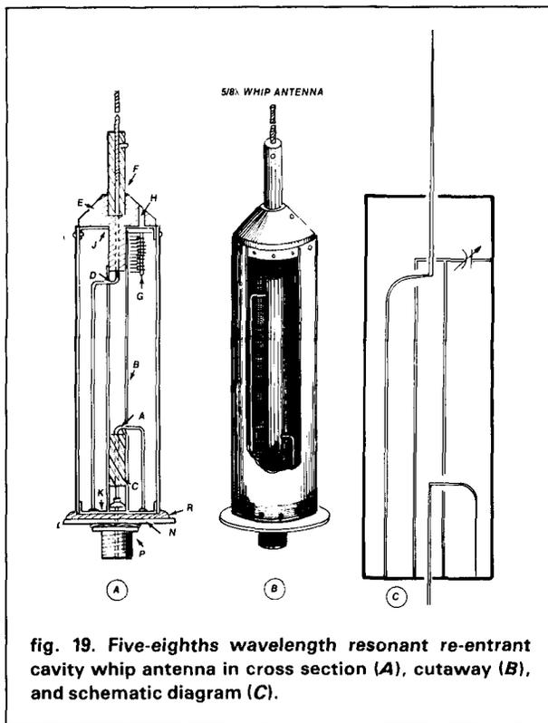
fig. 19. Five-eighths wavelength resonant re-entrant cavity whip antenna in cross section (A), cutaway (B), and schematic diagram (C).
