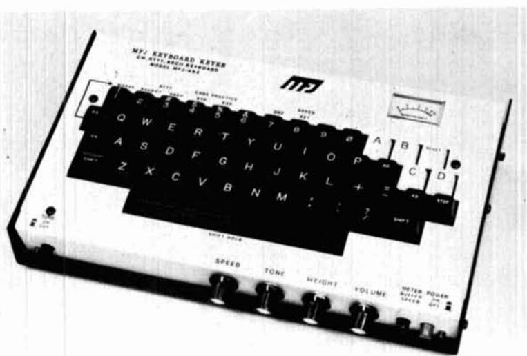
The 50-character text buffer can be filled prior to sending (pre-programmed), or it can be filled at any given speed if you type faster than the code is being sent. When the buffer approaches full, the side tone pitch changes and a red LED comes on to warn you to slow down typing to prevent buffer overflow.
