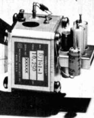
ARR is proud to offer the complete Microwave Associates Gunnplexer and accessory line. Two of the Gunnplexer transceivers shown here (the MA87141-1, at only \$239.95 per pair) can form the heart of a 10 GHz communications system for voice, cw, video or data transmission, not to mention mountaintop DXing! ARR sells a line of necessary support equipment such as power supply/modulator and receiver boards. Write or call for additional information.
