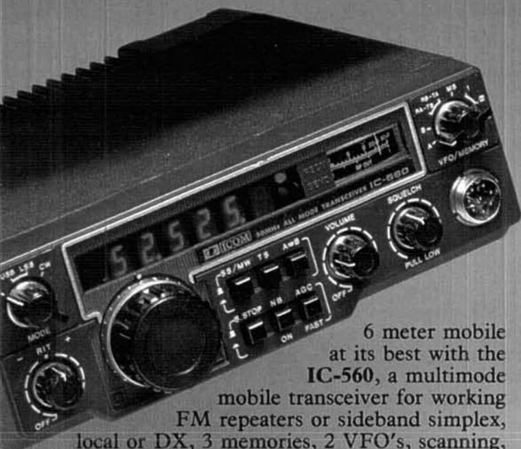
6 meter mobile at its best with the IC-560, a multimode mobile transceiver for working FM repeaters or sideband simplex, local or DX, 3 memories, 2 VFO's, scanning, squelch on SSB.
