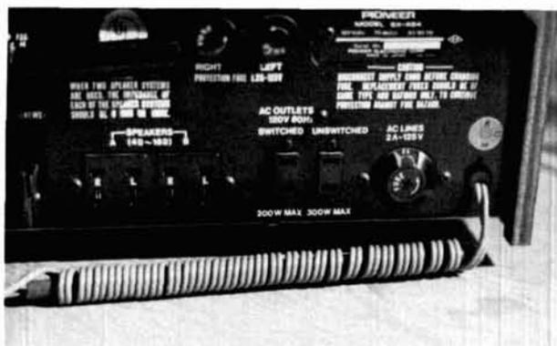
If the interference is entering the stereo through the ac line, the cord can be wrapped around a ferrite rod to form a bifilar choke.
