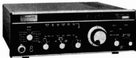
Features include excellent sensitivity and selectivity, high dynamic range, digital frequency readout, and full break-in CW operation. AGC time constants are selectable and RIT is front panel selectable. Most Drake 7-line accessories are compatible. Nominal power input is 150 watts. Price is \$1099.
