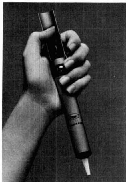
vacuum that instantly removes molten solder. Double O-ring piston-seals achieve maximum vacuum in a piston stroke of less than two inches. The piston is set with the thumb and released by pushbutton for maximum spring force. The worker's other hand is left free to hold the soldering iron that melts the solder.
