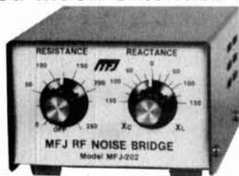
This MFJ-202 RF Noise Bridge lets you quickly adjust your single or multiband dipole, inverted Vee, beam, vertical, mobile whip or random system for maximum performance.
