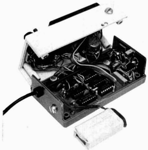
The auto-dialer in this plastic case uses an earlier version PC board that is a hair narrower than the board shown in **fig. 3**. The battery fits right on top of the ICs. Note the 1-inch speaker in the upper right corner of the cover.
