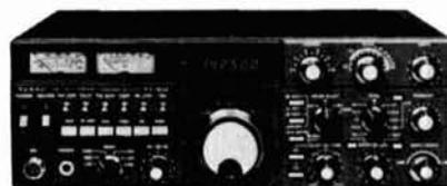
The FT-102 receiver uses JFET components in the front end for wide dynamic range. A number of filter options are available, with wide/narrow filter selection independent of the mode switch. Audio peak filtering for CW, audio shaping for all modes, and an i-f notch filter provide intelligence recovery. The noise blanker is highly effective against the Woodpecker and pulse noises.
