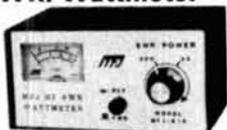
New MFJ-816 low cost HF SWR/Wattmeter for 1.8 to 30 MHz range. Toroidal current pickup gives uniform sensitivity over entire HF frequency. Read SWR, forward and reflected power in 2 ranges (30 and 300 watts) on two color scale. SO-239 coax connectors. 4-1/2x2-3/8x2-7/8 in.
