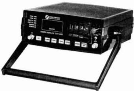
In addition to EIA CTCSS tones, the test unit works with digital codes compatible with Digital Private Line, Digital Channel Guard, Digital Quiet Channel, Digital Call Guard, etc. Used in conjunction with a monitor receiver, the test unit may be used to police shared repeaters, select unused
