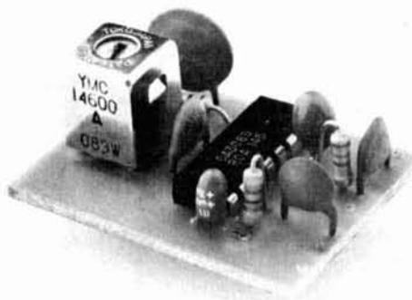
fig. 5. The fm demodulator board.
