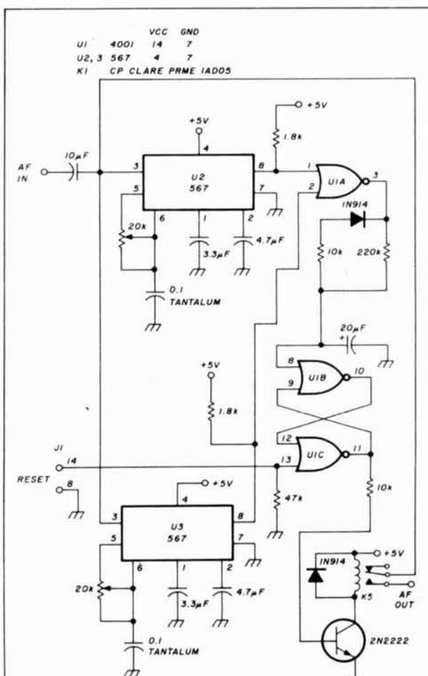
fig. 8. Optional fm audio-decoder schematic diagram. Any pair of tones can be selected. The tones must be held on for about eight seconds before relay K1 pulls in. This permits the system to be operated by an fm radio or telephone link.
