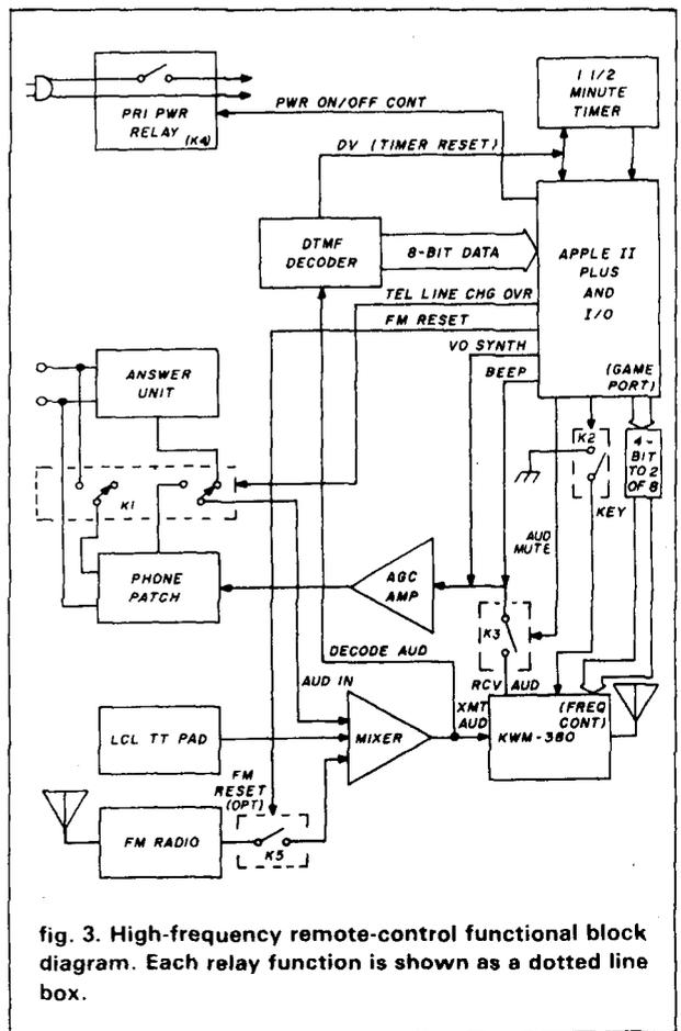
fig. 3. High-frequency remote-control functional block diagram. Each relay function is shown as a dotted line box.
