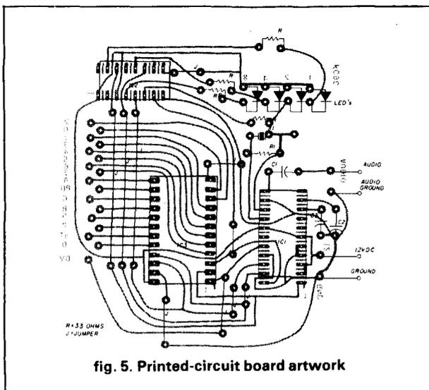
fig. 5. Printed-circuit board artwork
