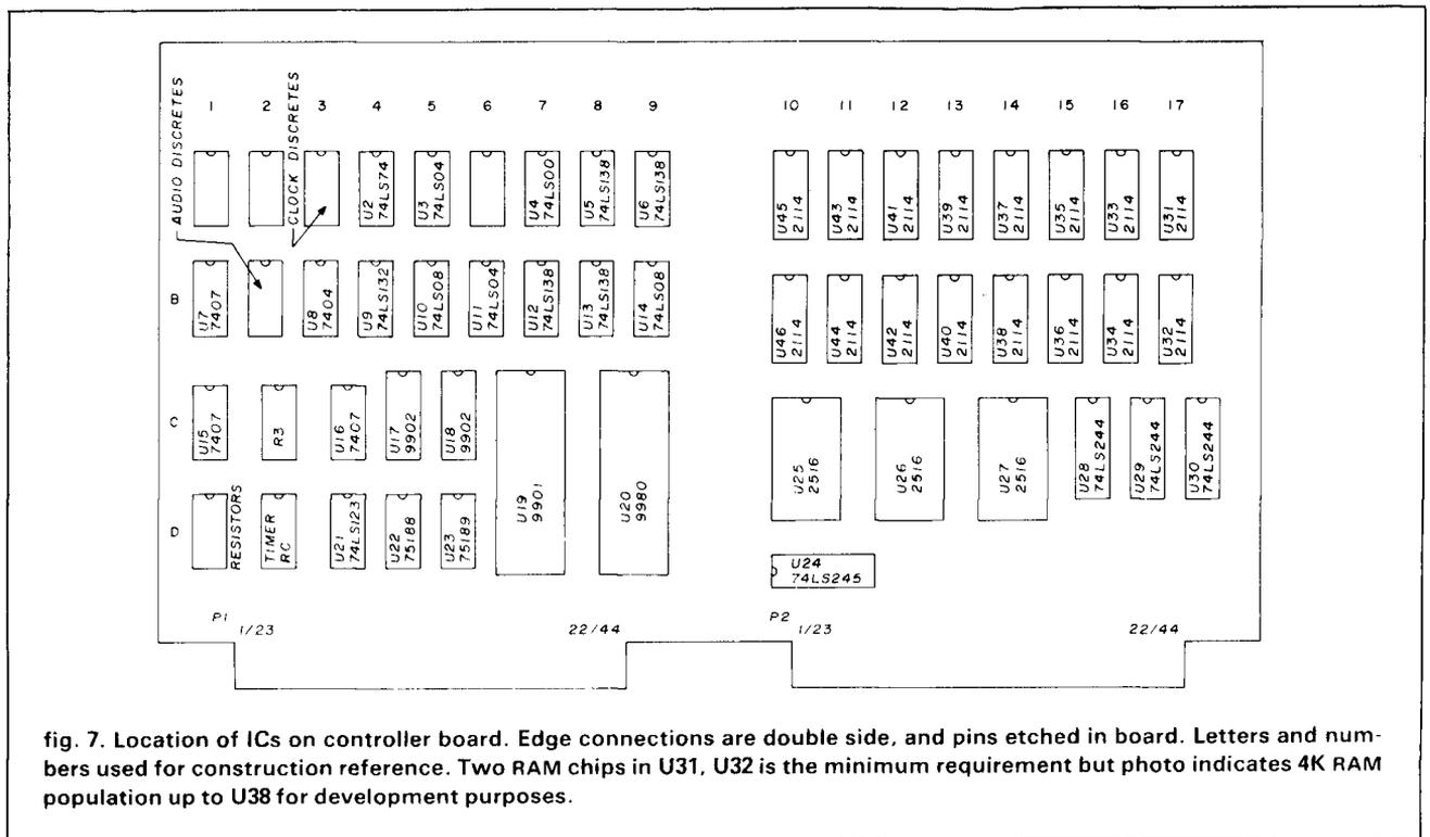
fig. 7. Location of ICs on controller board. Edge connections are double side, and pins etched in board. Letters and numbers used for construction reference. Two RAM chips in U31, U32 is the minimum requirement but photo indicates 4K RAM population up to U38 for development purposes.
