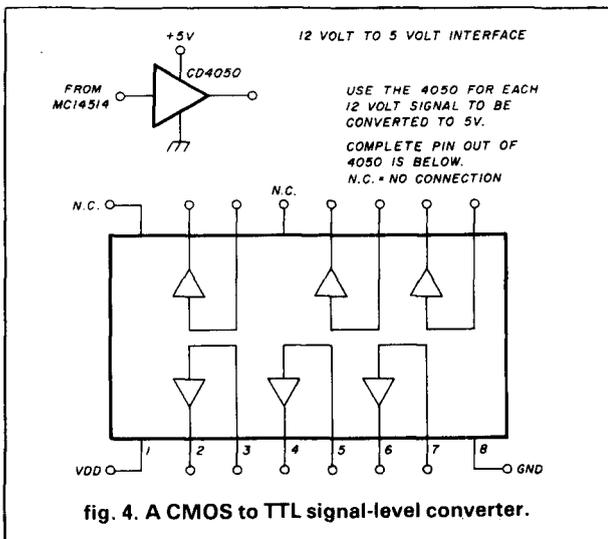
fig. 4. A CMOS to TTL signal-level converter.
