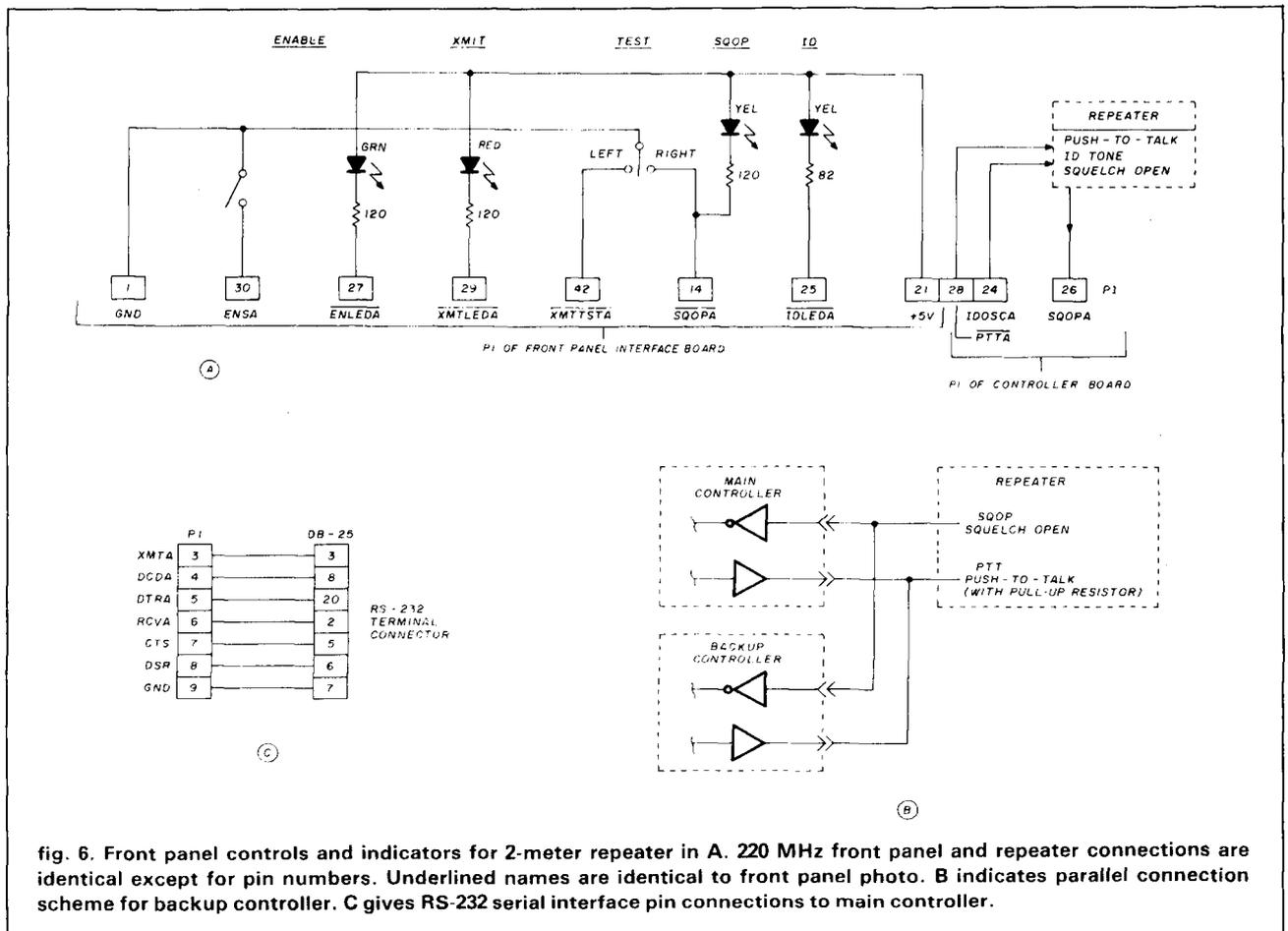
fig. 6. Front panel controls and indicators for 2-meter repeater in A. 220 MHz front panel and repeater connections are identical except for pin numbers. Underlined names are identical to front panel photo. B indicates parallel connection scheme for backup controller. C gives RS-232 serial interface pin connections to main controller.
