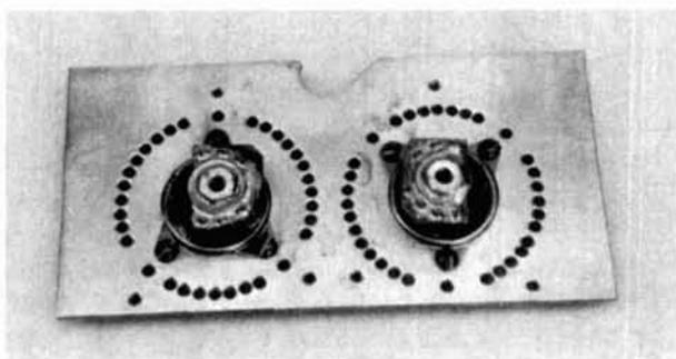
Triode amplifier socket plate assembly — bottom view.
