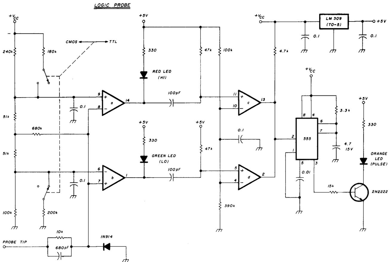
fig. 5. The improved logic probe.
