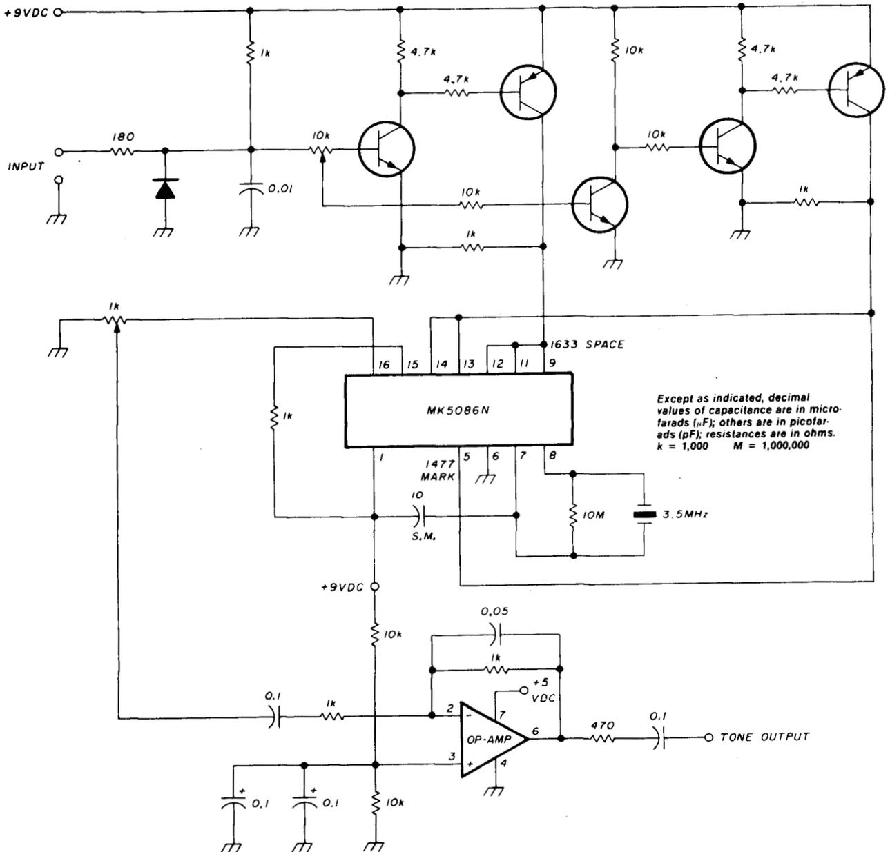
fig. 1. Schematic for the FSK tone generator.
