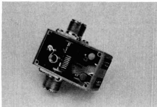
Output harmonic trap assembly. Three series traps — 100 MHz, 150 MHz, and 200 MHz. Piston capacitor adjustment screws (3) protrude out the bottom of the box.
