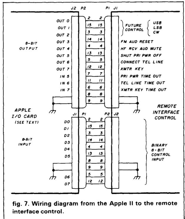
fig. 7. Wiring diagram from the Apple II to the remote interface control.
