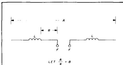
fig. 2. Loaded dipole with loading coils placed one-half the distance from the feedpoint (F-F) to the end. Distance A is one-quarter wavelength.
