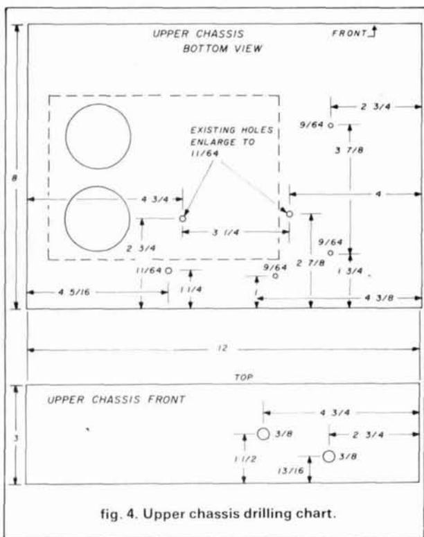
fig. 4. Upper chassis drilling chart.
