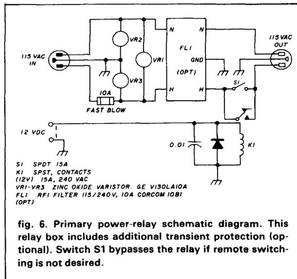
fig. 6. Primary power-relay schematic diagram. This relay box includes additional transient protection (optional). Switch S1 bypasses the relay if remote switching is not desired.
