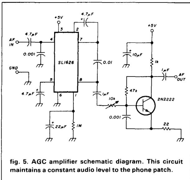
fig. 5. AGC amplifier schematic diagram. This circuit maintains a constant audio level to the phone patch.
