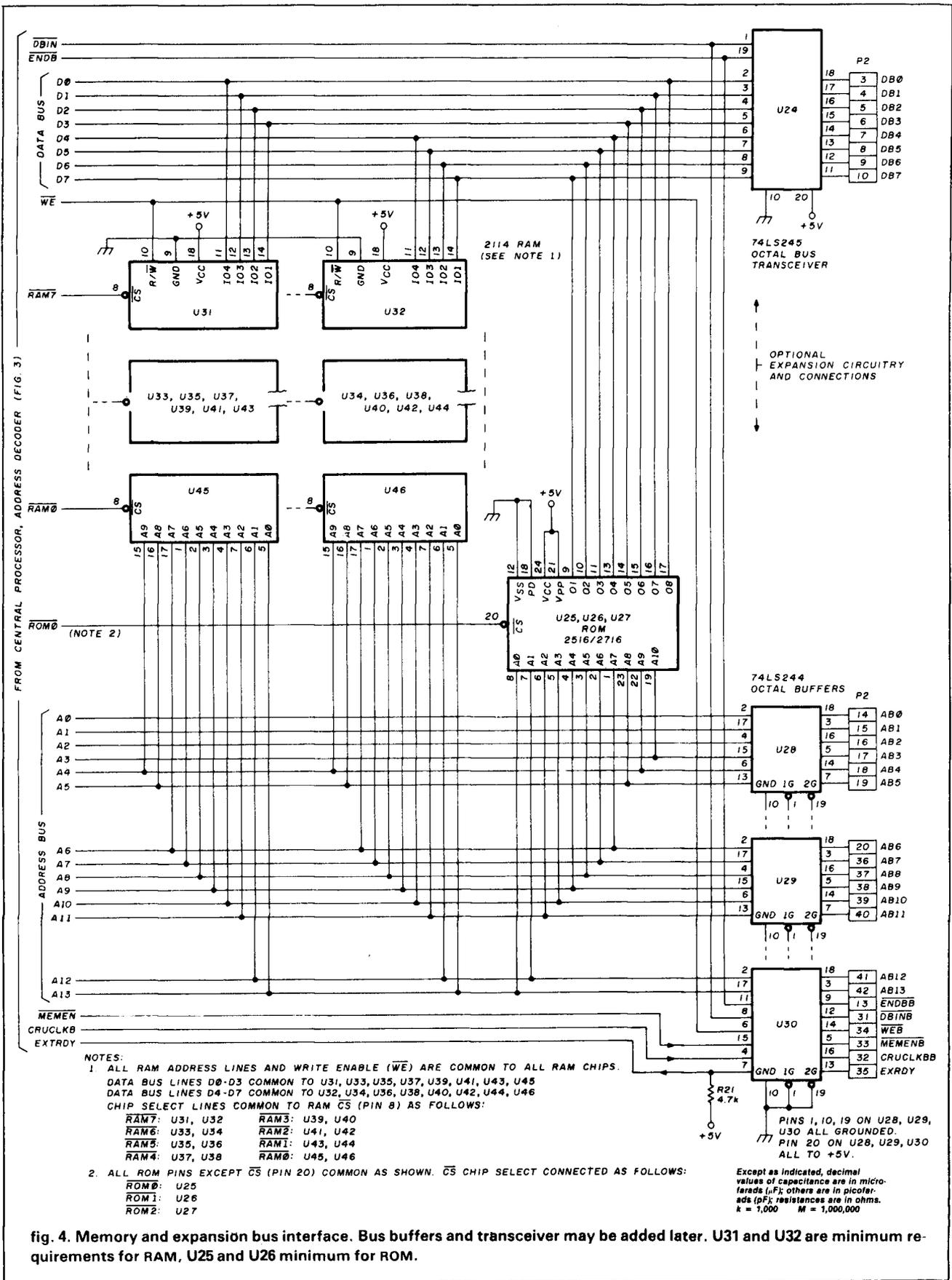
fig. 4. Memory and expansion bus interface. Bus buffers and transceiver may be added later. U31 and U32 are minimum requirements for RAM, U25 and U26 minimum for ROM.
