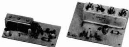
Our lab has developed a new line of low-noise receiver preamps with helical resonator filters built in. The combination of a low noise amplifier similar to the LNA series and the sharp selectivity of a 3 or 4 section helical resonator provides increased sensitivity while reducing intermod and cross-band interference in critical applications. See selectivity curves at right. Noise figure = 1 to 1.2 dB. Gain = 12 to 15 dB.
