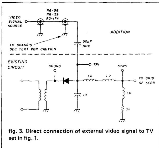
fig. 3. Direct connection of external video signal to TV set in fig. 1.
