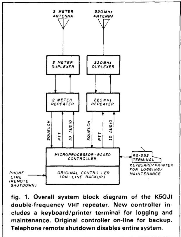
fig. 1. Overall system block diagram of the K5QJ1 double-frequency VHF repeater. New controller includes a keyboard/printer terminal for logging and maintenance. Original controller on-line for backup. Telephone remote shutdown disables entire system.
