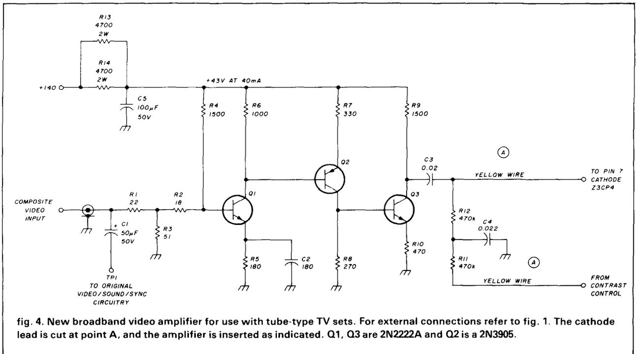
fig. 4. New broadband video amplifier for use with tube-type TV sets. For external connections refer to fig. 1. The cathode lead is cut at point A, and the amplifier is inserted as indicated. Q1, Q3 are 2N2222A and Q2 is a 2N3905.
