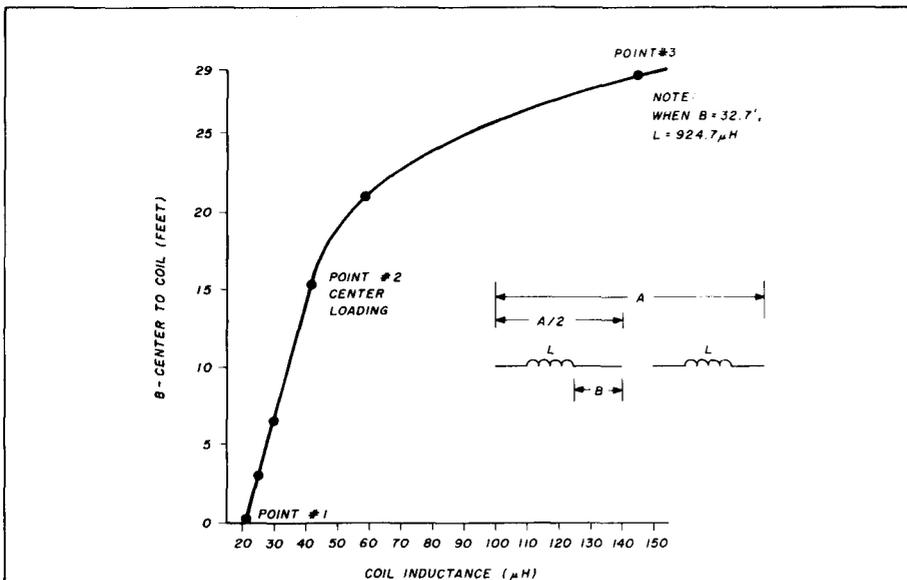
fig. 3. Inductance increases as the coil moves outward from the center of the loaded element. The increase in inductance is linear until coil reaches the center point of the element, and then it increases rapidly approaching the tip. If the coil is placed at the tip, inductance would theoretically have to be infinite. Coil loss increases with inductance, and point 2 on curve represents a practical compromise. Point 1 is for base loading.
