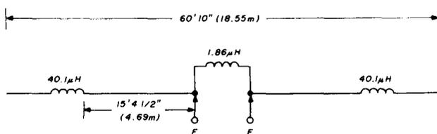
fig. 7. Compact, coil-loaded dipole for 3.80 MHz. Tip length is adjusted for minimum SWR at design frequency. Coil is wound with No. 16 (M1.3) wire per data in fig. 5.
