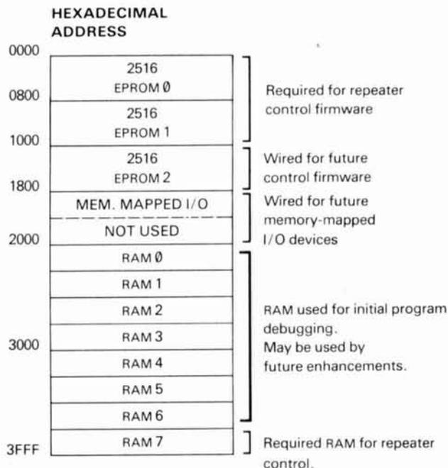
fig. 4A. Memory map of controller. Monitor ROM located in \$0000 to \$07FF address. Minimum RAM in address location \$3D00 to \$3FFF (\$ = hexadecimal).
