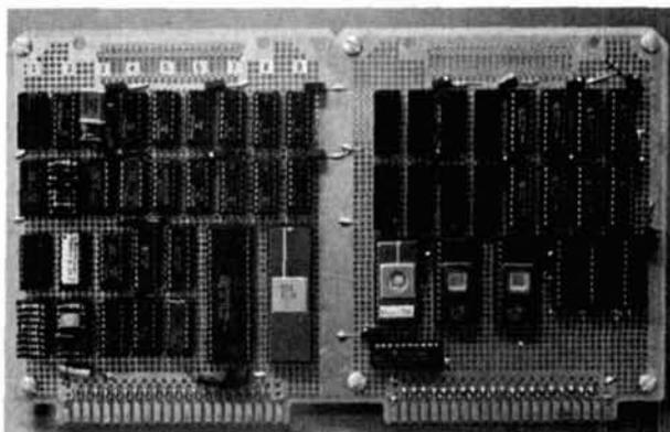
**photo 2.** Photo of controller board made just before final circuit freeze. All ICs are socketed on prototype board. Except for supply bypass capacitors, all discrete components mounted on DIP plugs. Number labels were construction references.
