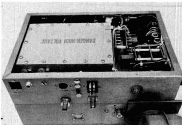
Triode amplifier bottom view to illustrate mounting of optional circuit features on terminal boards in lower chassis.
