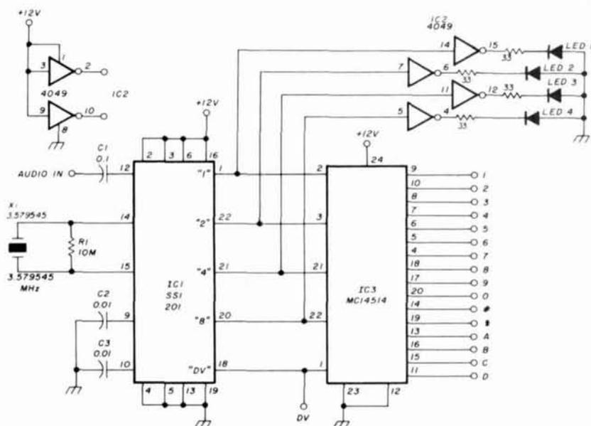
fig. 3. Schematic diagram of the author's completed decoder circuit. The CMOS signals are all 12-volt levels, so a converter is needed if the decoder must drive TTL.
