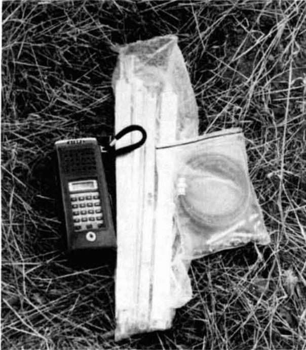
The station, ready to be assembled. The longer antenna parts are in a plastic bag. The smaller pieces and a length of coaxial cable are in the smaller pouch. (Photo courtesy N6ST.)
