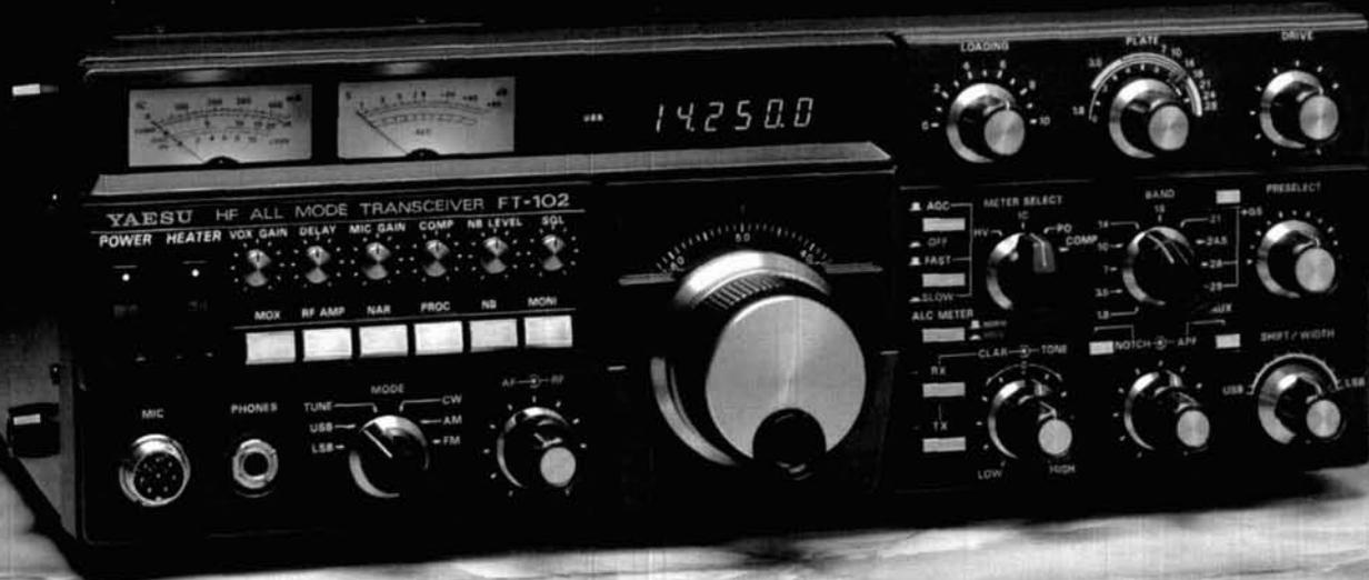
The FT-102 is factory equipped for operation on all present and proposed Amateur HF bands. An extra AUX band position is available for special applications. Equipped for SSB, CW, and AM (RX), the FT-102 may be activated on FM and AM (TX) via the optional AM/FM-102 Module.
