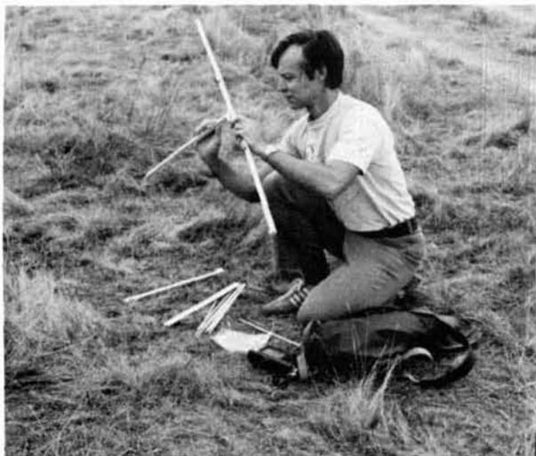
The boom is assembled and the first part of the mast is added. (Photo courtesy N6ST.)
