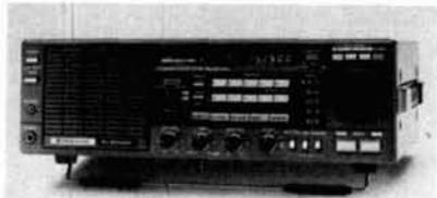
fm. Among the more interesting features to be found on this model are digital VFOs, ten memories that store frequency, band, and mode data, memory scan, programmable band scan, and dual 24-hour quartz clocks with a timer that can be programmed to turn the radio on and off on a pre-selected schedule.
